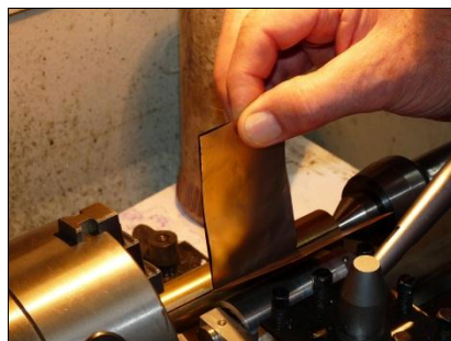
FIG. 2. Preliminary profiling of liner after profiling foils.
