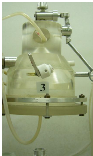
FIG.9. Equipment for filtration, drying and filling of dried gel granules.
