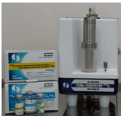
FIG. 15. ^{99m}\text{Tc} gel-generator with set of evacuated and saline vials.
