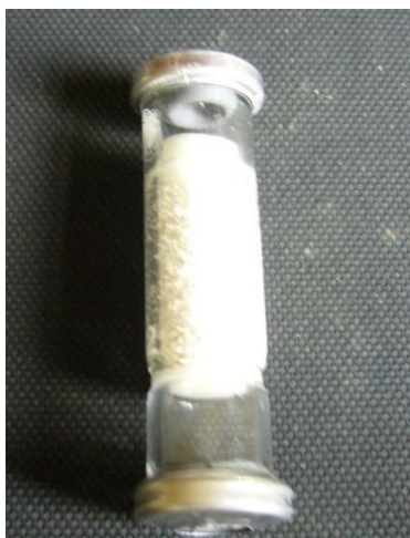
FIG.12. Column of ^{99\text{m}}\text{Tc} gel-generator with ^{99}\text{Mo} -Zr gel.
