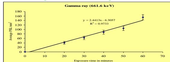
Average PSL readout from NIP VS exposure time
