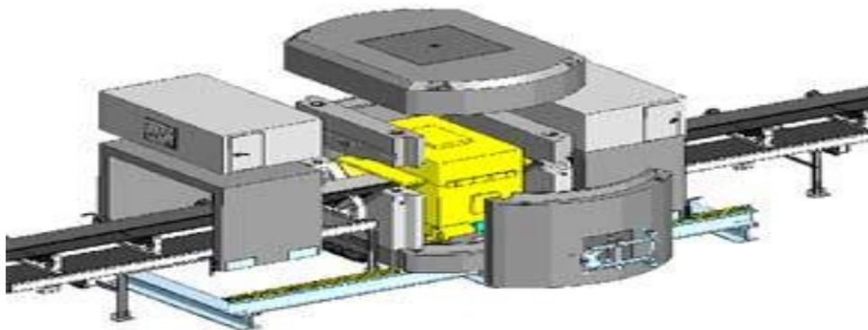
*Fig. 4. Layout of PGNAA on-line analytical facility for coal analysis.*
