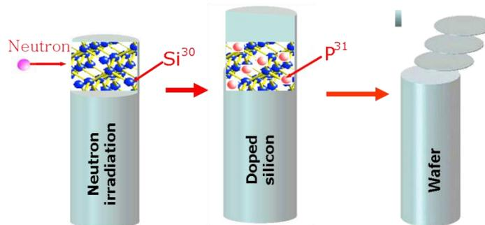
Fig. 4. Neutron transmutation doping reaction by neutron.
