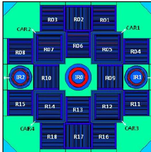
*Fig. 1. JRTR Core showing the fuel assemblies and beryllium blocks.*
