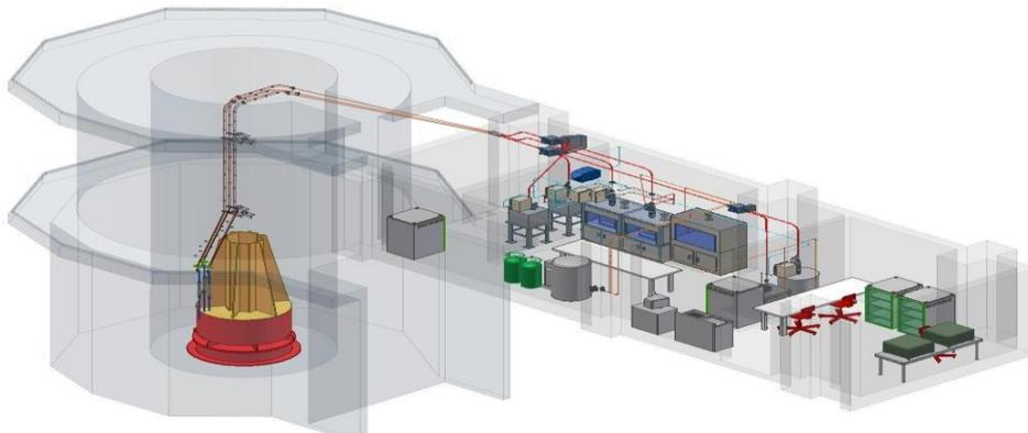
*Fig. 3. Neutron activation analysis facility.*
