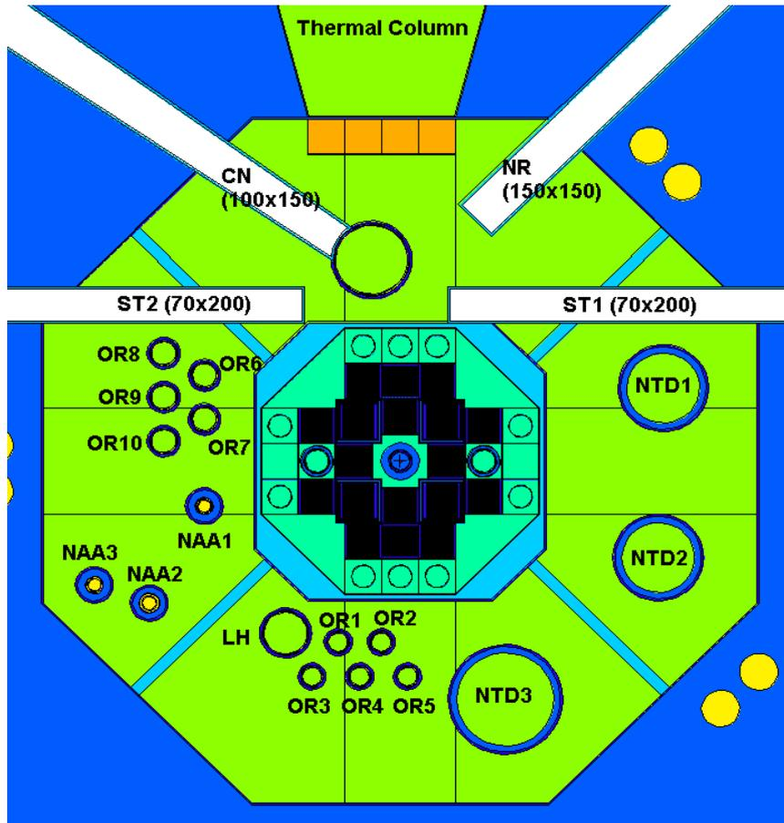
*Fig. 2. JRTR utilization facilities layout.*
