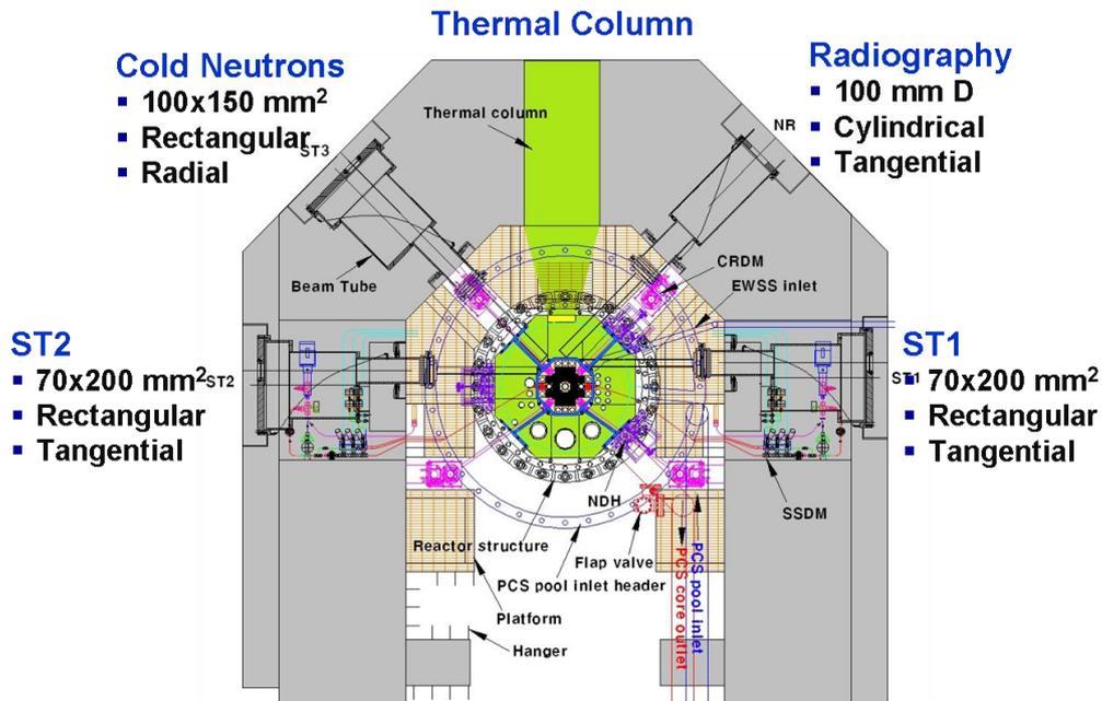
Fig. 5. JRTR neutron beam ports.
