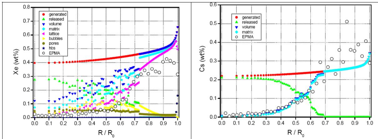
Fig. 6. Prediction of fission product behaviour in irradiated MOX fuel and comparison with microprobe analysis; note that released Xe is not detectable by EPMA due to the sample preparation method.
