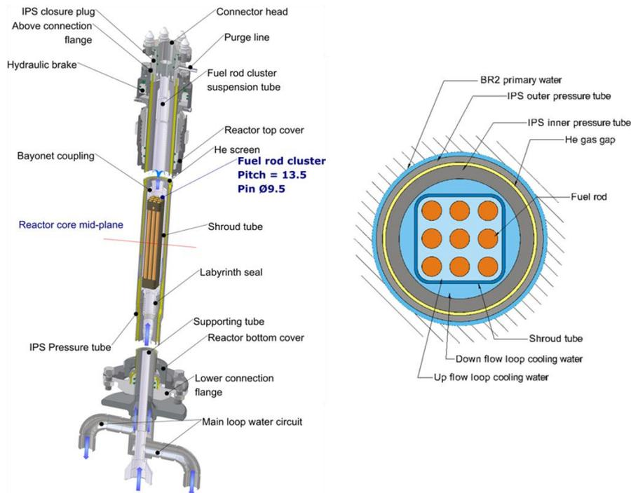
Fig. 4. Layout of the in-pile section of the CALLISTO loop.
