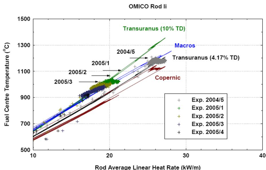
Fig. 7. Code predictions versus measured internal temperatures in the OMICO experiment in the CALLISTO loop.
