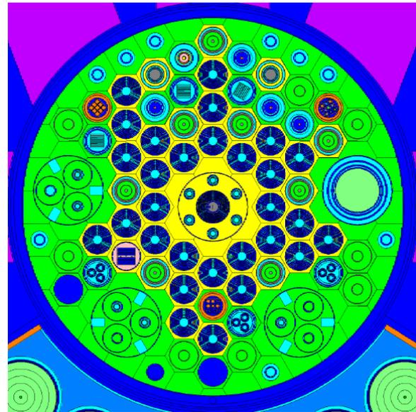
Fig. 2. current reactor core configuration.
