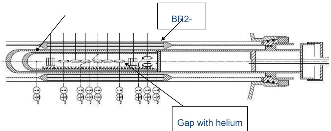
*Fig. 8. Schematic of the LBE capsule for irradiation of materials in ADS relevant conditions inside a BR2 fuel element.*
