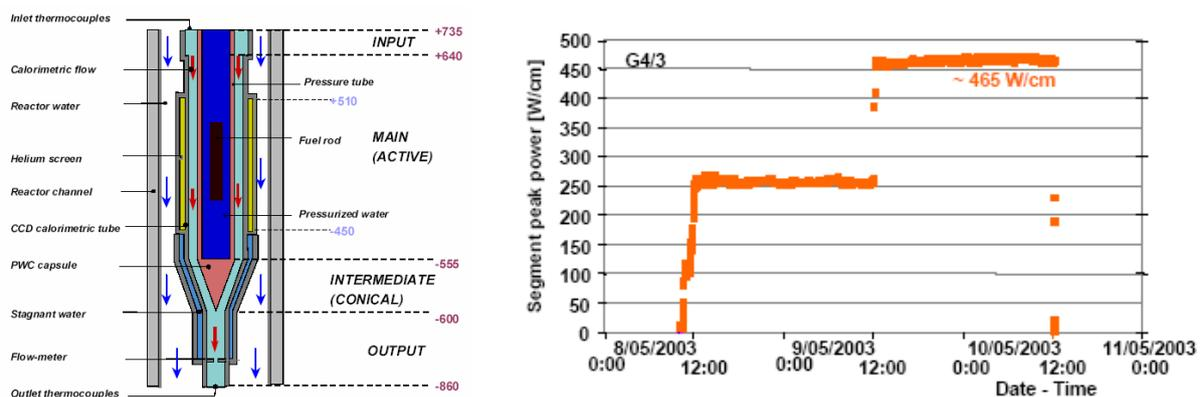
Fig. 5a (left): lay out of the PWC-CCD device for fuel pin testing; figure 5b (right): power profile during a transient test of a fuel pin in the PWC-CCD device.
