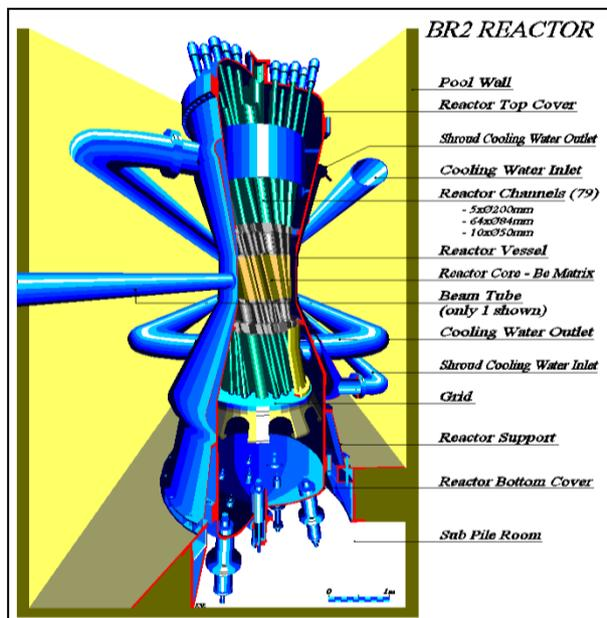
Fig. 1. general lay out of the BR2 reactor.
