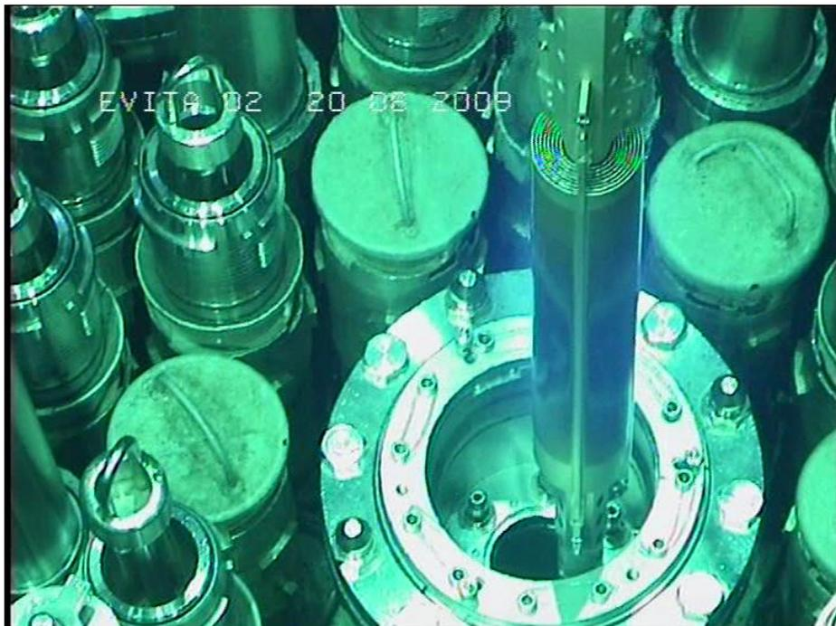
*Fig. 9. Unloading of the prototype RJH fuel element from the test loop after irradiation in the BR2 reactor.*
