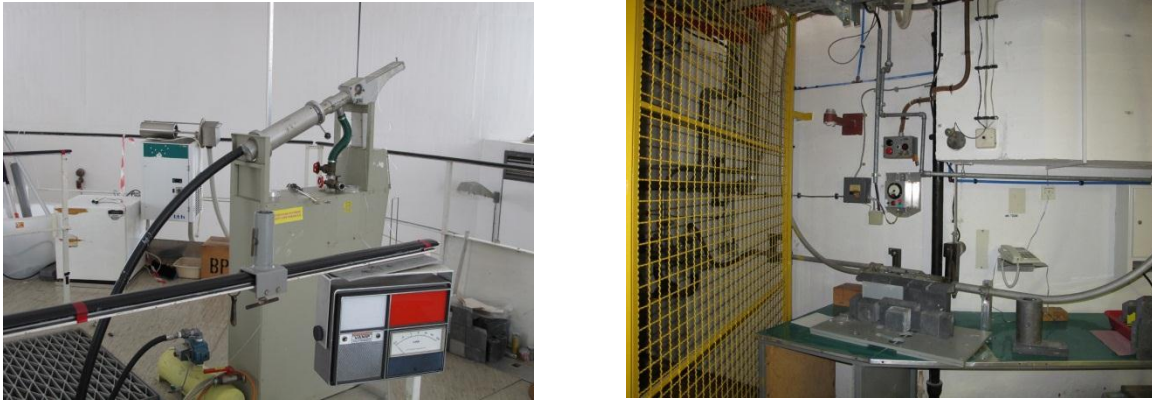
Fig. 1. Pneumatic systems for long (left) and short (right) irradiations.
