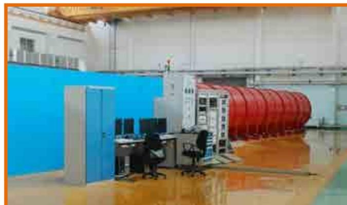
FIG. 9. Small Angle Neutron Spectrometer.
