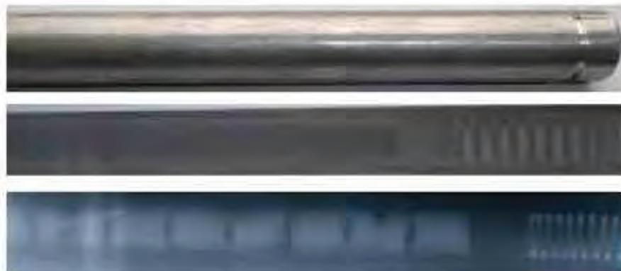
*FIG. 18. The photo (upper), X ray image (middle) and neutron image (lower) of simulated Nuclear fuel elements.*
