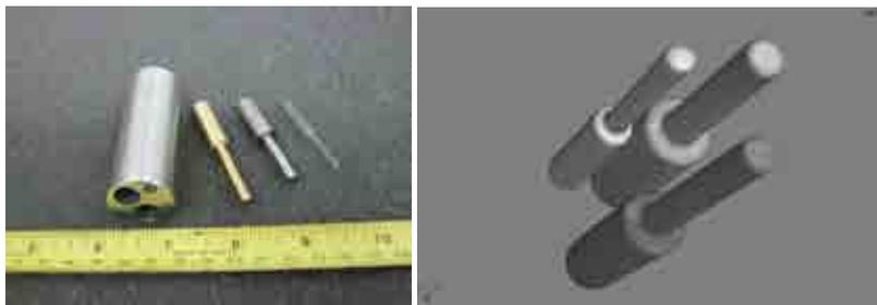
FIG. 7. (left) Aluminium case and insets (brass, steel and Perspex); (right) 3D image of the insets.
