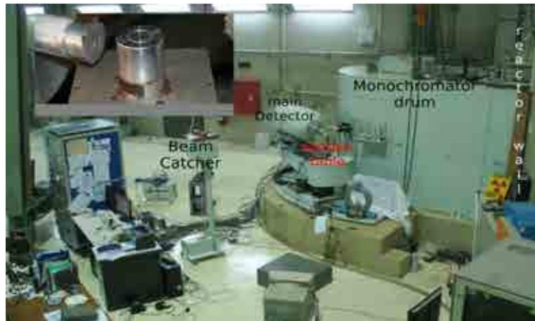
FIG. 12. Neutron diffractometer for residual stress measurement DN1 installed at the beam tube S6 of the RSG-GAS reactor. Inset: position of VAMAS shrink-fit sample for radial direction measurement.
