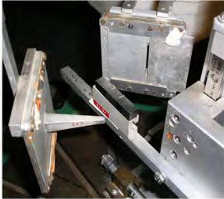
*FIG. 6. Photo of the specimen with the weld on one side as installed on the neutron beam defined by slits.*
