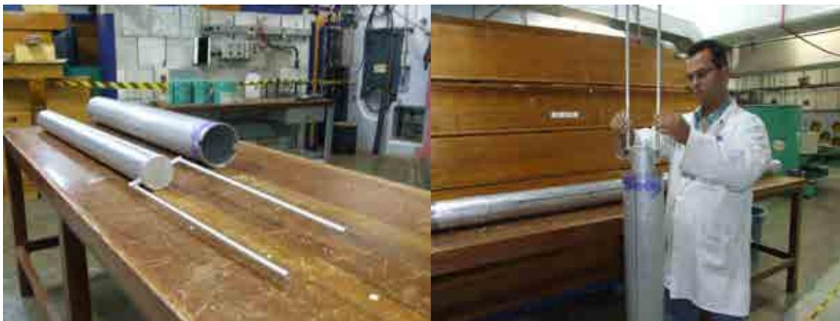
*FIG. 12. (left) Parts of the new collimator; (right) mounting of the collimator.*
