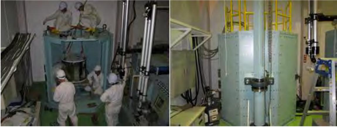
FIG. 6. Superconducting 15.5 Tesla magnet installed in the hot cell of the Oarai Branch of the IMR.
