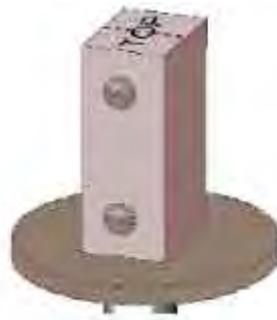
FIG. 11. Resolution sample (PSI): Type A(Al+ Cu), Type B(Fe+ Al).
