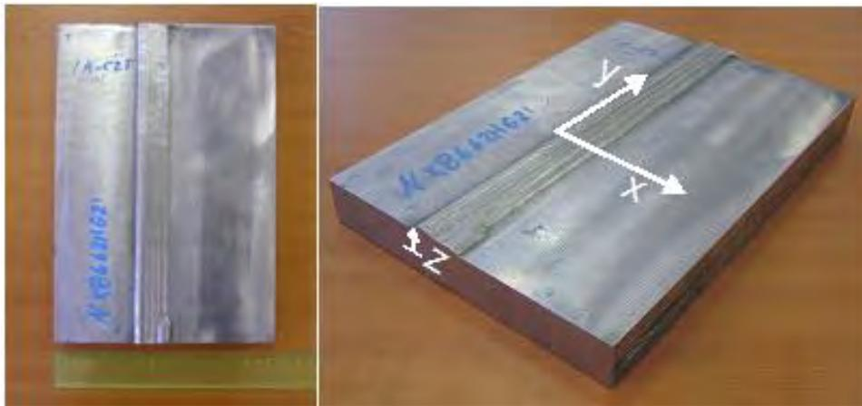
FIG. 1. Photograph of the 2HG21 welded plate and chosen system of coordinates (compatible with Fig. 2).
