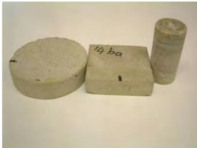
FIG. 4. Examples of the concrete, mortar and cement paste samples saturated with liquid.
