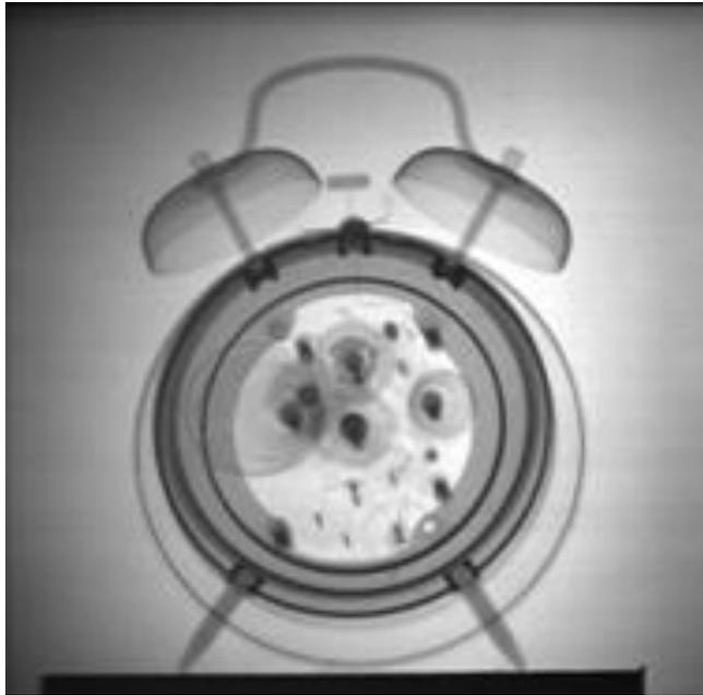
*FIG. 1. First image from DINGO neutron radiography instrument.*
