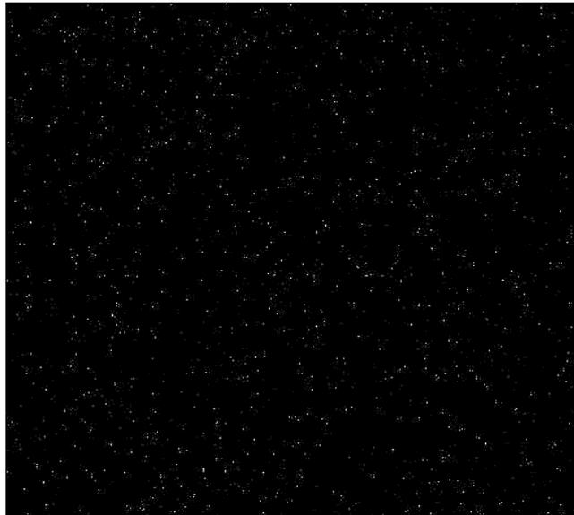
*FIG. 10. Damages caused by radiation in the CCD sensor.*
