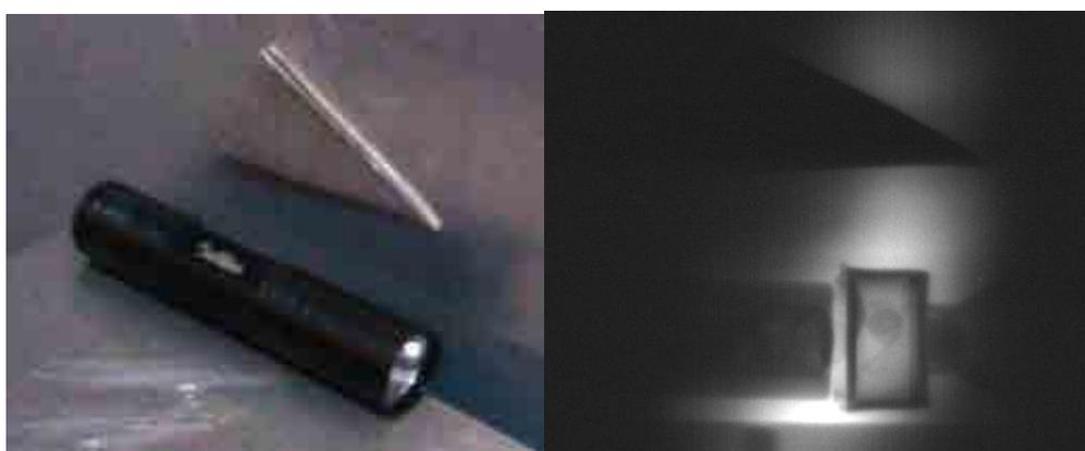
FIG. 20. Real-time Neutron image of flashlight. The neutron flux is about  $10^6 \text{ n}\cdot\text{cm}^{-2}\cdot\text{s}^{-1}$ . Resolution from MTF method is 0.5 mm. Pixel size is 0.136 mm. Exposure time is 2 seconds. 200 pictures accumulated.
