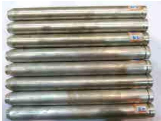
*FIG. 17. Simulated Nuclear fuel elements made from Pb and Al.*
