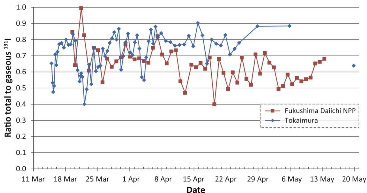
FIG. III-8. Ratio of gaseous  $^{131}\text{I}$  to total  $^{131}\text{I}$  measured at the Fukushima Daiichi site and at Tokaimura [III-19].
