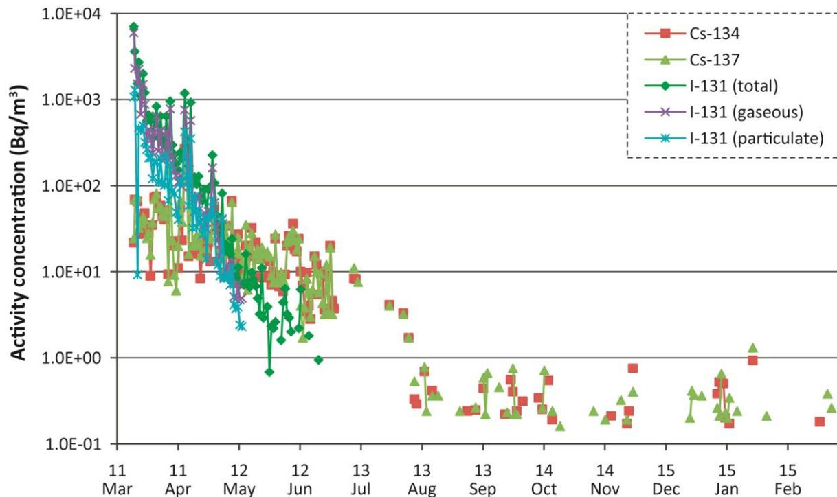
FIG. III–2. Airborne activity concentrations of  $^{134}\text{Cs}$ ,  $^{137}\text{Cs}$  and  $^{131}\text{I}$  measured at locations around the Fukushima Daiichi NPP from March to July 2011 [III–8].
