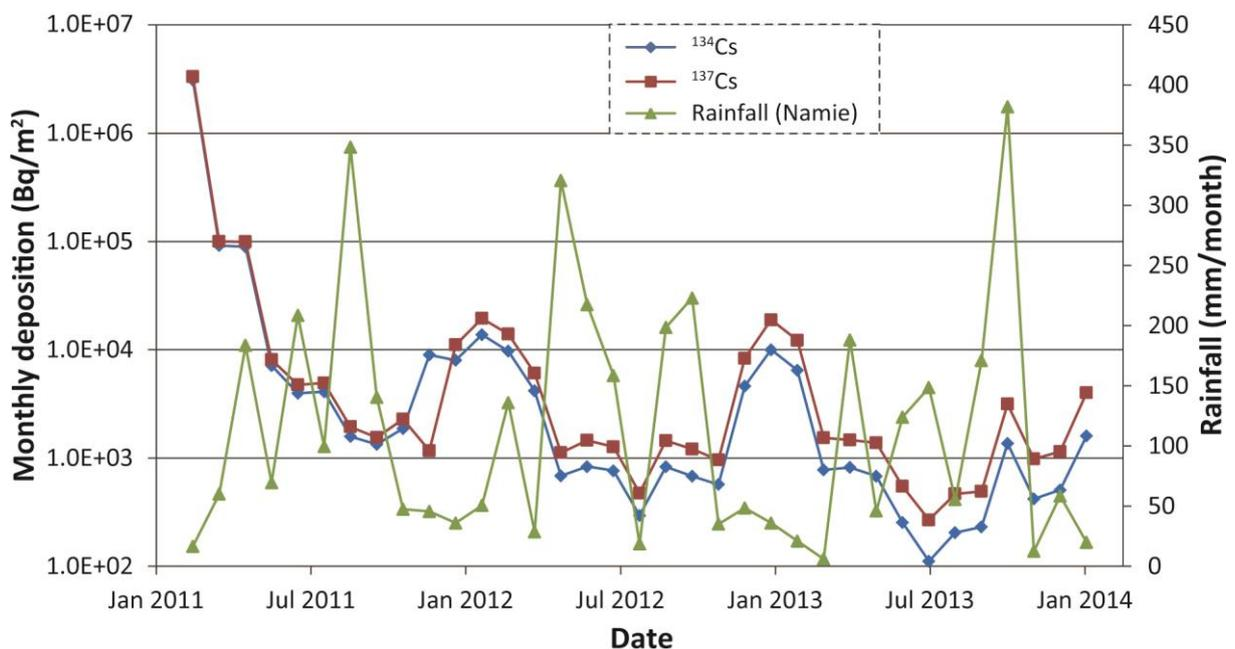
FIG. III-9. Monthly deposition rates of  $^{134}\text{Cs}$  and  $^{137}\text{Cs}$  and monthly accumulated rainfall measured in Fukushima Prefecture [III-23].
