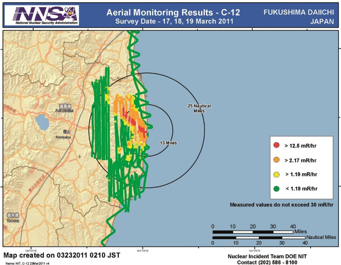
FIG. III-1. Early aerial monitoring of ambient dose equivalent rate measured from 17 to 19 March 2011 [III-3].
