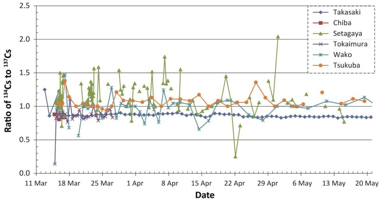
FIG. III-7. Ratios of activity concentrations of airborne  $^{134}\text{Cs}$  to  $^{137}\text{Cs}$  [III-11 to III-18].
