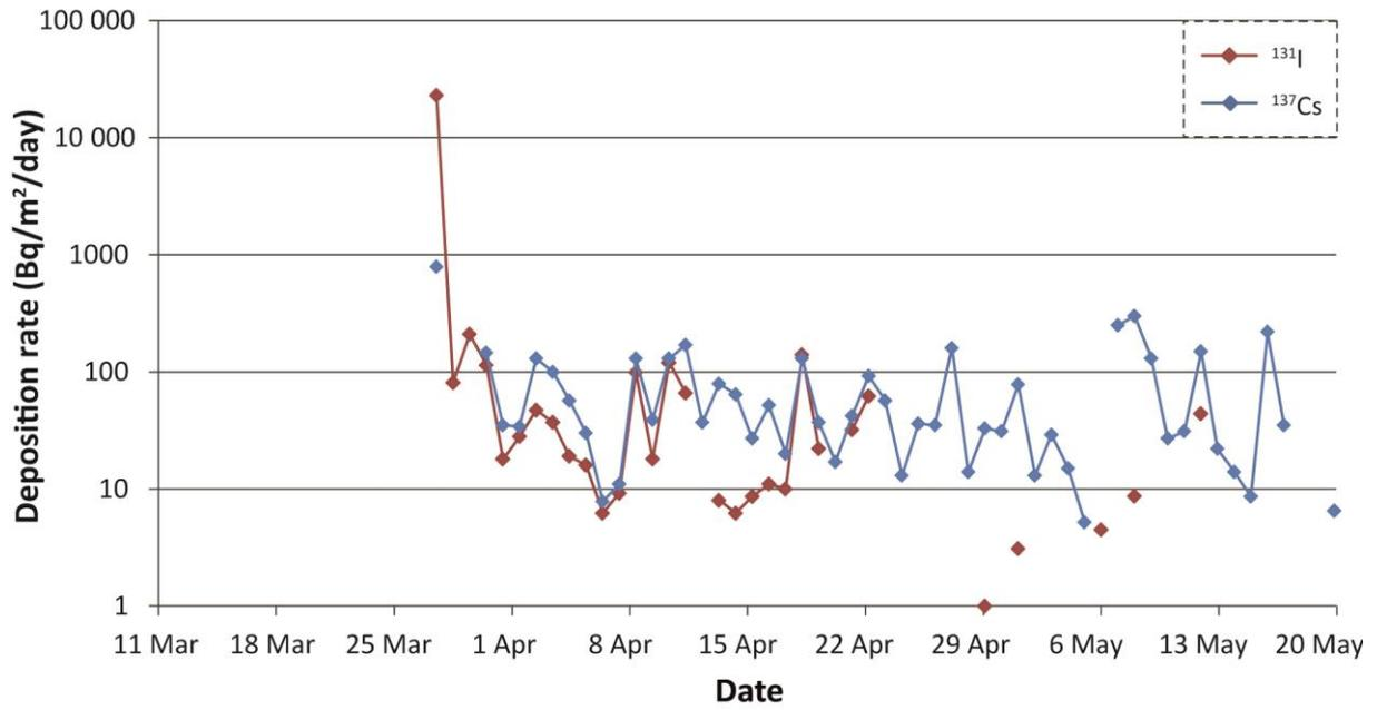
FIG. III-10. Daily deposition rates of  $^{137}\text{Cs}$  and  $^{131}\text{I}$  measured in Fukushima Prefecture, March–May 2011 [III-23].
