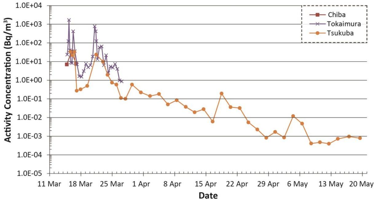
FIG. III-5. Total  $^{131}\text{I}$  activity concentration in air at various locations in 2011 [III-11, III-12, III-17, III-18].
