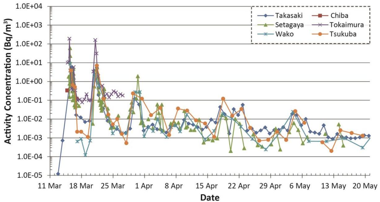
FIG. III-4.  $^{137}\text{Cs}$  activity concentrations in air at various locations in 2011 [III–11 to III–18].
