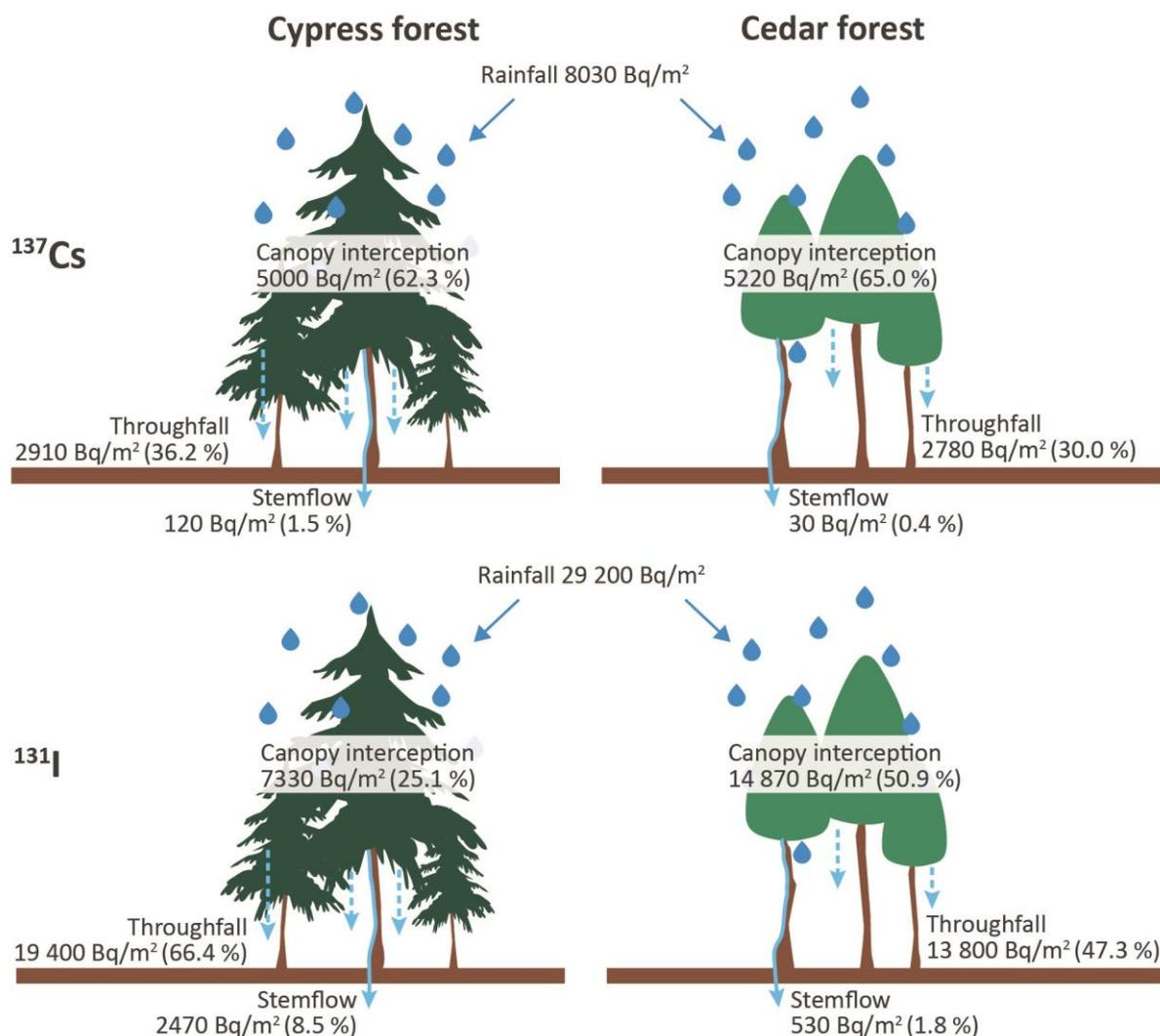
FIG. III-13. Schematic diagram of  $^{137}\text{Cs}$  and  $^{131}\text{I}$  deposition in rainwater, throughfall, and stemflow in the cypress and cedar forests [III-37].
