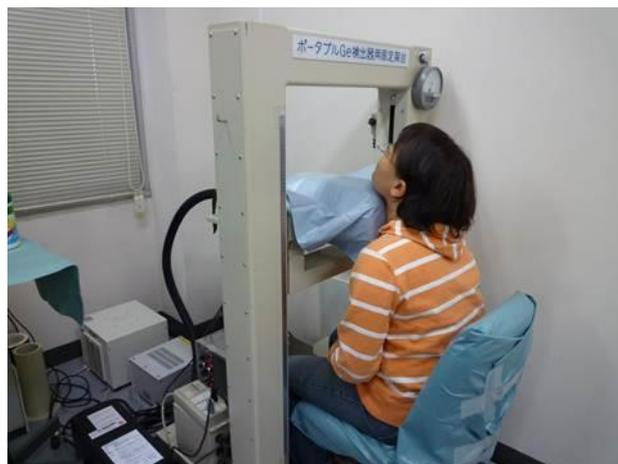
FIG. I-4. Example of a thyroid measurement device [I-5] (Photograph courtesy of National Institute of Radiological Science).
