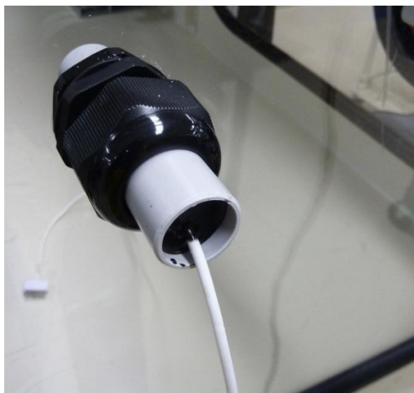
Figure 2 Glove box feed through for digital evidence cables
