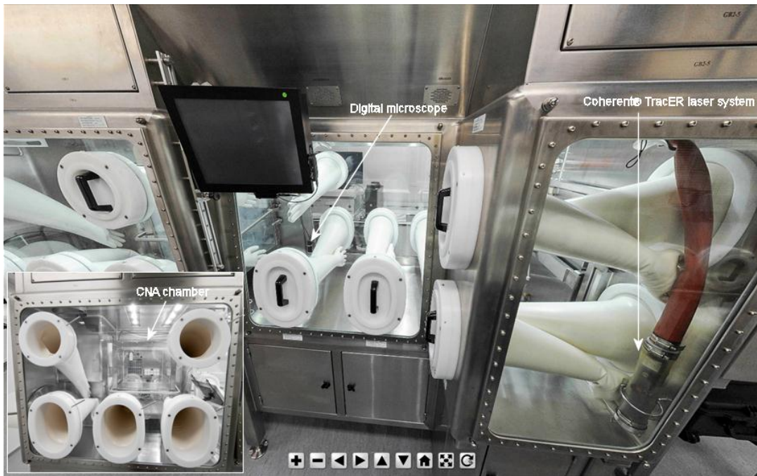
FIG 1. One of the glove box units housed within the CFAC laboratory. The digital microscope for imaging and the integrated Coherent® TracER laser system used to support fingerprint development are visible in the image. Insert shows the integrated chamber for the cyanoacrylate (CNA) vapour treatment.
