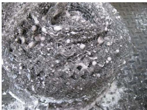
FIG. 1. Section of a woven steel wool support loaded with polluted sodium ( $\text{Na}+\text{Na}_2\text{O}+\text{NaH}+\text{NaT}$ ).
