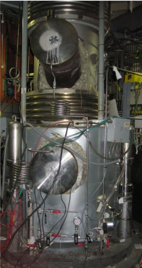
Intermediate heat exchanger isolation of the secondary loop
