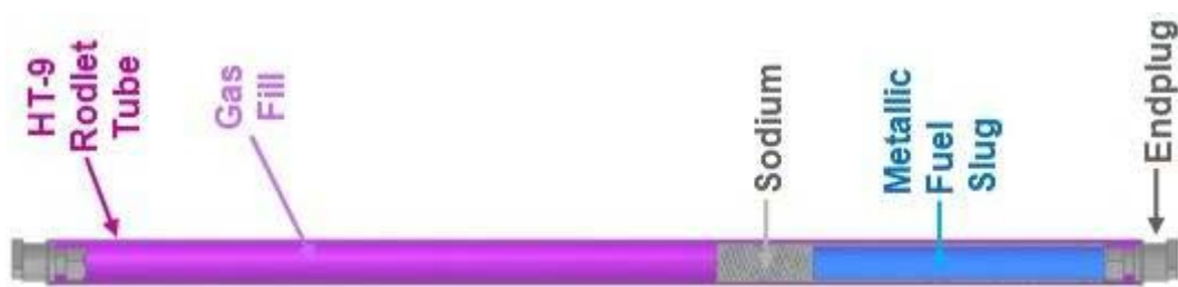
FIG. 1. Schematic of rodlet. Total length is approximately 15 cm with an outside diameter of 0.58 cm.
