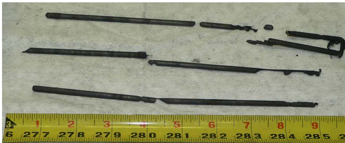
FIG. 2. Segmented depleted uranium pins cast using the BCS under a pressure differential. Note the scale shown is in inches.
