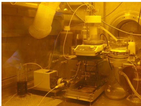
Figure 2 : Vortex precipitator and coprecipitation device in a shielded cell
