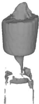
FIG. 5. Argon simulation as an adiabatic bubble passing through the melt during mold filling due to insufficient venting of the mold.
