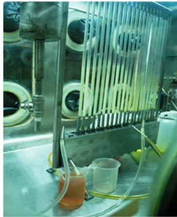
FIG. 5. A proto type 20-stage ejector mixer settler
