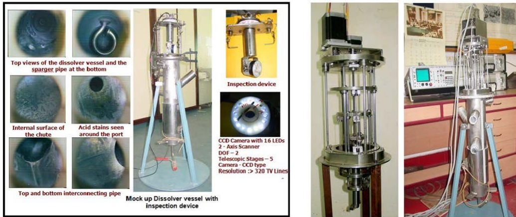
FIG. 12. a) Remote Visual inspection of CORAL Dissolver Vessel b) 2-axis telescopic scanner for dissolver wall thickness measurement using UT
