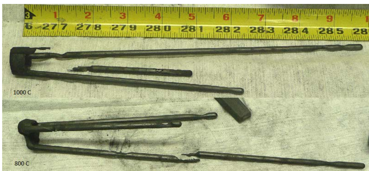
FIG. 4. Comparison of pins cast at either 1000° or 800°C mold preheat.
