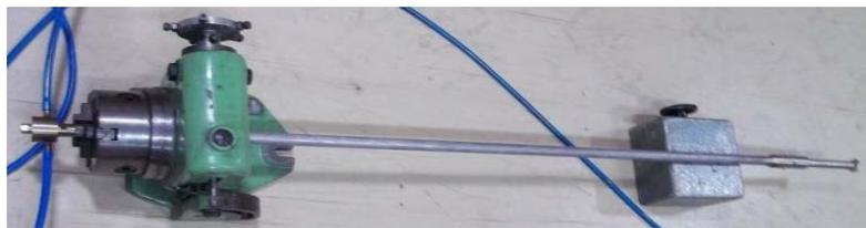
Fig.8(b) Device to fill helium filling in secondary containment
