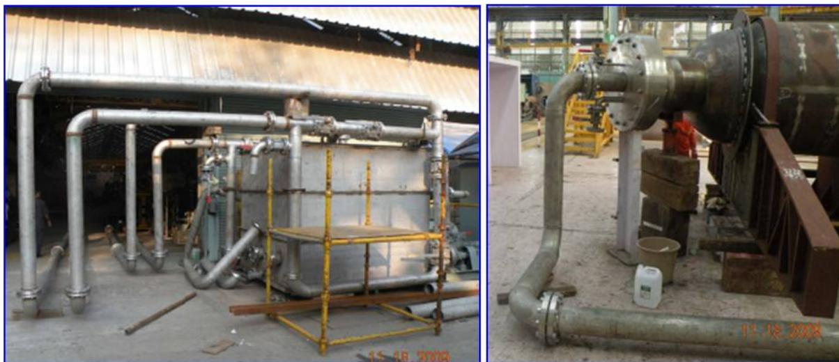
FIG. 2. Piping arrangements for degreasing of Steam Generators
