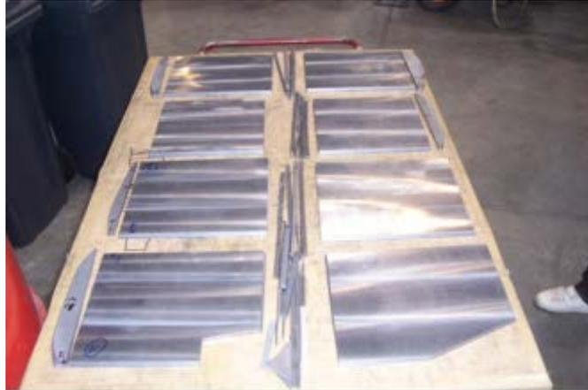
**Figure 3:** Plates of V-4Cr-4Ti CEA grade (manufactured by GfE Metalle und Materialien GmbH, Nuremberg, Germany) after cold rolling and machining [13].
