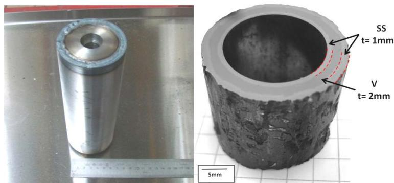
**Figure 5:** SS/V/SS billet before extrusion (left) and piece of the "triplex" rod after extrusion (right).
