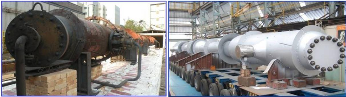
*FIG. 8. Surface appearance of SG after PWHT and after shot blasting & painting*
