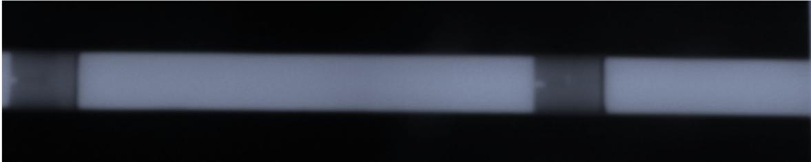
*Fig 8(c) Neutron radiograph of Fe-B capsule before irradiation*
