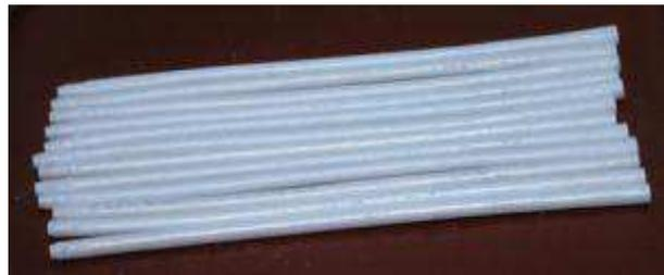
FIG. 6. Simulators of oxidized fragments of fuel rod claddings.
