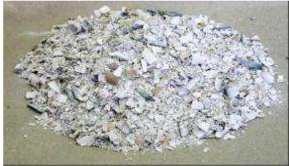
FIG. 4. Grinded  $ZrO_2$ .
