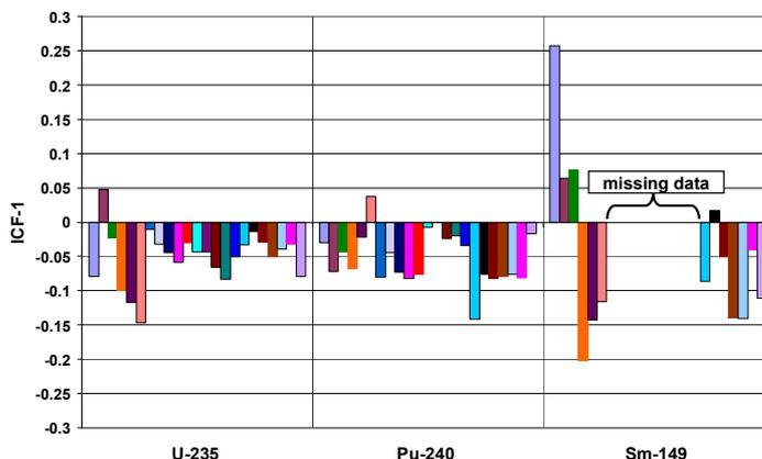
FIG. 2. Examples of the variations of the Isotopic Correction Factors (ICFs) obtained from different chemical assay measurements. The isotope  $^{149}\text{Sm}$  has not been observed in all of the evaluated measurements, i.e. the ICF data set is incomplete with respect to the total number of evaluated measurements.
