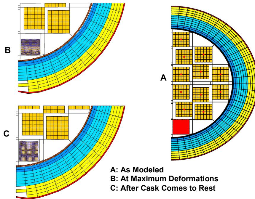
FIG. 11. End snapshot view of cell 24 assembly deformations at maximum response and after cask comes to rest.
