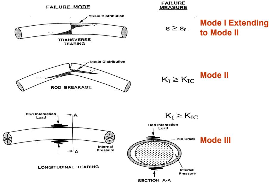
FIG. 1. Possible failure modes under cask drop.
