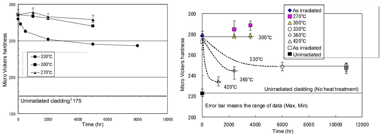
FIG. 9. Irradiation-hardening recovery property.
