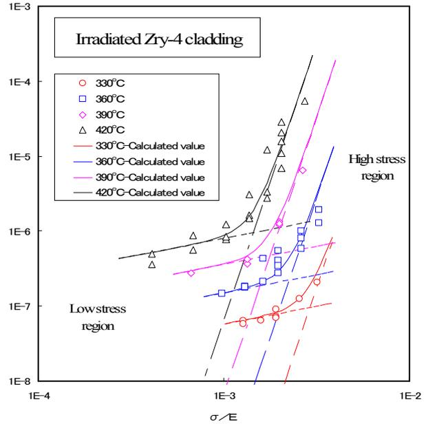
FIG. 5. Stress dependency of secondary creep rate (Hoop stress,  $E$ : Young's modulus).
