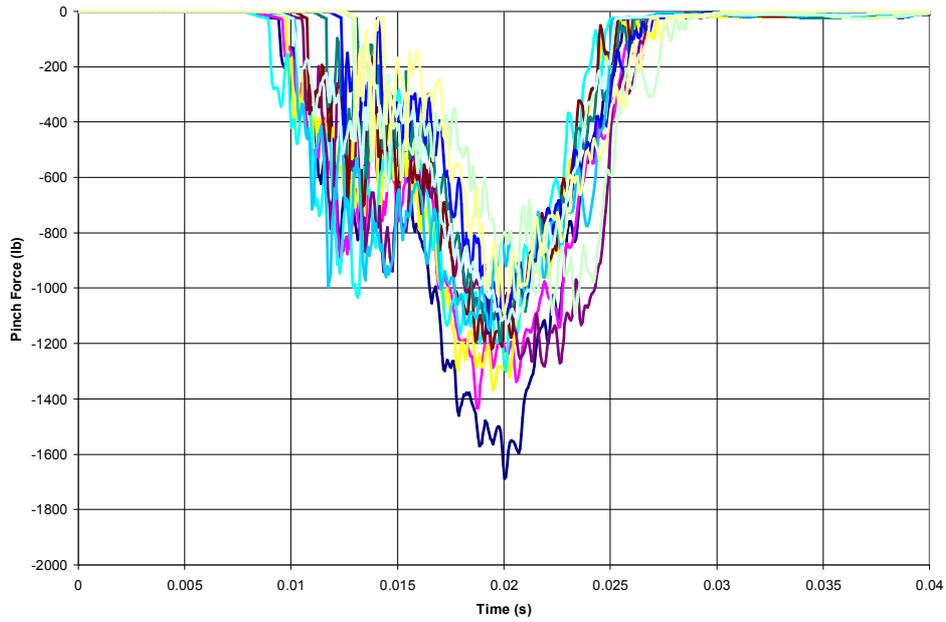
FIG. 5. Assembly 22 maximum pinch force time histories at spacer grid.
