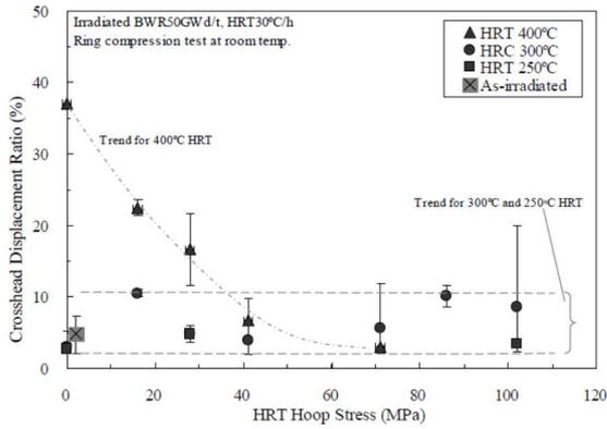
FIG. 7. Correlation between the degree of reorientation and the HRT conditions for irradiated BWR Zry-2 cladding with Zr liner.
