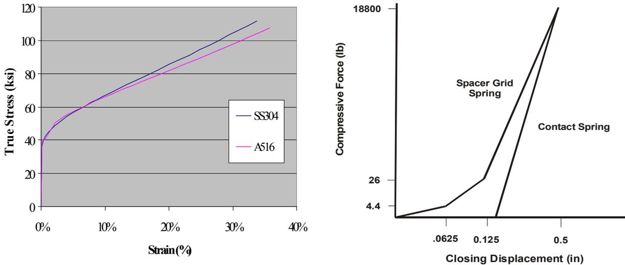
FIG. 4. (a): Stress-strain curve for steel materials and (b): force-displacement model for spacer grid springs & rod-to-rod contact springs.
