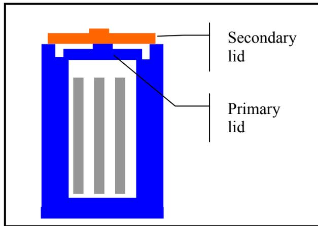
FIG. 1. Double-lid design principle.
