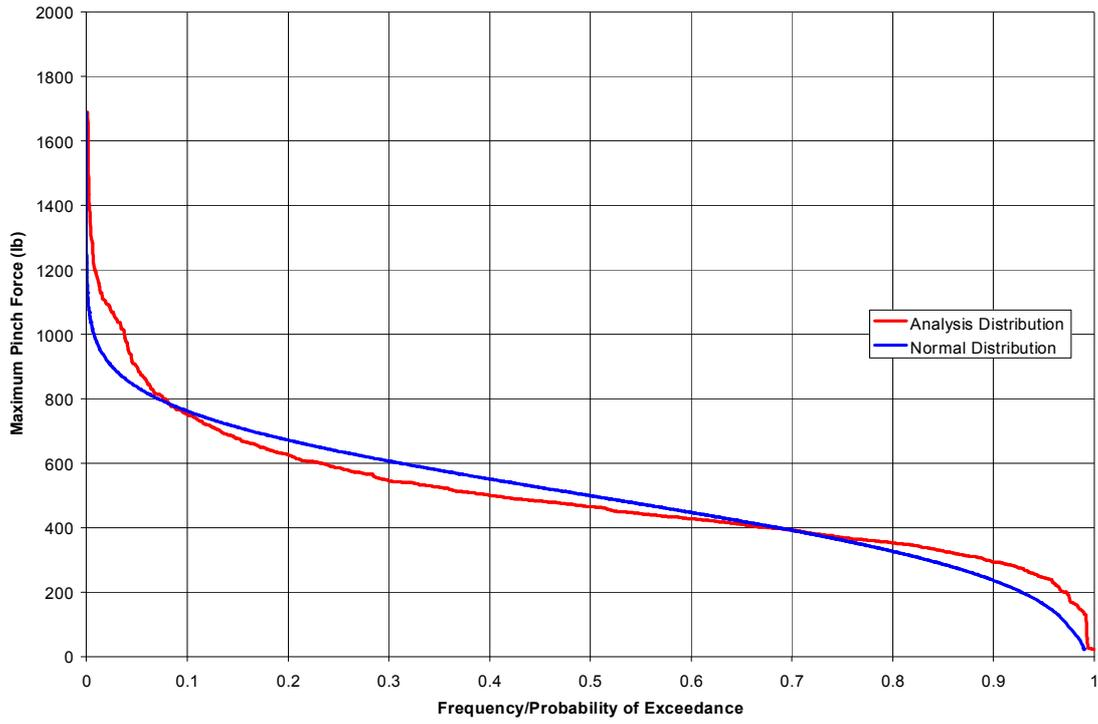
FIG. 7. Maximum pinch force frequency/probability distribution — spacer grid.
