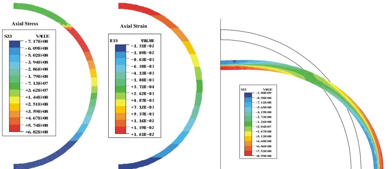
FIG. 12. Axial stress and axial strain distributions in the guide tube at maximum force & moment
