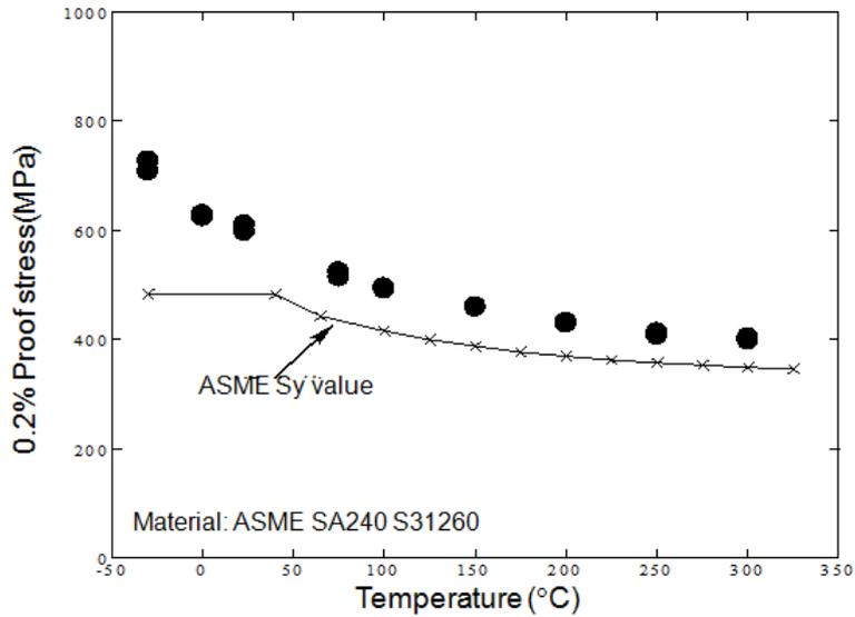
FIG. 11. Comparison between 0.2% Proof Stress and ASME Sy Value of ASME SA240 S31260.
