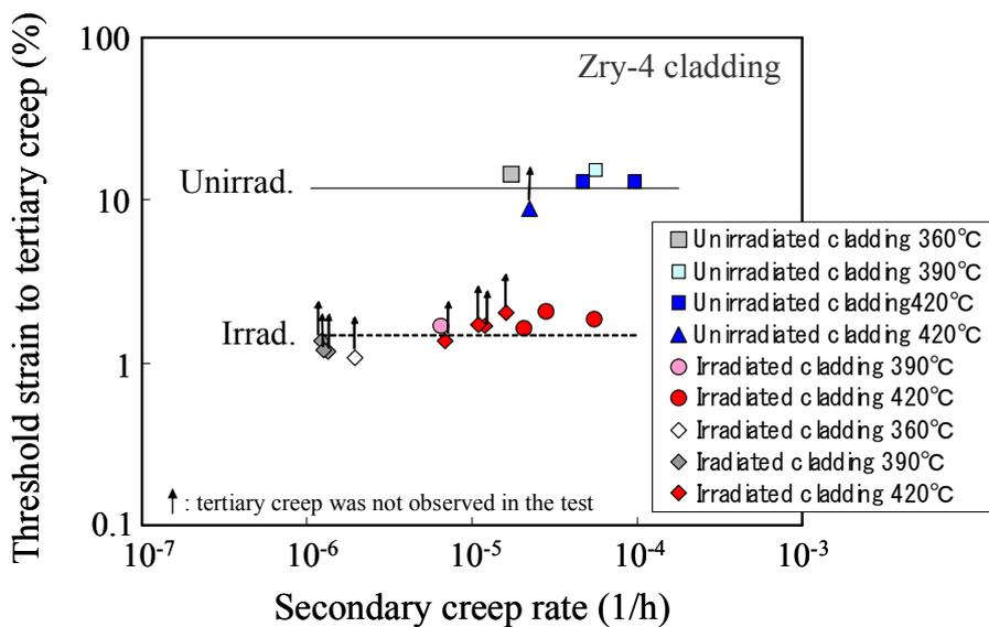
FIG. 6. Relation between threshold strain to tertiary creep and secondary creep rate (Zry4).
