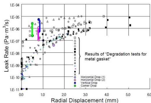
FIG. 4. Leak rate vs. relative radial displacement of lid.
