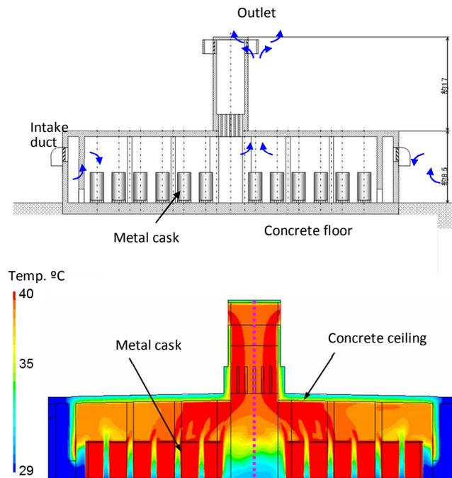
FIG. 10. Temperature profile calculated by FLUENT.
