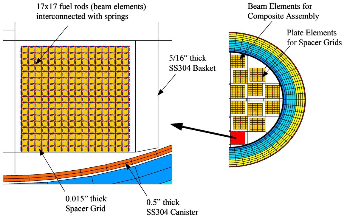
FIG. 3. 3D Centre spacer grid slice models.
