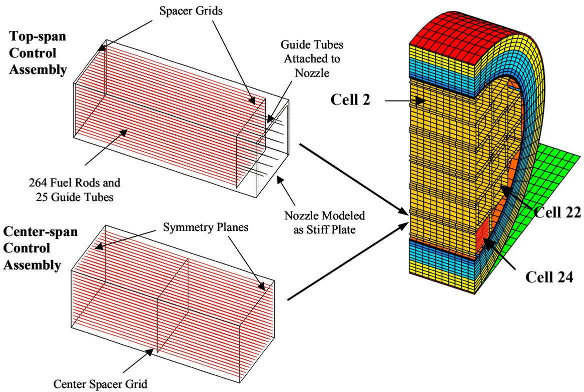
FIG. 2. Fuel assembly models within a three-dimensional slice of the global model.
