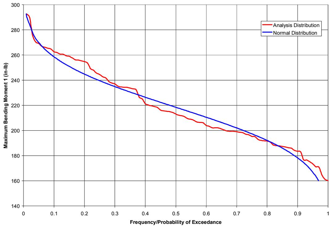
FIG. 8. Maximum bending moment 1 frequency/probability distribution top plate model.
