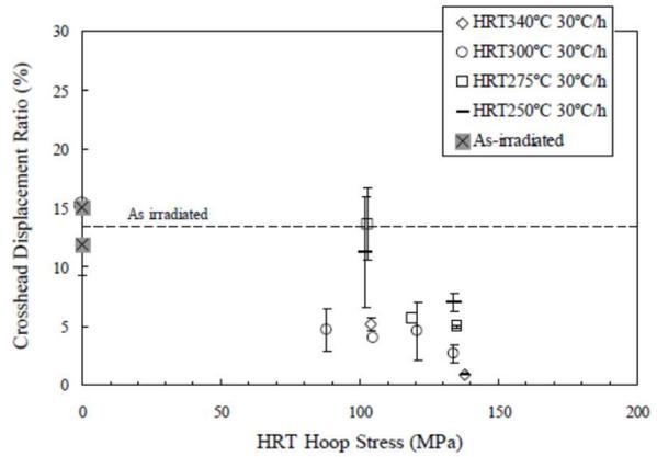
FIG. 8. Correlation between the degree of reorientation and the HRT conditions for irradiated PWR Zry-4 cladding.
