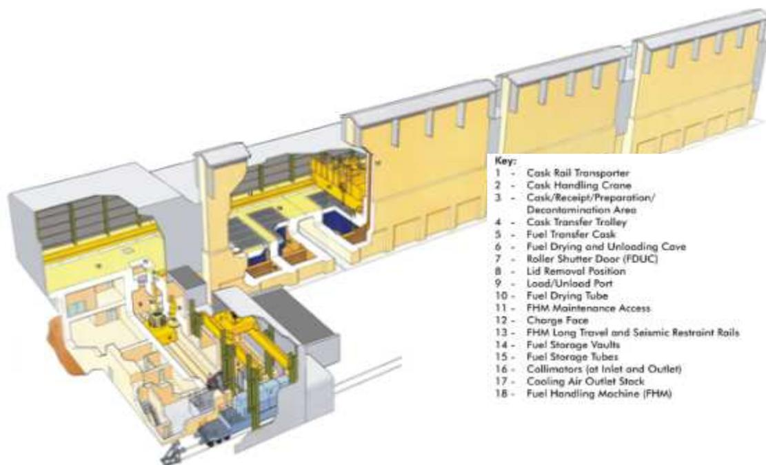
FIG 1. The layout of the Modular Vault Dry Storage facility.
