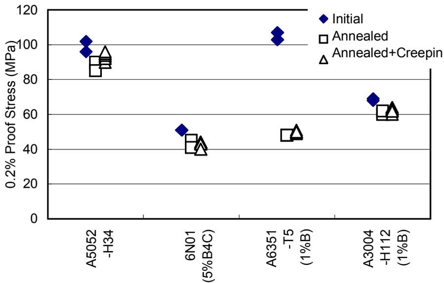
FIG. 1. Comparison of proof strength (at 250°C).
