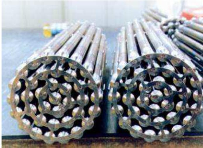
*FIG. 4. A typical 37 rod CANDU fuel element.*
