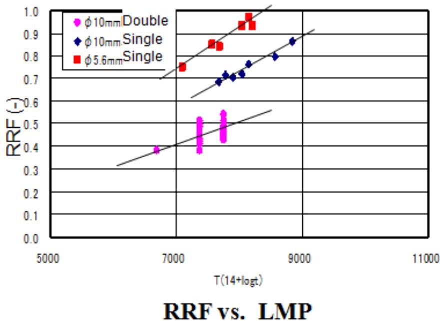
FIG. 3. Reduction ratio of reaction force vs. LMP.
