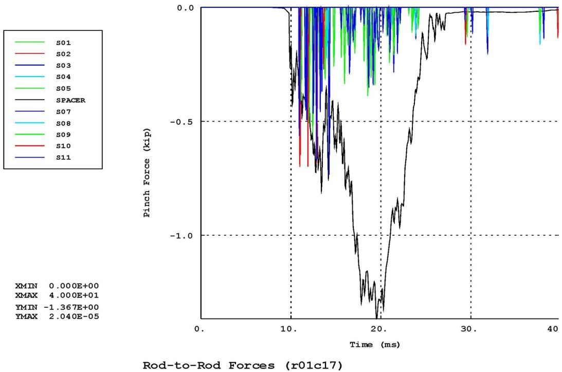
FIG. 6. Cell 22 Maximum rod-to-rod contact force time history at mid-span.
