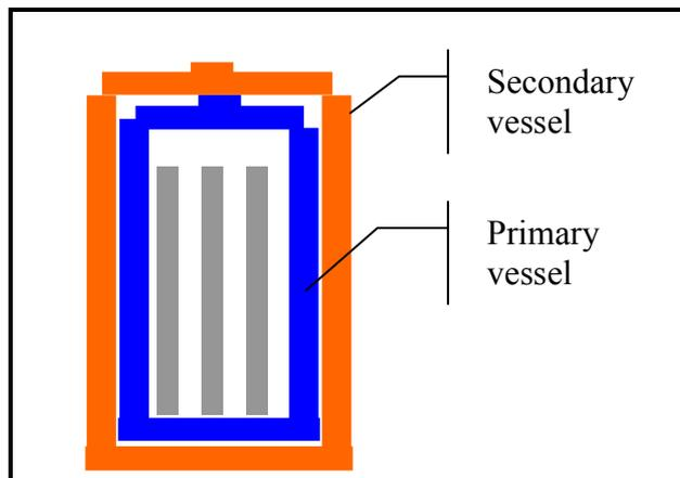
FIG. 2. Double-vessel design principle.
