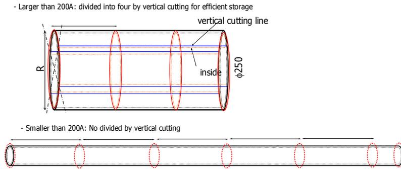
FIG. 53. Segmentation model for piping in DecDose.
