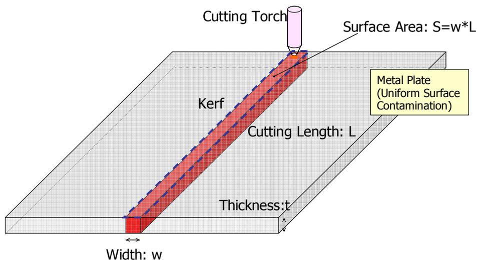
FIG. 28. Dispersed model during cutting activity for surface contaminated plate in DecDose.
