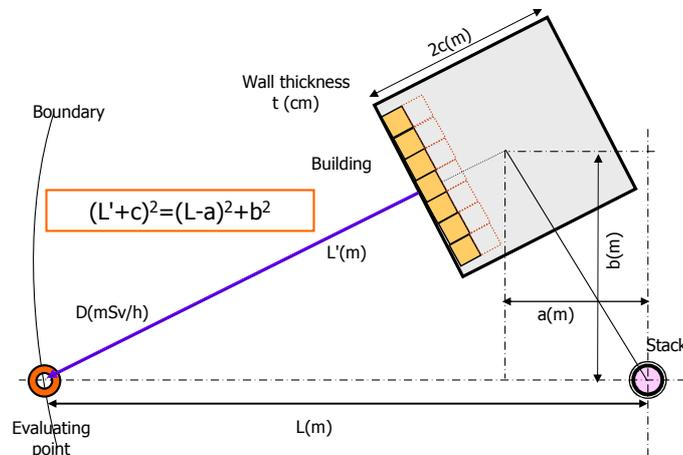
FIG. 54. Concept of the modelling for direct radiation from wastes.
