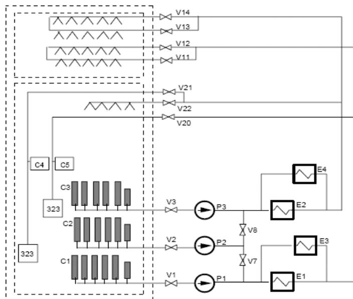
FIG. 15. Schematic of containment spray system 322.
