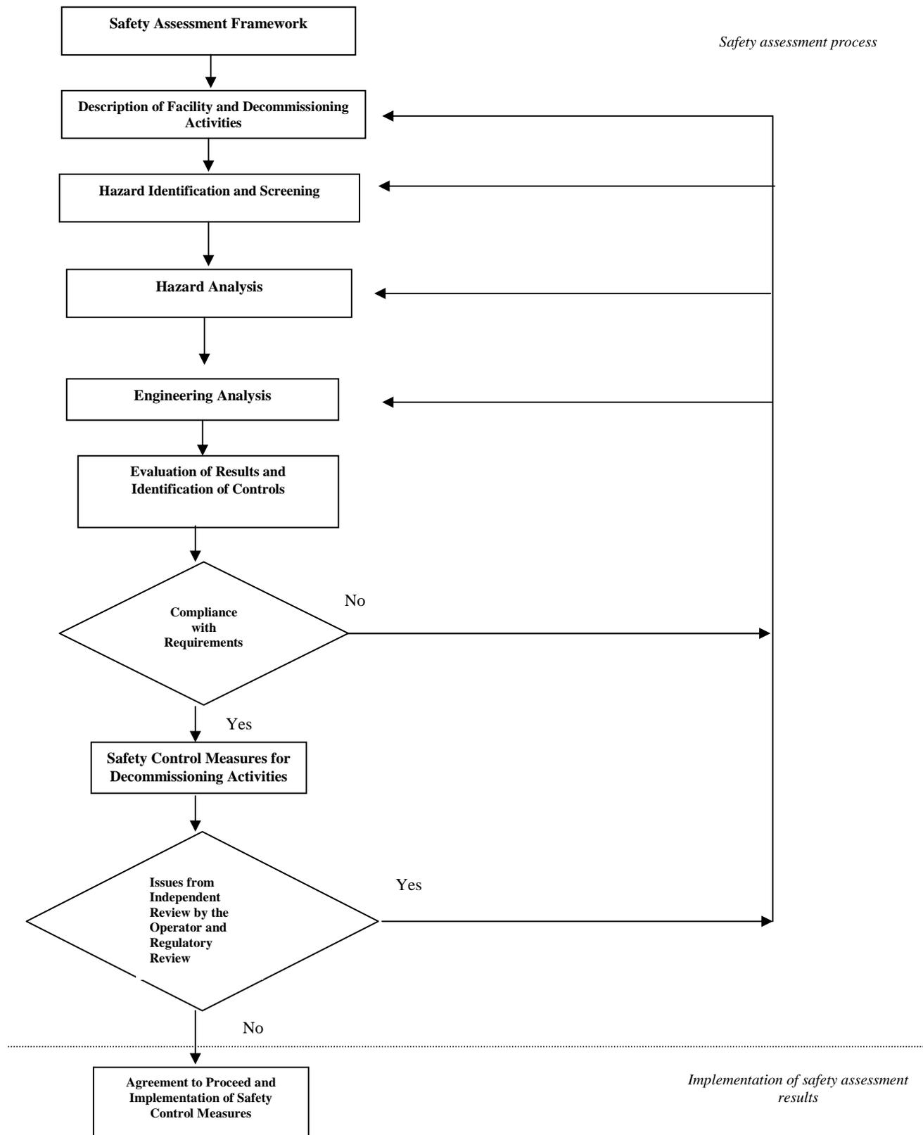
FIG. 4. The safety assessment methodology applied to the NPP Test Case.
