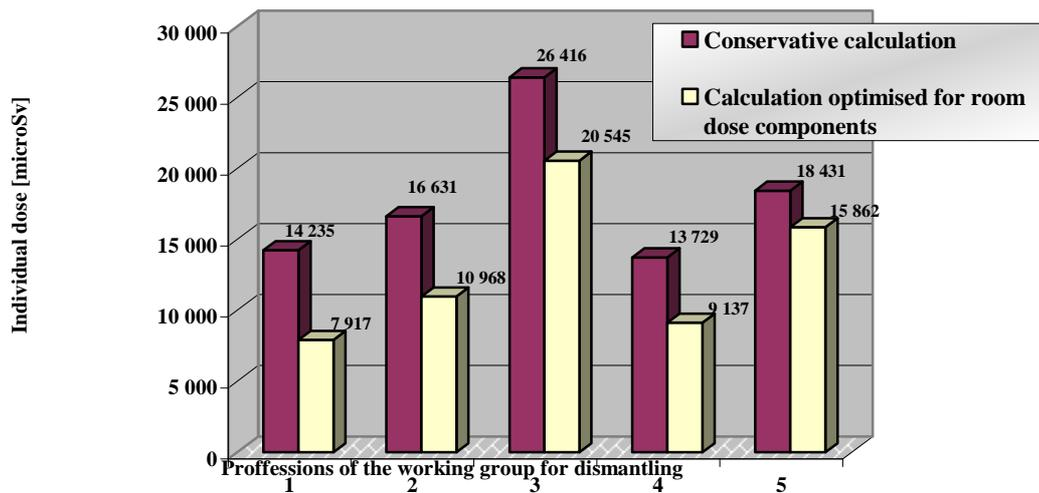
FIG. 44. Demonstration of optimization of dose uptake calculation versus conservative calculation.
