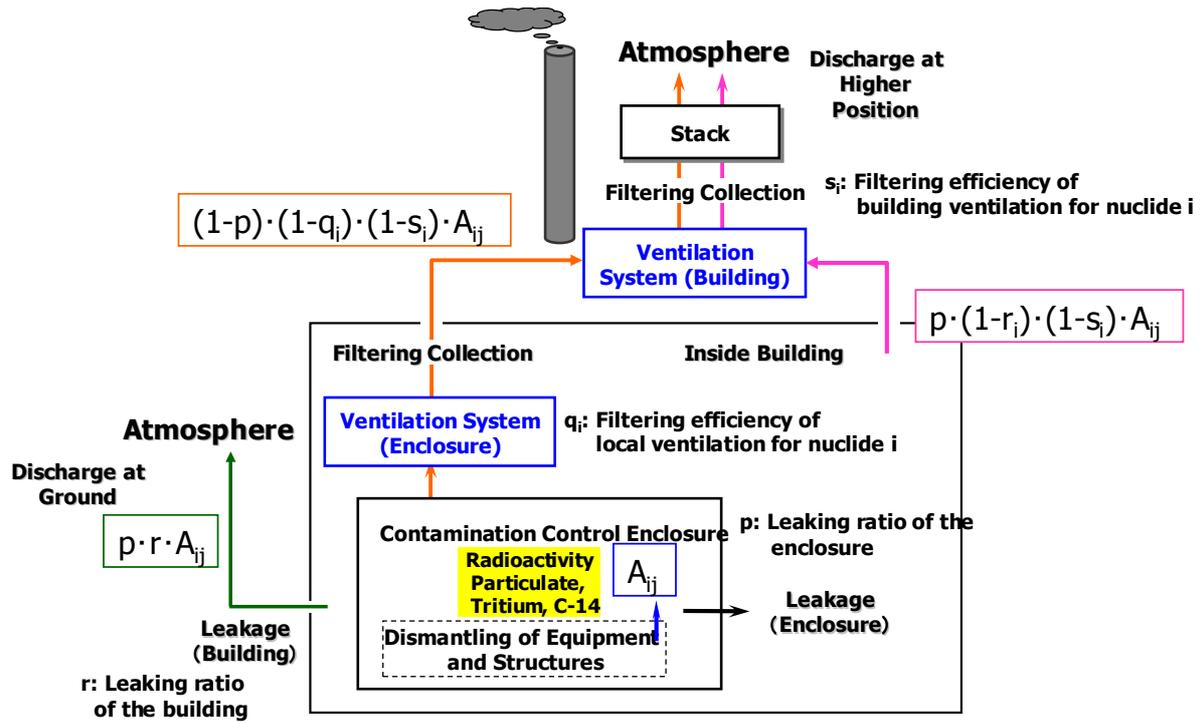
FIG. 29. Discharge routes from enclosure to the atmosphere in DecDose.
