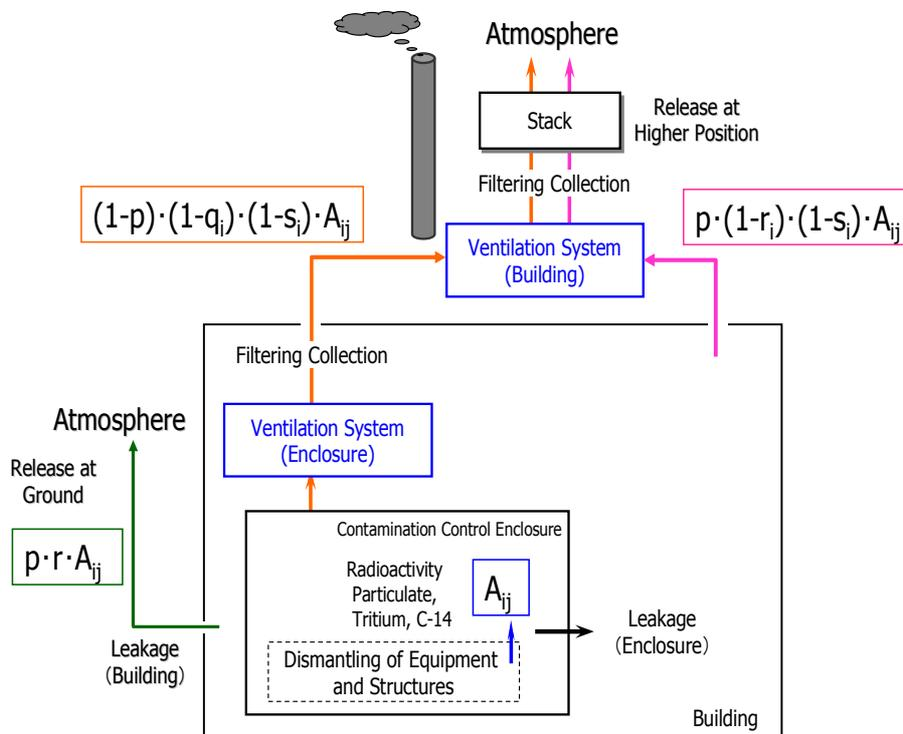
FIG. 52. Discharge routes to the atmosphere.
