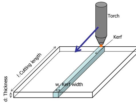
FIG. 51. Model for cutting of plate with activation and contamination.
