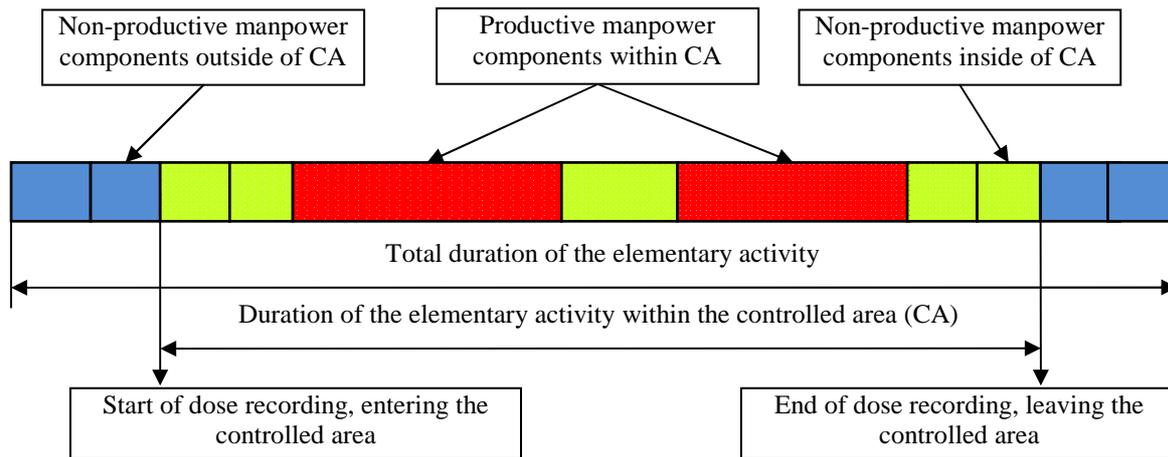
FIG. 38. Model working time structure of a specific decommissioning activity.
