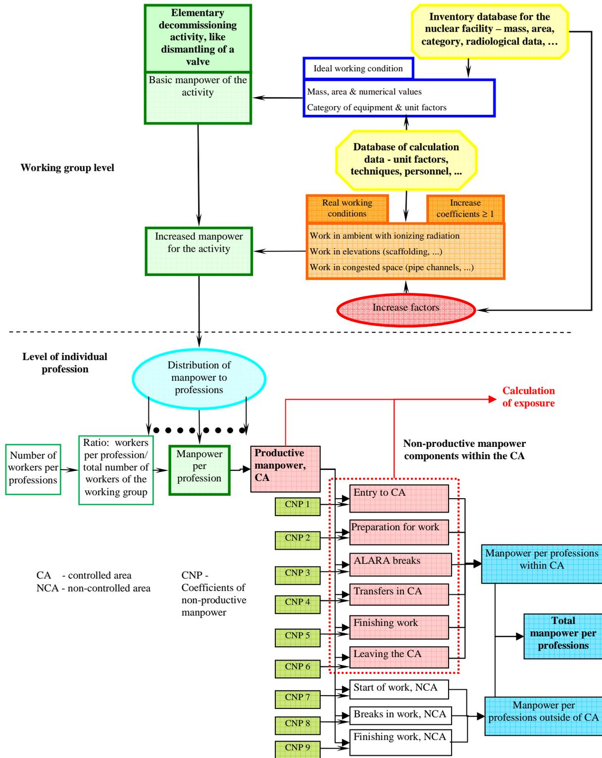
FIG. 40. The principal scheme for calculation of specific manpower components.
