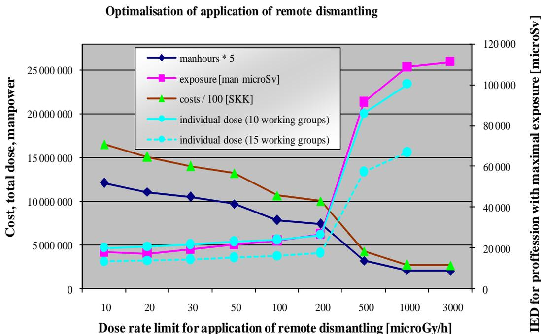
FIG. 45. Evaluation of costs for dismantling of the primary circuit of A1 NPP versus dose uptake by varying the limit for application of remote dismantling.
