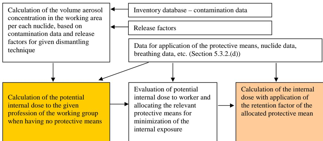
FIG. 23. Principle of calculation of internal dose during dismantling.
