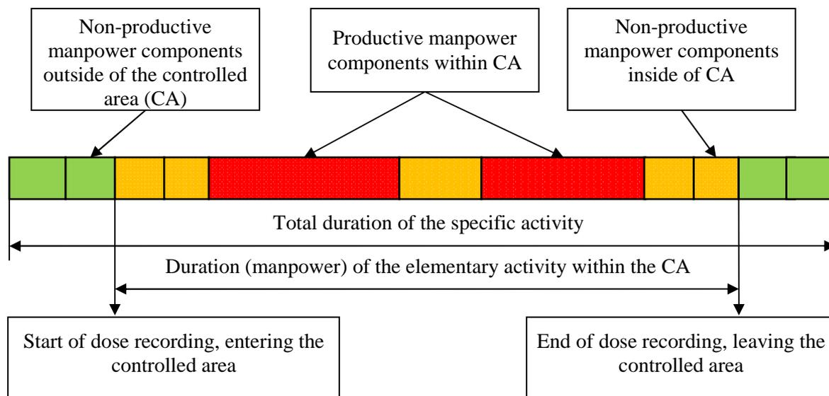
FIG. 24. Model working time structure for calculating the dose to workers.
