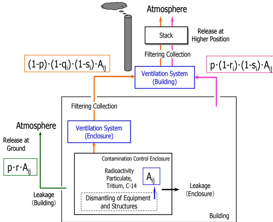
FIG. 52. Discharge routes to the atmosphere.
