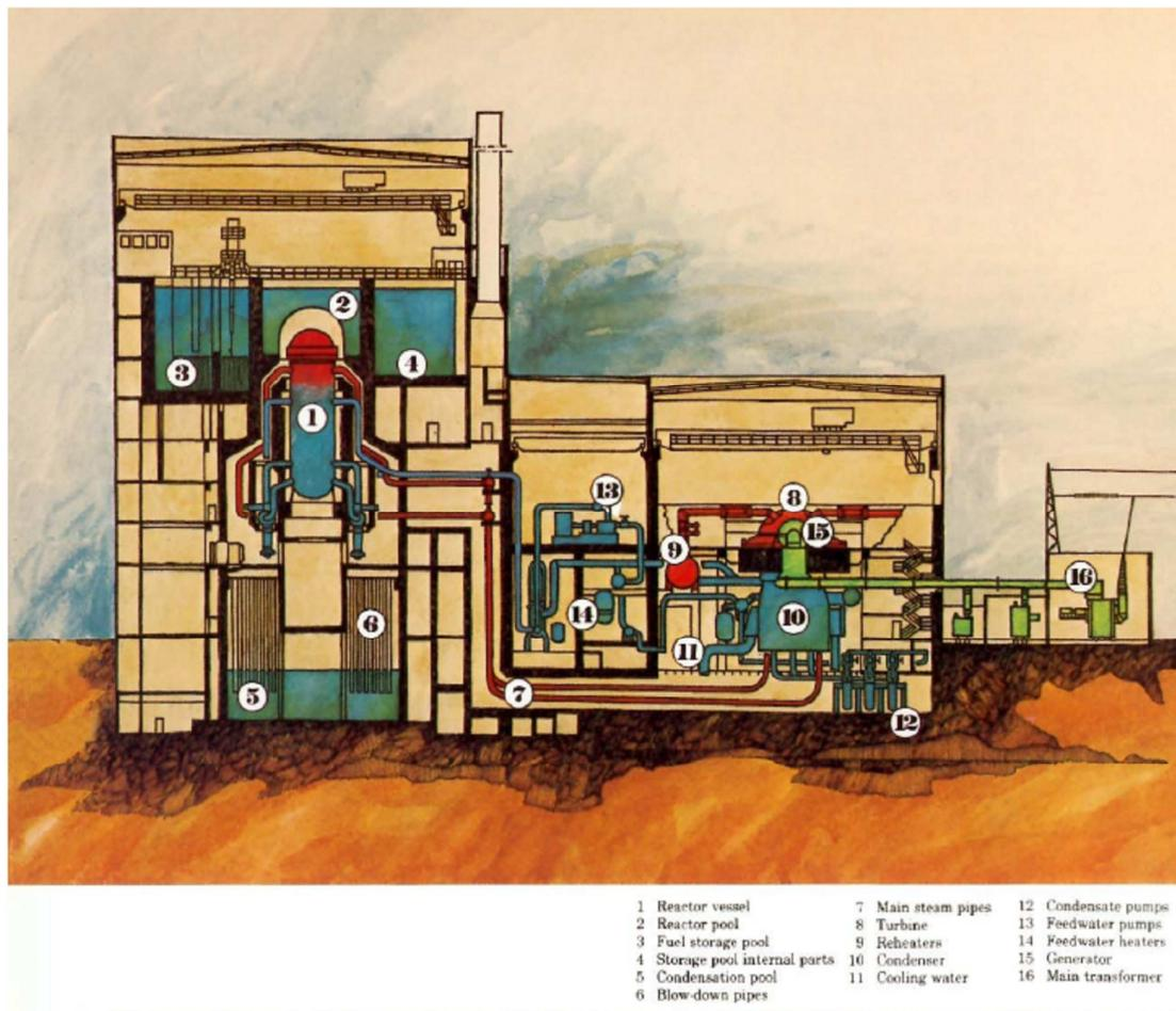
FIG. 8. Vertical cross-section of unit 1
