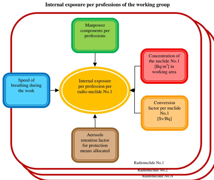
*FIG. 43. Calculation procedure for internal exposure.*
