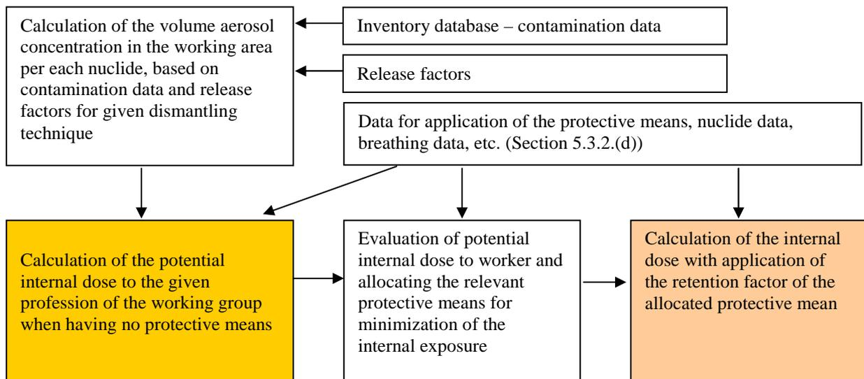
FIG. 23. Principle of calculation of internal dose during dismantling.
