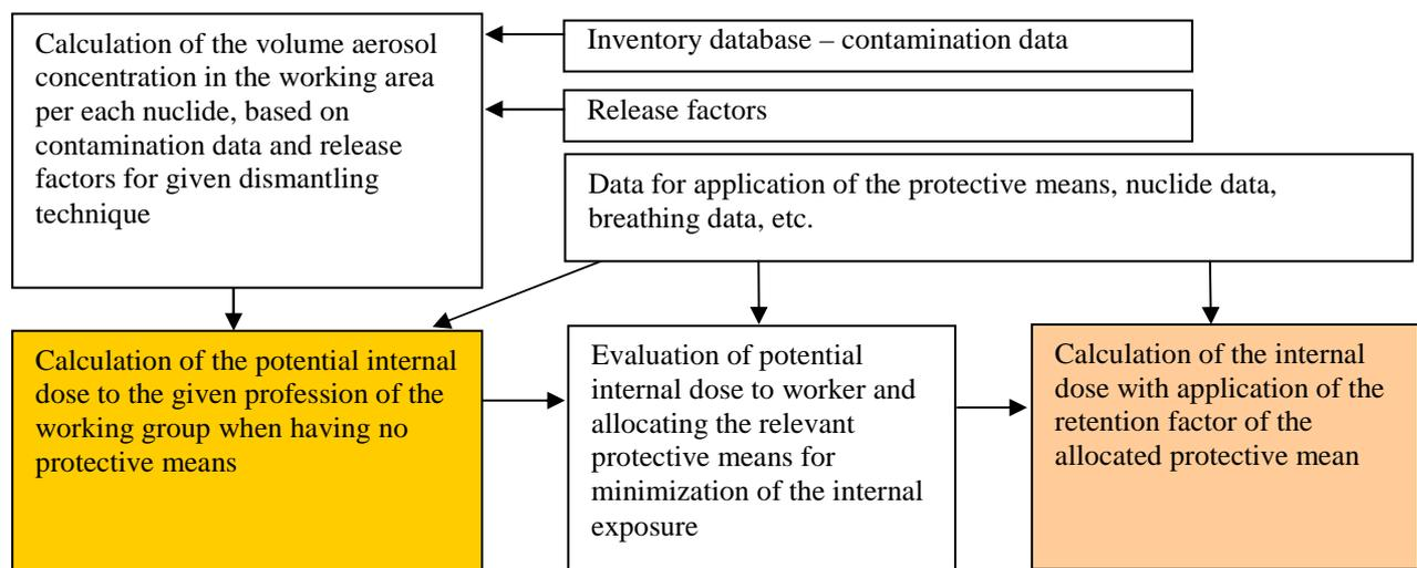
FIG. 42. Principle of calculation of internal dose during dismantling.
