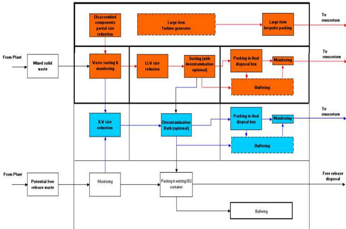
FIG. 20. NPP waste processing and package facility.
