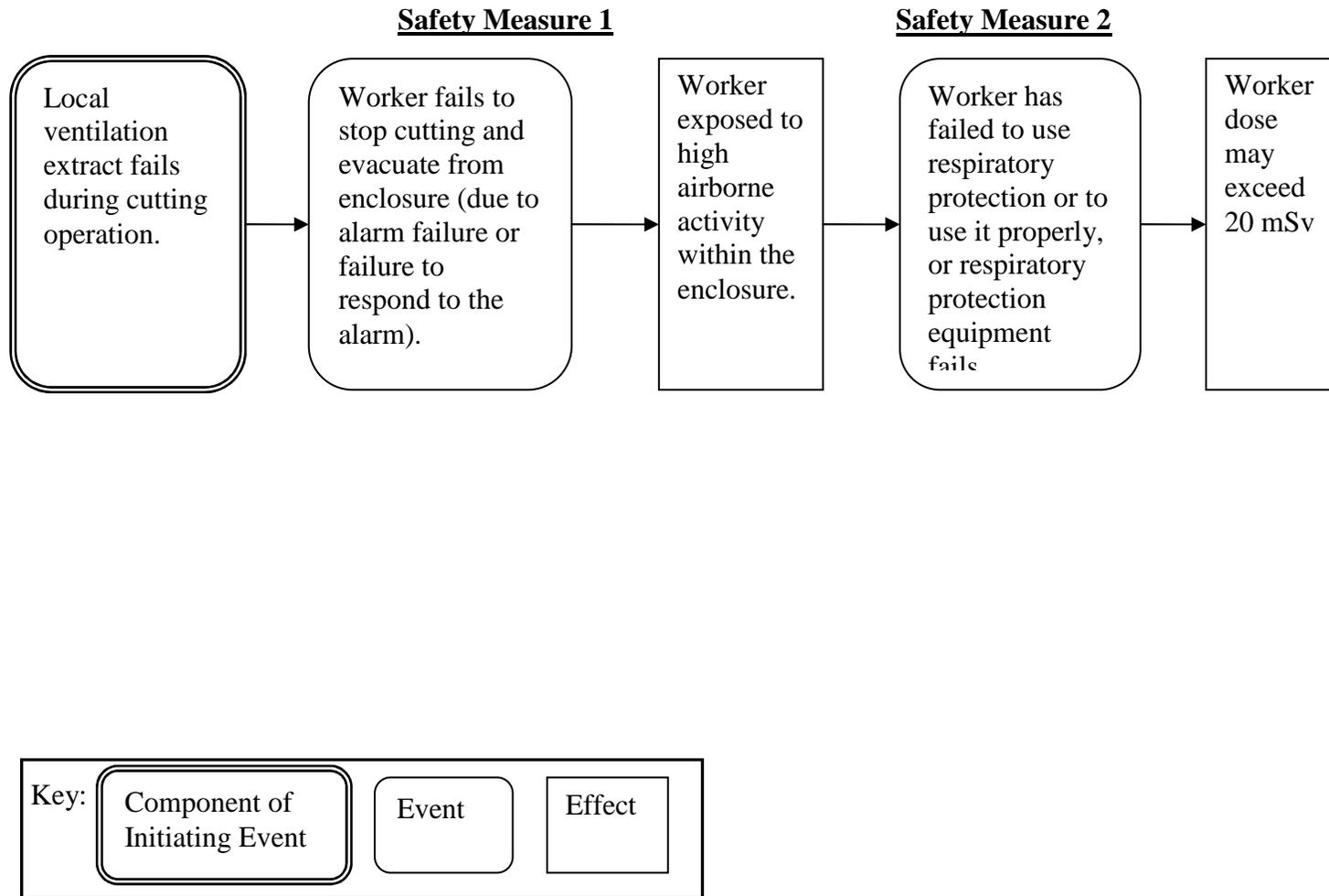
FIG. 56. Scenario progression diagram for faults during cutting operations.
