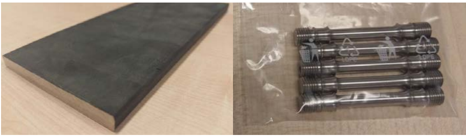
FIG. 73. Left: a segment of MONICR plate as supplied by the Research Centre Řež; right: tensile samples fabricated at the Research Centre Řež from the same material (courtesy of R. Hania, NRG).
