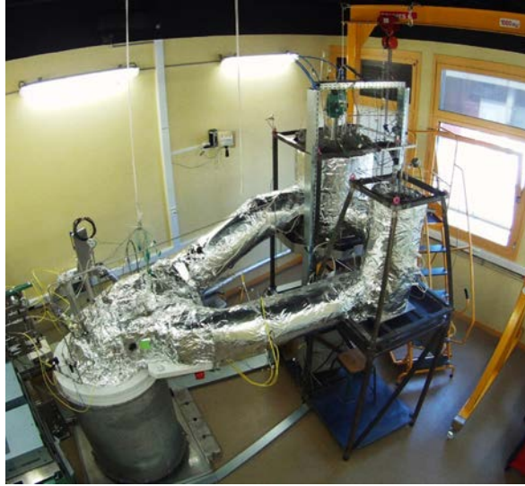
FIG. 58. View of the FFFER facility with thermal insulation around the pipes (courtesy of E. Merle, Laboratoire de Physique Subatomique et de Cosmologie).
