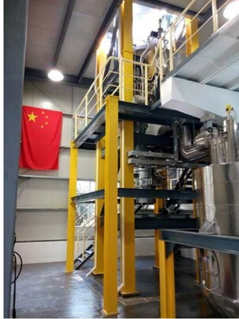
FIG. 13. Overall layout of the nitrate natural circulation experiment loop (courtesy of Y. Zou, Shanghai Institute of Applied Physics).
