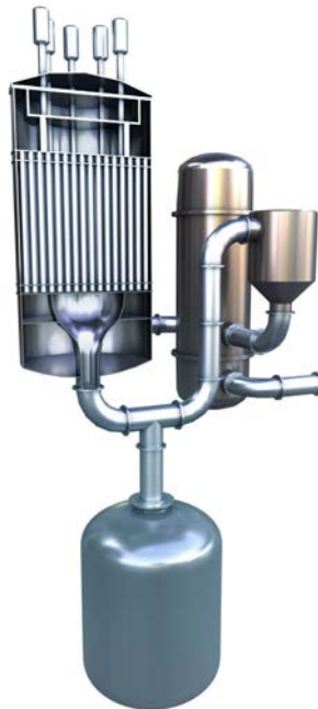
FIG. 108. Concept illustration of the CMSR primary circuit and fuel salt drain tank (reproduced from Ref. [452]).
