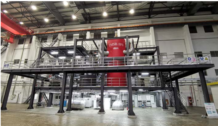
FIG. 16. Layout of the TMSR-0 simulator reactor (courtesy of Y. Zou, Shanghai Institute of Applied Physics).
