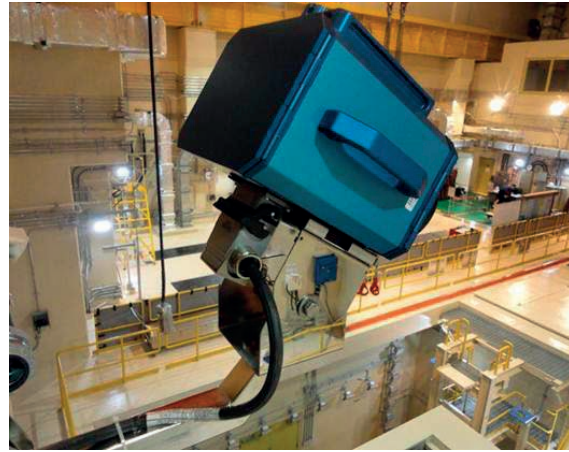
FIG. 7. A next generation IAEA surveillance system.
