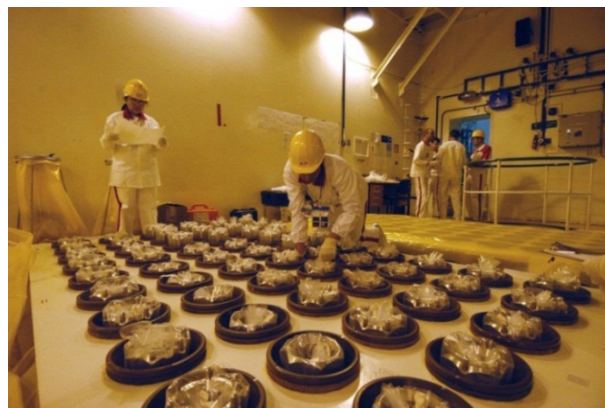
FIG. 4. Item counting in a fresh fuel store.
