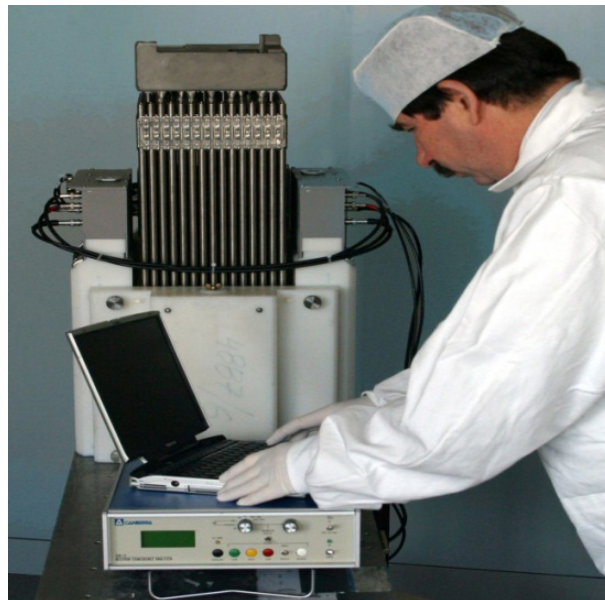
FIG. 16. Uranium neutron collar being used to measure ^{235}\text{U} content in a fuel assembly [15].
