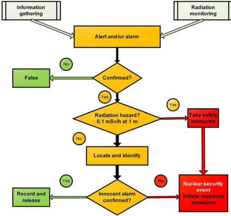
FIG. 3. Generic functional flow for initial assessment of alarms and alerts.
