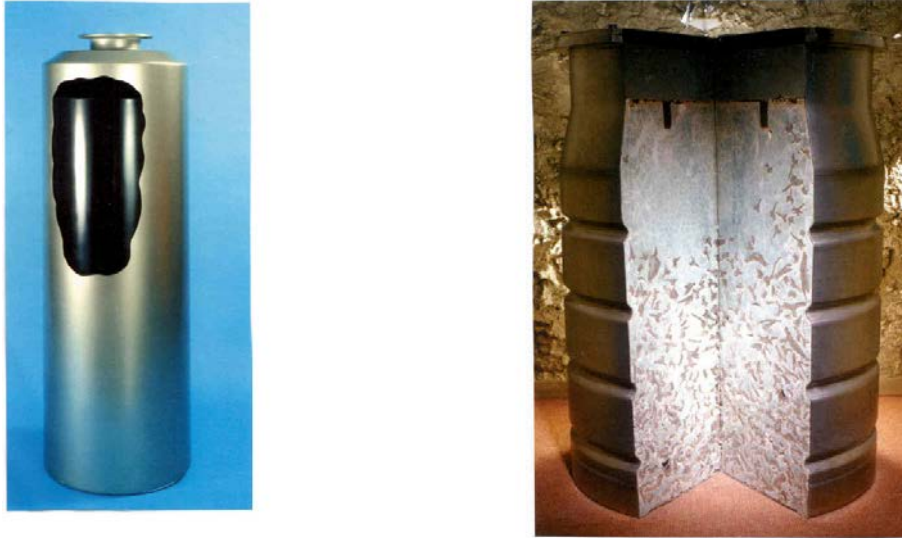
FIG. 4. Solid radioactive waste forms. Left: Cutaway showing simulated vitrified high level waste in a stainless steel production container. The container is 1.3 m high and holds about 150 L of glass. Right: Cutaway showing simulated cement encapsulated intermediate level waste from reprocessing of spent fuel (metallic fuel cladding waste) in a 500 L stainless steel drum. Several such drums might be placed in a steel or concrete box, surrounded by an additional cement matrix, for disposal. (Photographs courtesy of BNFL.)
