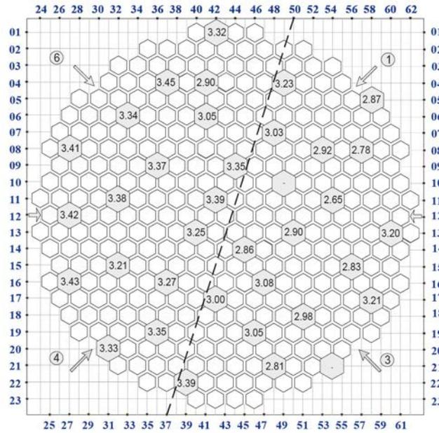
FIG. 24. Measured velocity results averaged over all the measurements.
