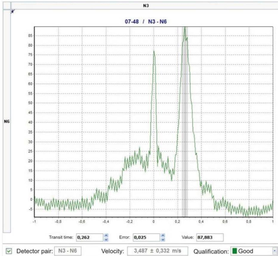
FIG. 10. Impulse response function for the estimation of transit time.
