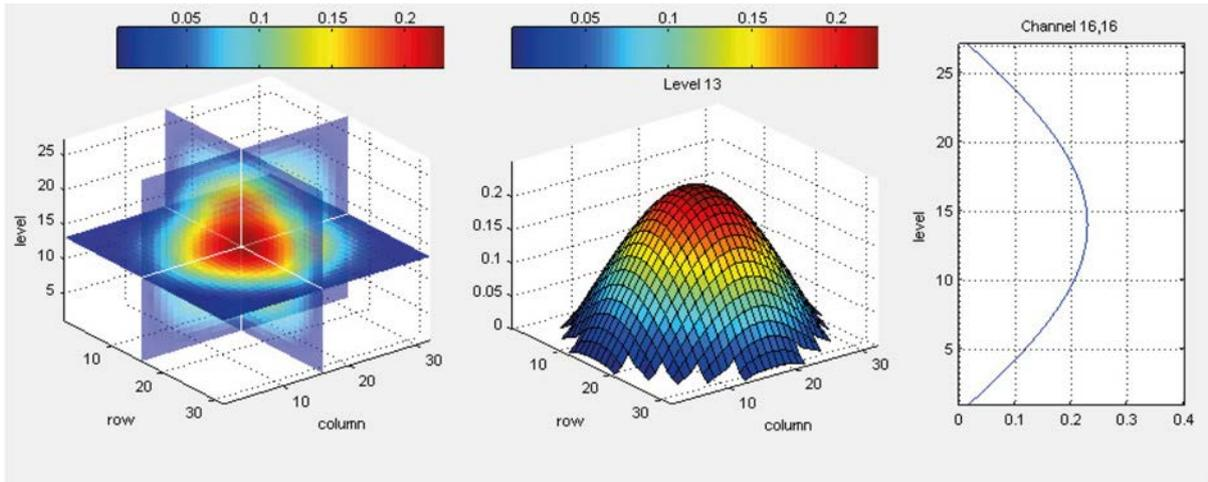
FIG. 18. Spatial distribution of the calculated static thermal neutron flux.
