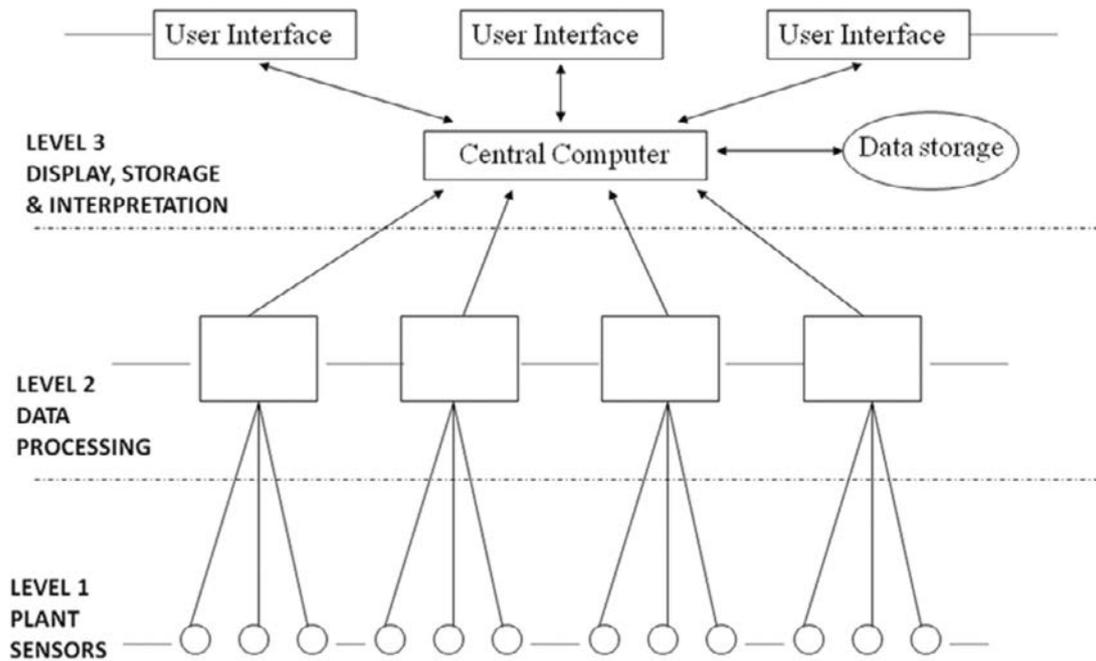
FIG. 76. Traditional approach to condition monitoring.
