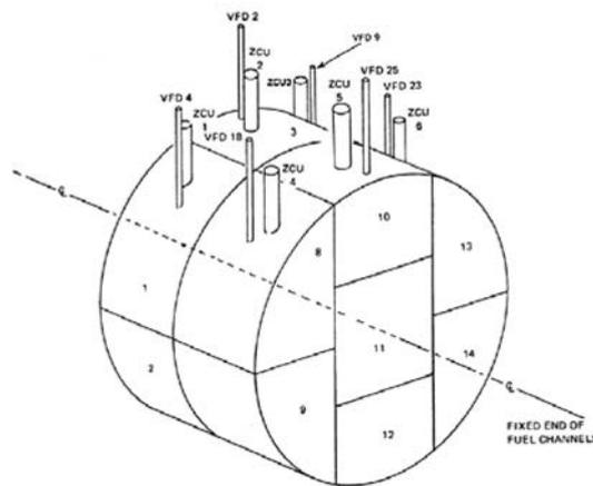
FIG. 21. Liquid zone controllers.
