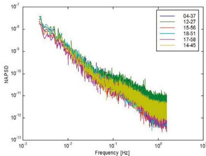
FIG. 27. Normalized APSD functions of some SPND background detector signals.
