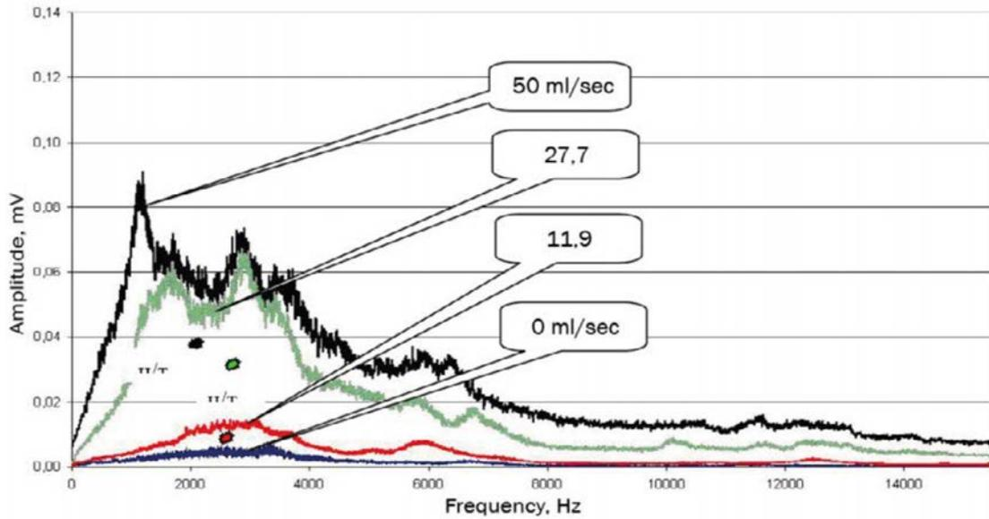
FIG. 43. Plots of ultrasonic signal spectra for different rates of leakage volume.
