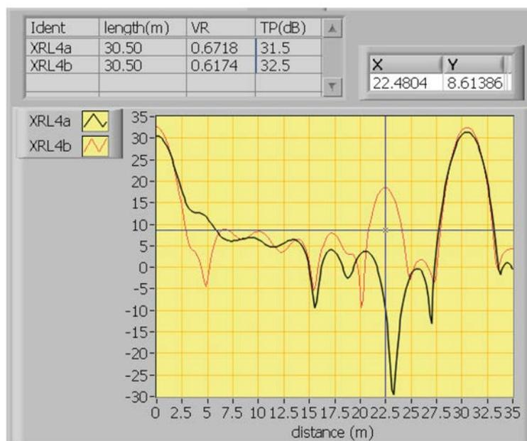
FIG. 70. LIRA measurement on XLPE before (black line) and after (red line) local thermal ageing at 22.5 m.
