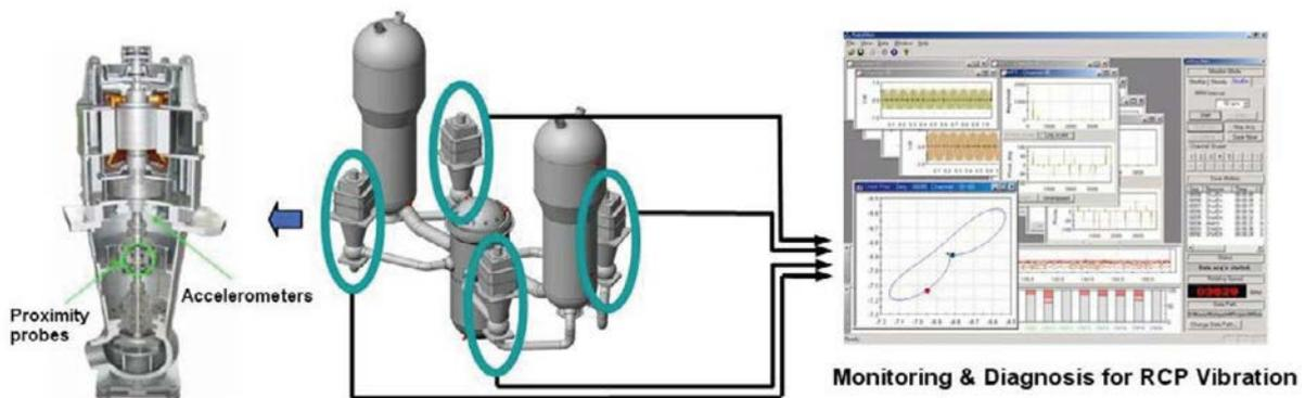
FIG. 32. Schematic of the RCPVMS.
