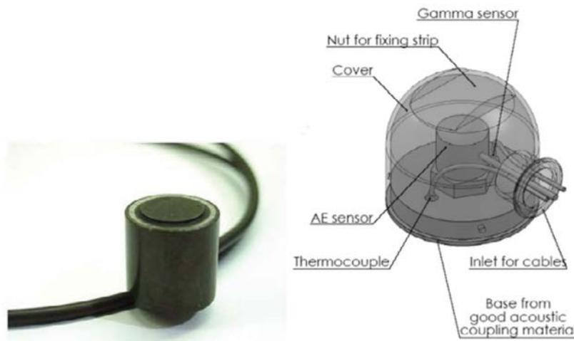
FIG. 40. Conceptual design of a radiation hardened AE sensor (D9215) and the combined sensor containing gamma detector and thermocouple.
