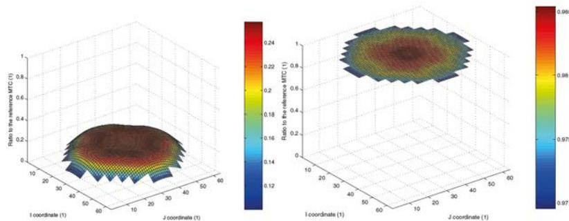
FIG. 8. Ratio between the MTC noise estimate and its actual value as calculated by CORE SIM.
