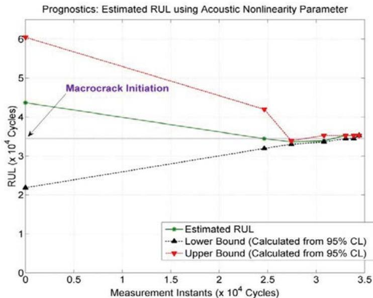
FIG. 65. Estimate of time to failure (RUL), with confidence limits (CL), from the predicted DI in Fig. 64.
