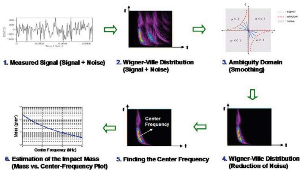
FIG. 37. A new mass estimation procedure.
