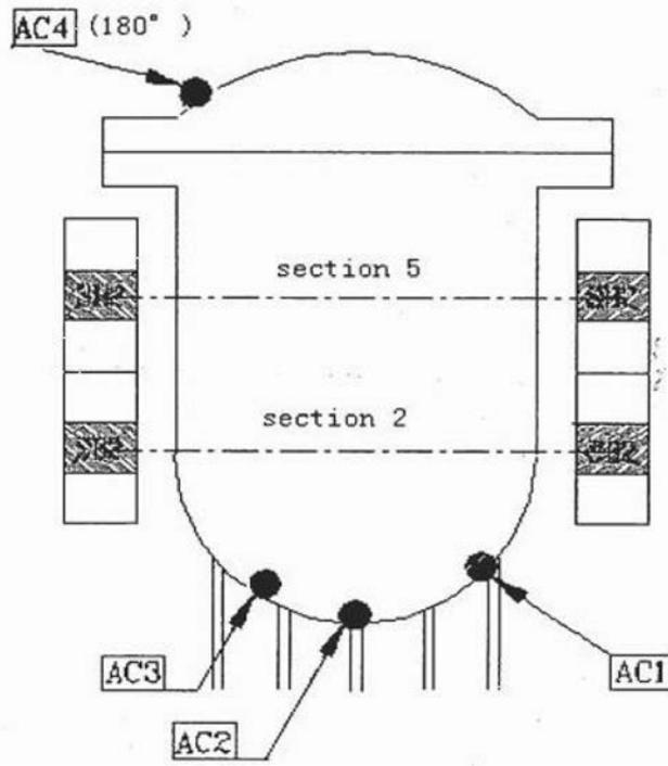
FIG. 38. Accelerometer (AC) locations on the reactor pressure vessel at the Lingao Units 3 and 4 in China.
