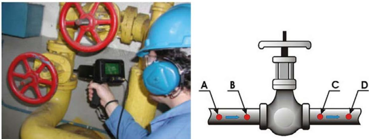
FIG. 42. Ultrasonic measurement (left) and monitoring points relative to a medium stream (right).
