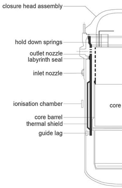
FIG. 23. Reactor vessel internals and ionization chambers.
