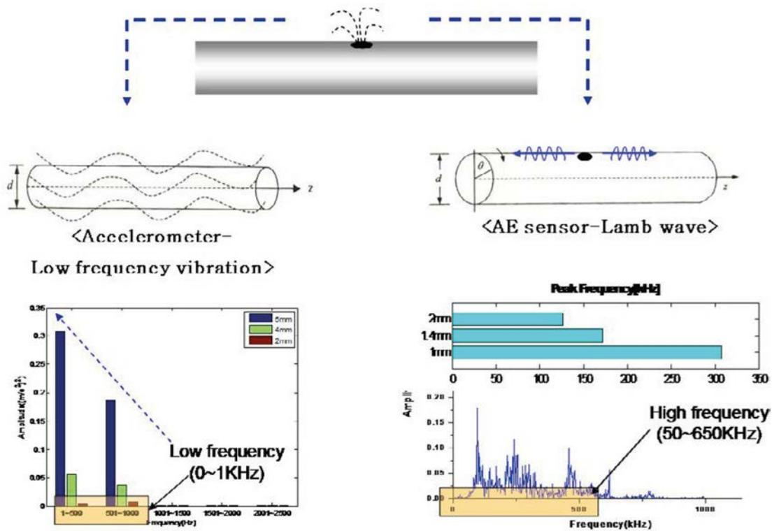
FIG. 41. A new approach for leakage monitoring.
