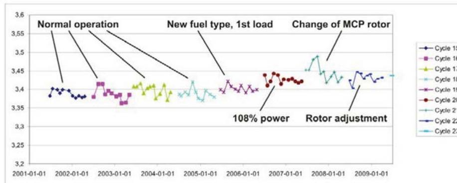
FIG. 25. Average coolant velocity trend for Unit 4 of Paks NPP (during 8 years).
