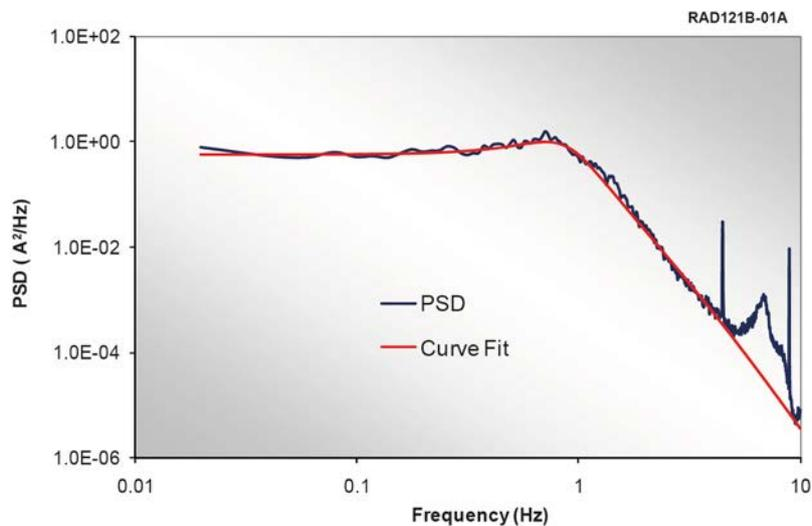
FIG. 68. FFT analysis of response of pressure sensor.
