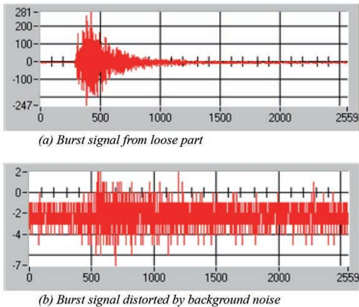
FIG. 30. Burst signals of metal to metal impact (a) as registered by a nearby acoustic sensor (accelerometer), and (b) distorted by background noise.
