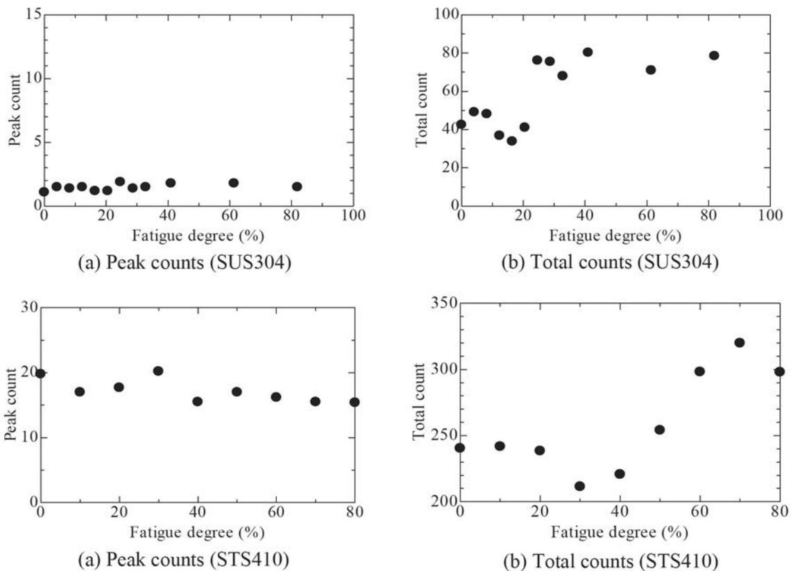
FIG. 58. Magnetic AE at each fatigue phase.
