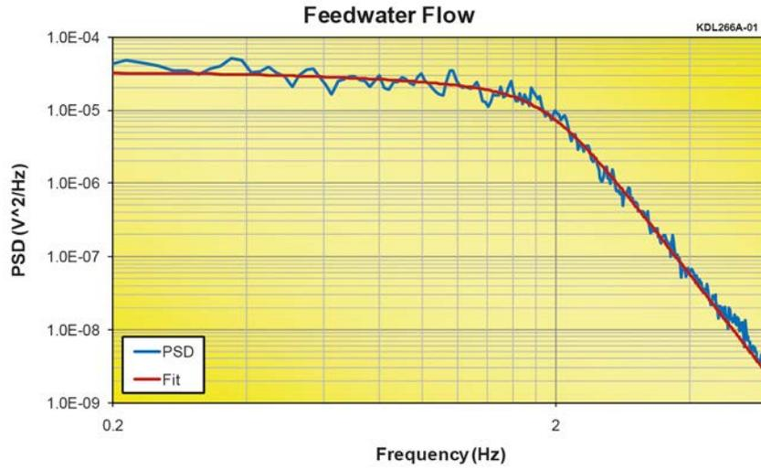
FIG. 16. PSD and fit for feedwater flow transmitter.
