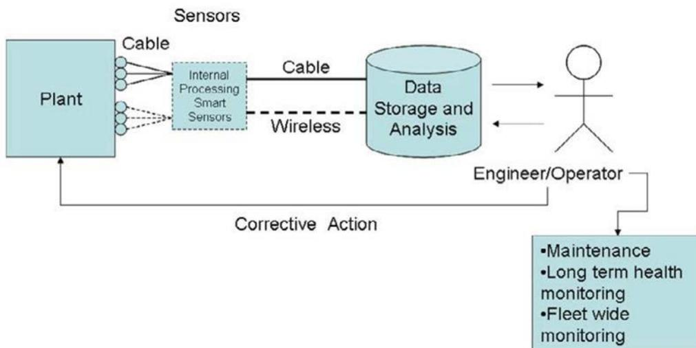
FIG. 66. Overall architecture of an OLM system.
