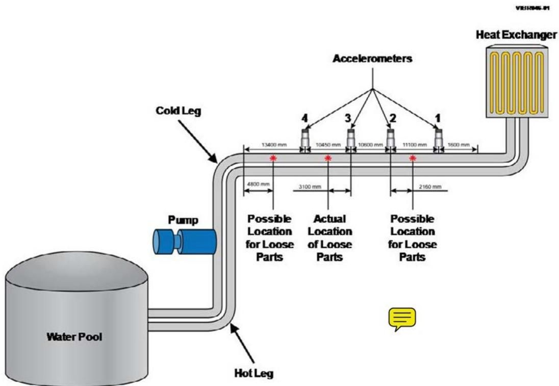
FIG. 45. Schematic of the test loop for loose parts benchmark, showing the placement of sensors and possible loose parts.
