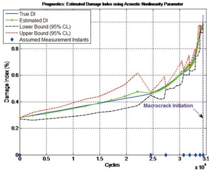
FIG. 64. Prediction of the DI from acoustic non-linearity measurements, to demonstrate the feasibility of the prototype Bayesian algorithm.
