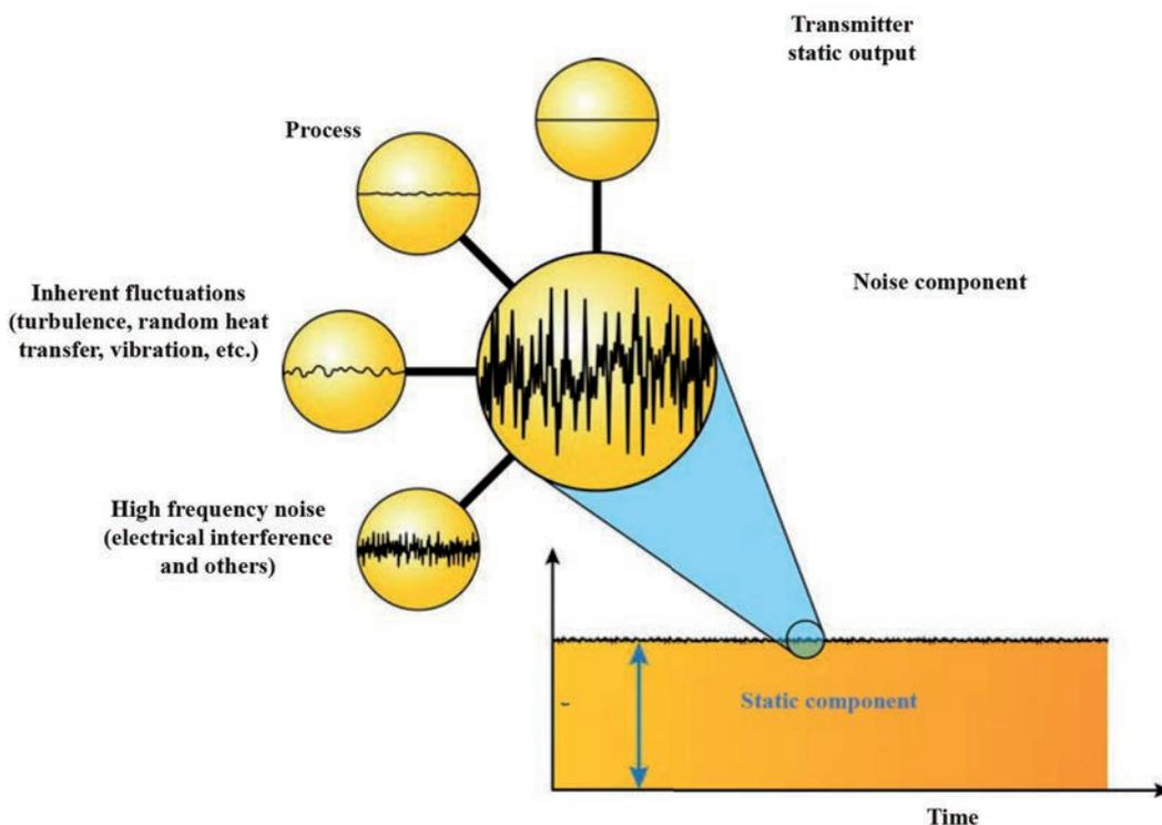
FIG. 2. Static and noise components of a sensor output.
