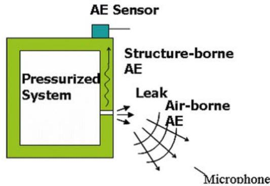
FIG. 31. AE technique for leak detection.
