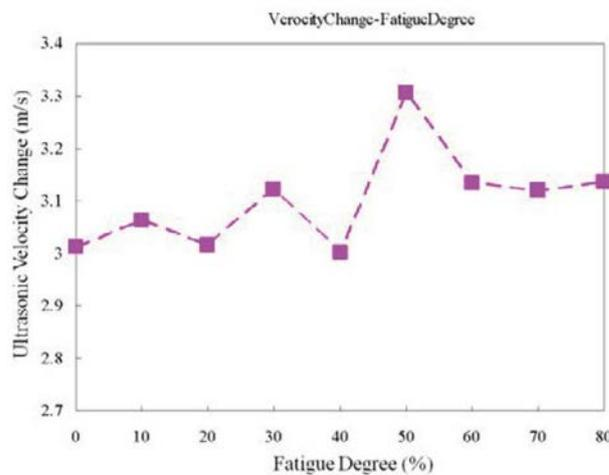
(c) Speed change of transverse wave by magnetization oscillating in parallel direction to magnetic field (STS410)
