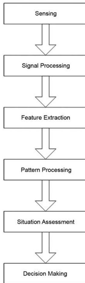
FIG. 79. Waterfall data fusion architecture.
