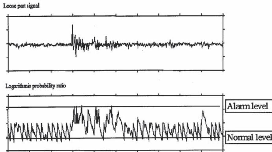
FIG. 34. Event in time signal (upper plot) and its indication by the LLR.
