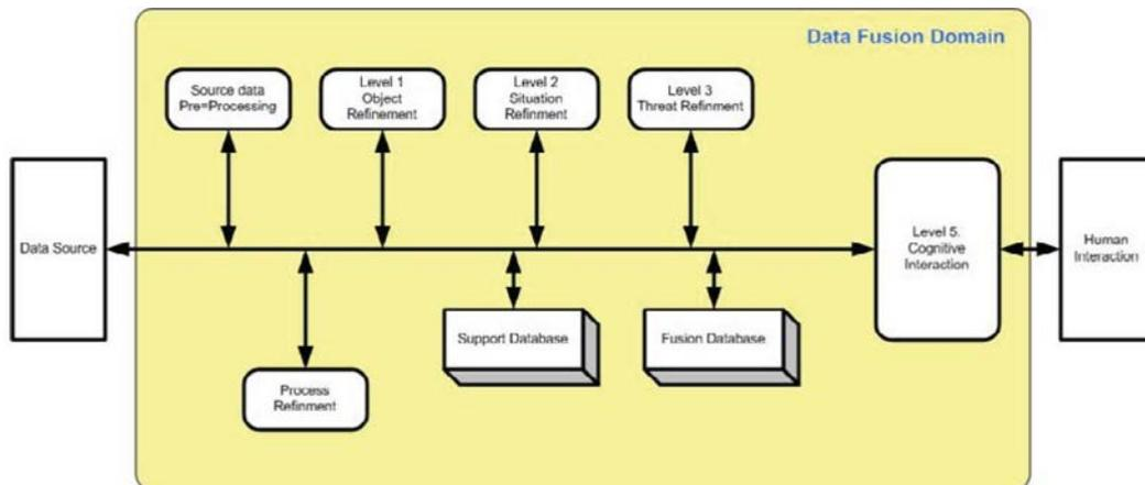
FIG. 78. The JDL data fusion process model.
