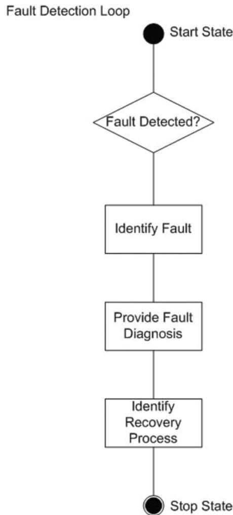
FIG. 67. Activities executed in the fault detection loop.
