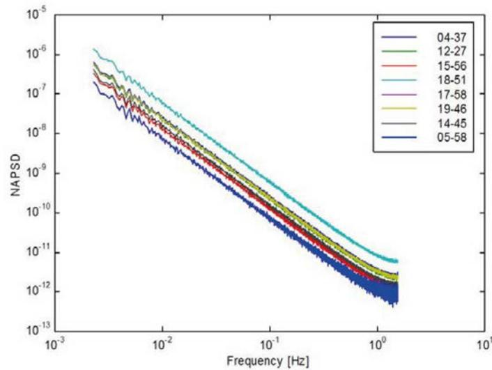
FIG. 26. Normalized APSD functions of some SPND signals from the 7th (highest) level of the chain.
