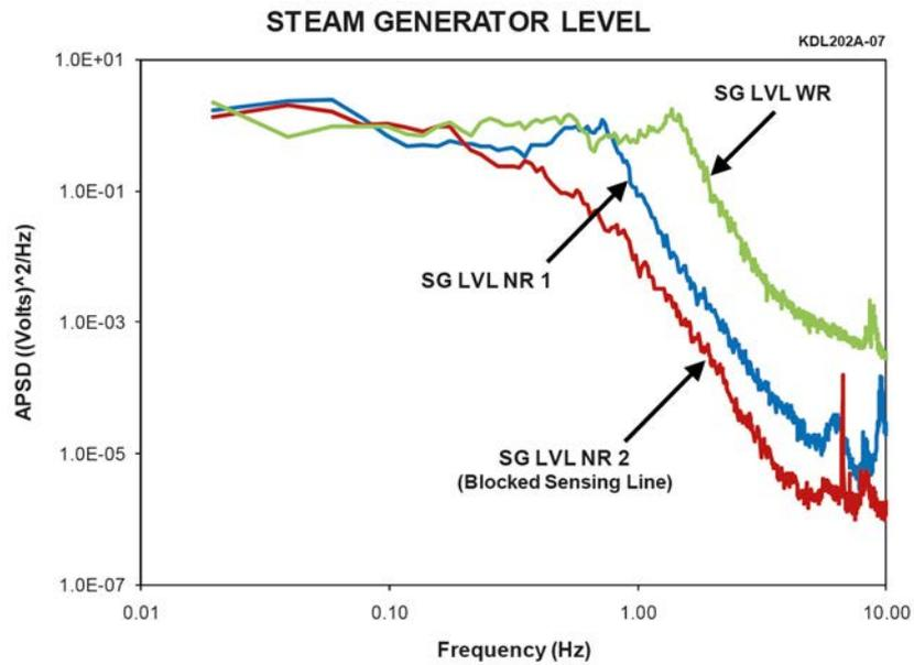
FIG. 17. Comparison of steam generator level (SG LVL) transmitters in the benchmark data.
