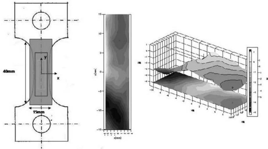
FIG. 59. Electrical potential distribution on PVDF thin film attached onto a specimen with 80% fatigue phase (SUS316NG).
