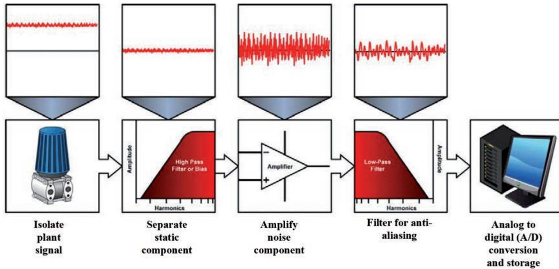
FIG. 4. Noise data acquisition process.
