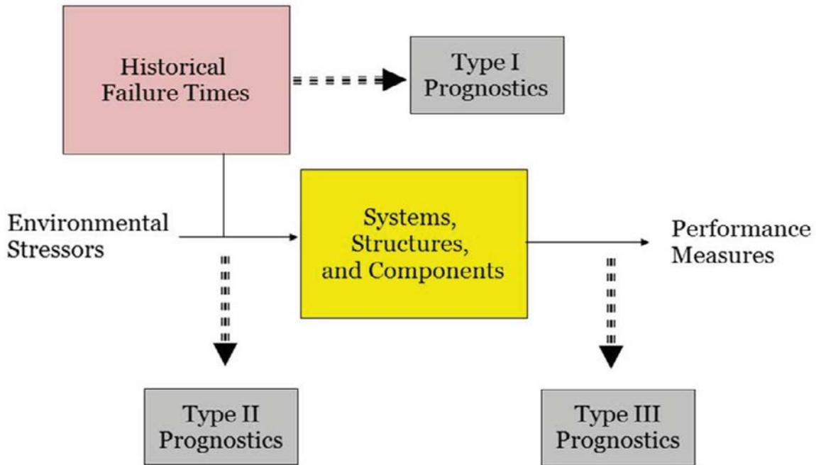
FIG. 53. Prognostic method types.
