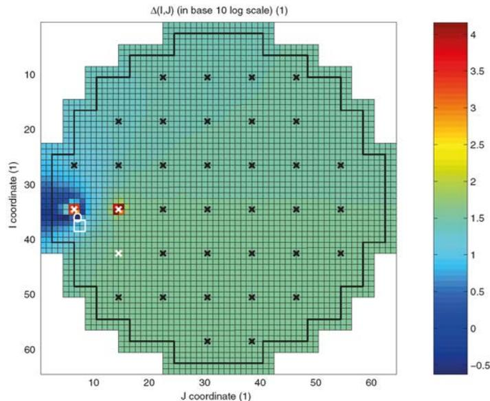
FIG. 28. Result of the localization algorithm in the Forsmark-1 case.
