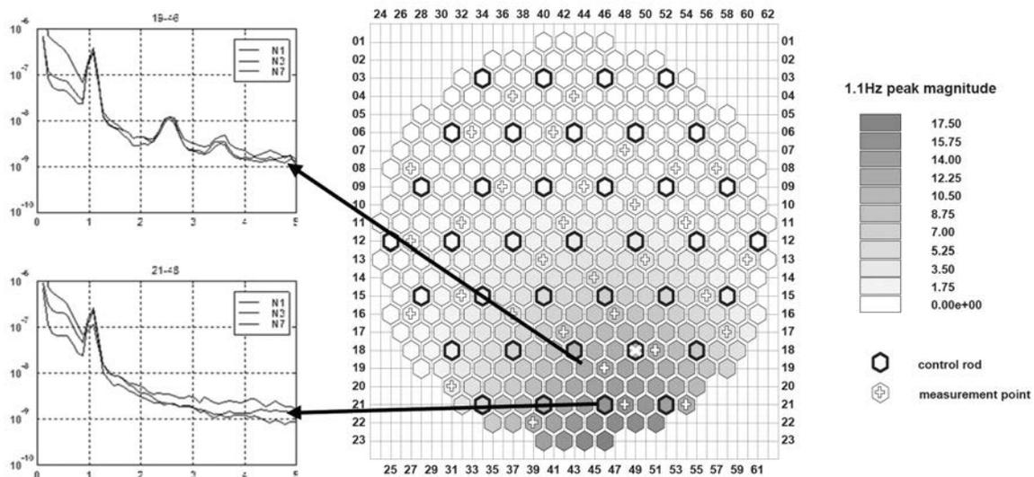
FIG. 22. Noise map of a control rod vibration at 1.1 Hz.
