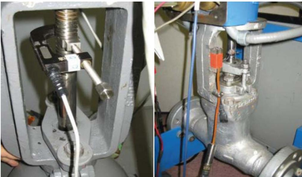
FIG. 44. Ultrasonic measurement of MOV integrity at a Hungarian nuclear plant.
