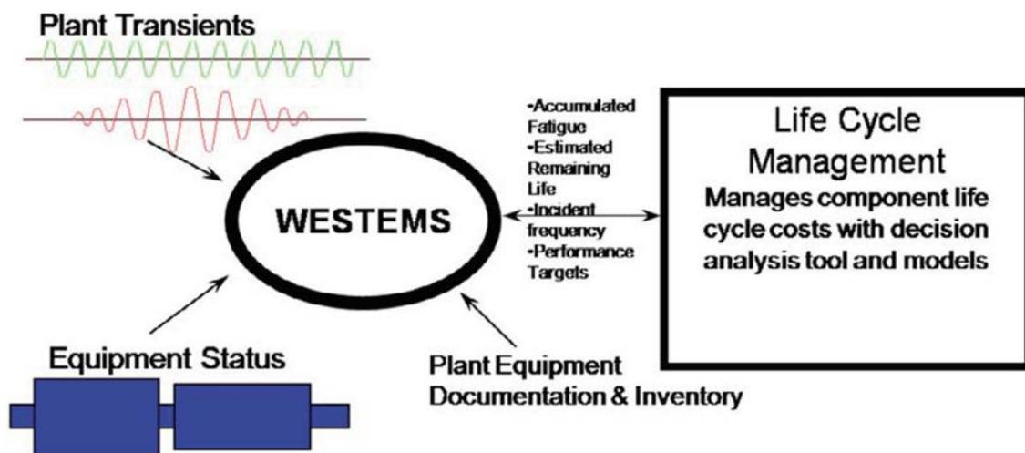
FIG. 73. Typical solution with a WESTEMS monitoring and diagnostic system.
