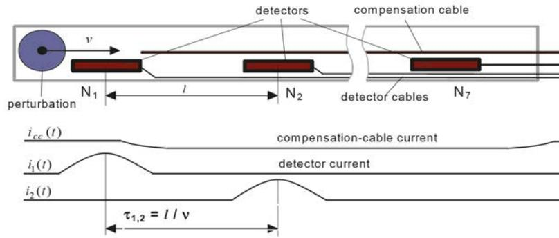
FIG. 6. Transit time ( $\tau_{1,2}$ ) of a propagating perturbation estimated from SPND time signals.
