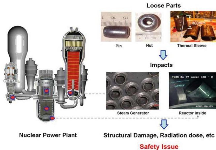
FIG. 29. Primary system pressure boundaries of a PWR and examples of loose parts.
