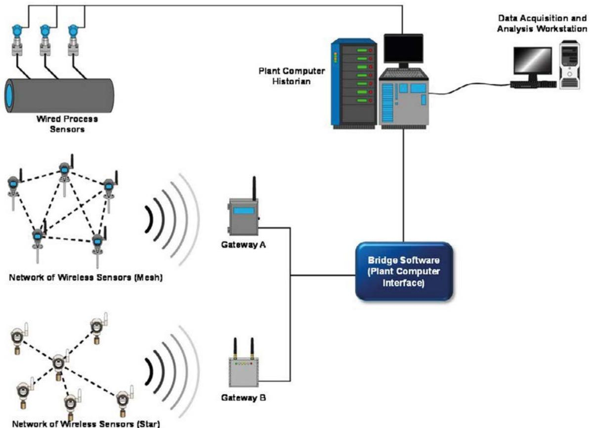
FIG. 77. Wireless sensors in a plant network.
