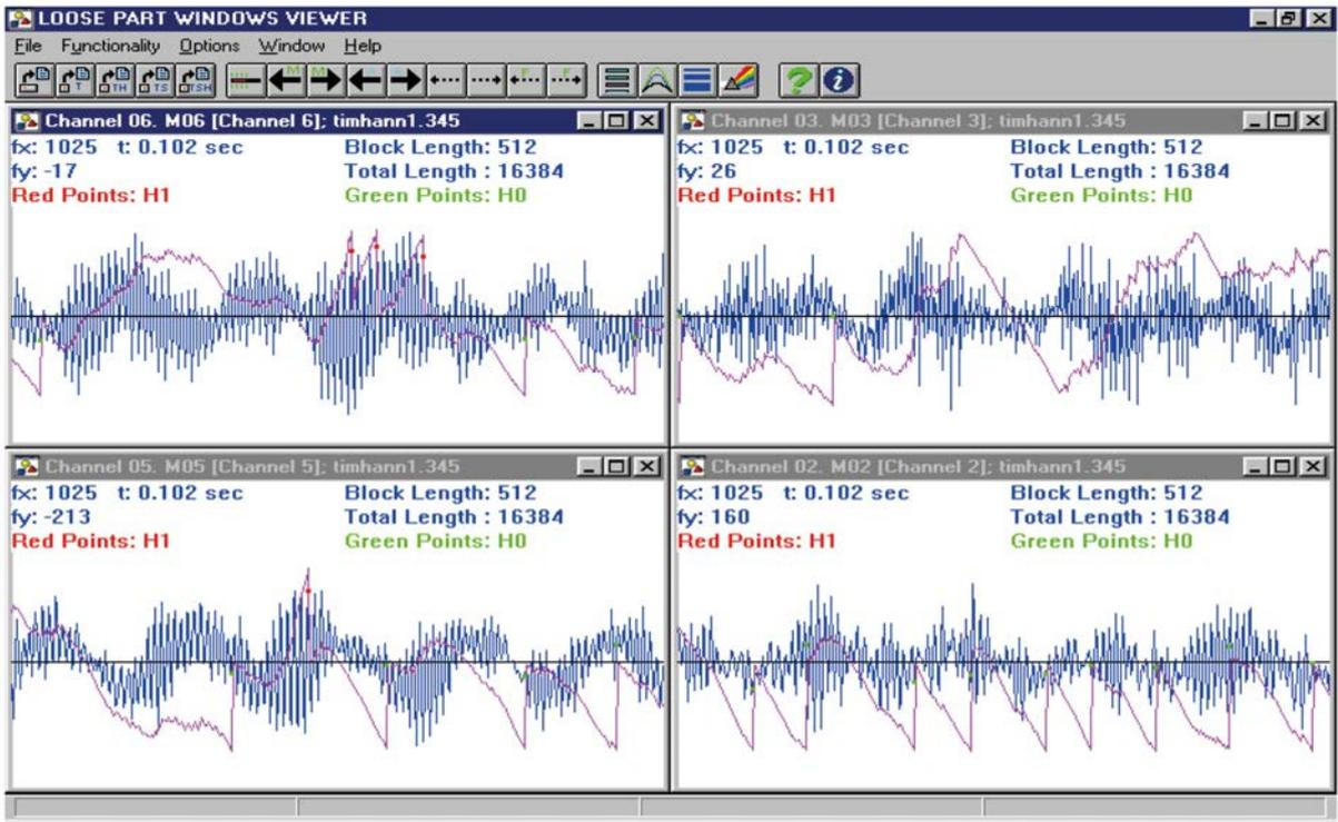
FIG. 35. Time signals indicating loose parts and the LLR functions.
