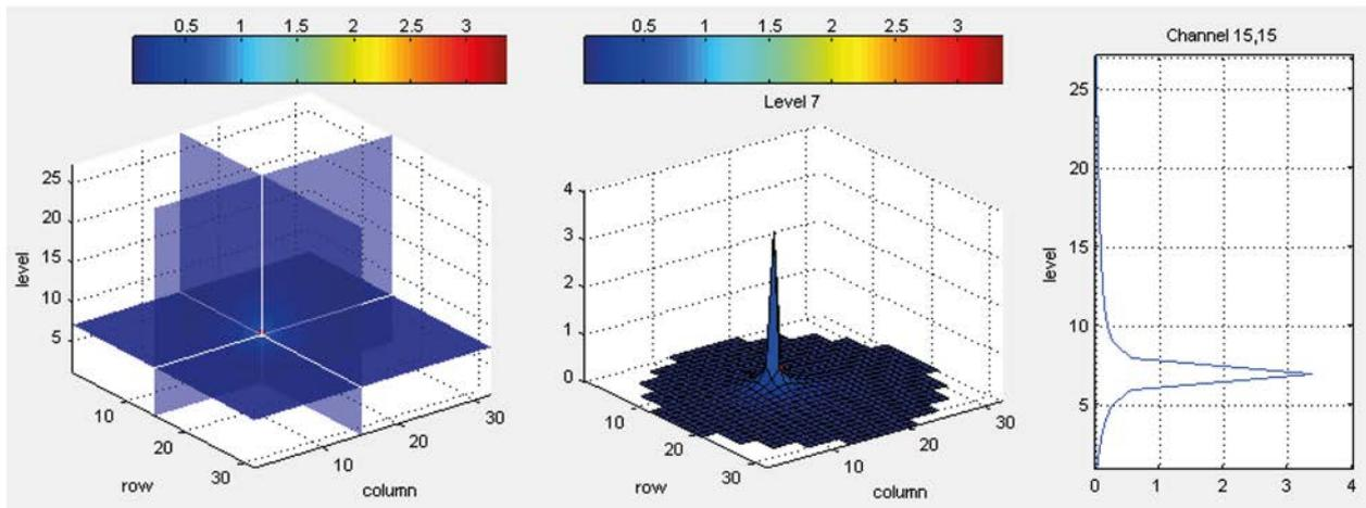
FIG. 19. Spatial distribution of the calculated magnitude of the thermal neutron noise.
