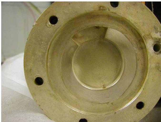
*FIG. 3.4. Keyhole water target design. The material of construction of this target was silver.*
