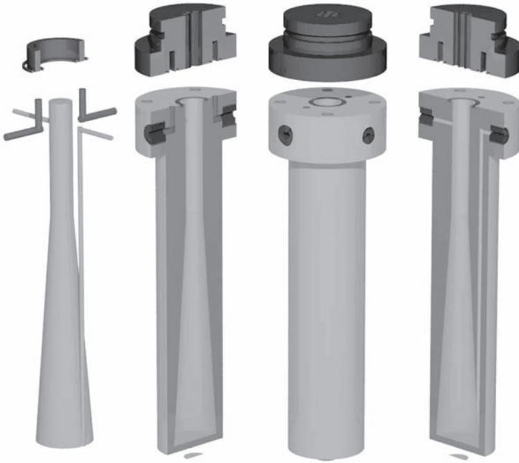
FIG. 5.10. Conical design for  $^{11}\text{C}$  gas target.
