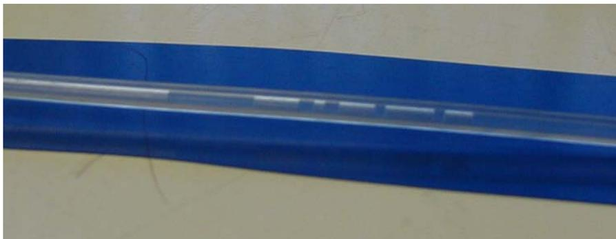
FIG. 4.7. Picture of the water broken up into several sections in the plastic tubing.
