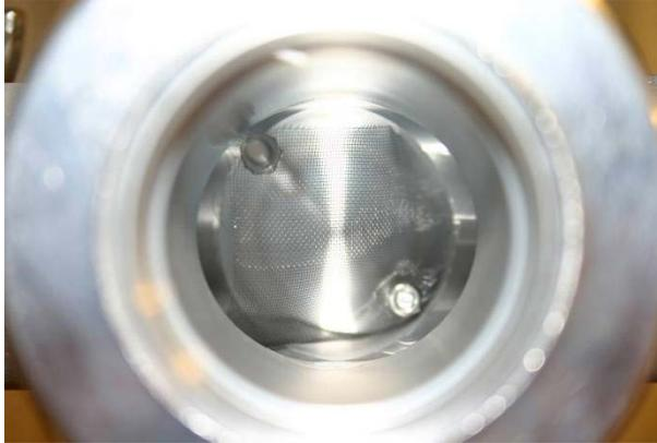
FIG. 2.2. Fine wire mesh used to determine the beam profile.
