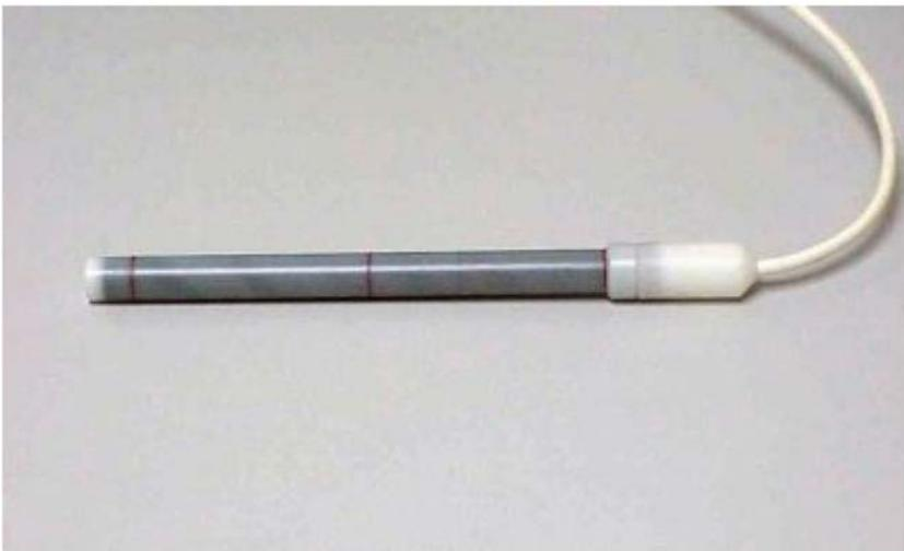
FIG. 39. Pencil ionization chamber used for dosimetry of CT examinations. The active volume of the chamber is typically  $3 \text{ cm}^3$  and the active length is  $100 \text{ mm}$  [26].
