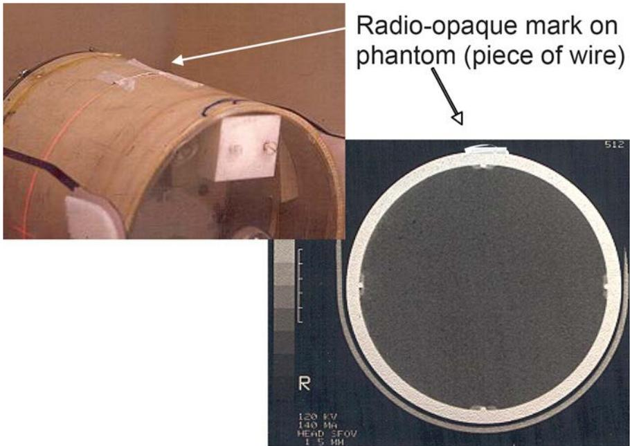
FIG. 20. Light alignment with scan plane: Imaging method.
