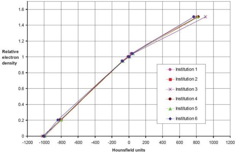
FIG. 30. CT calibration curves measured with the CIRS phantom at different hospitals [67].
