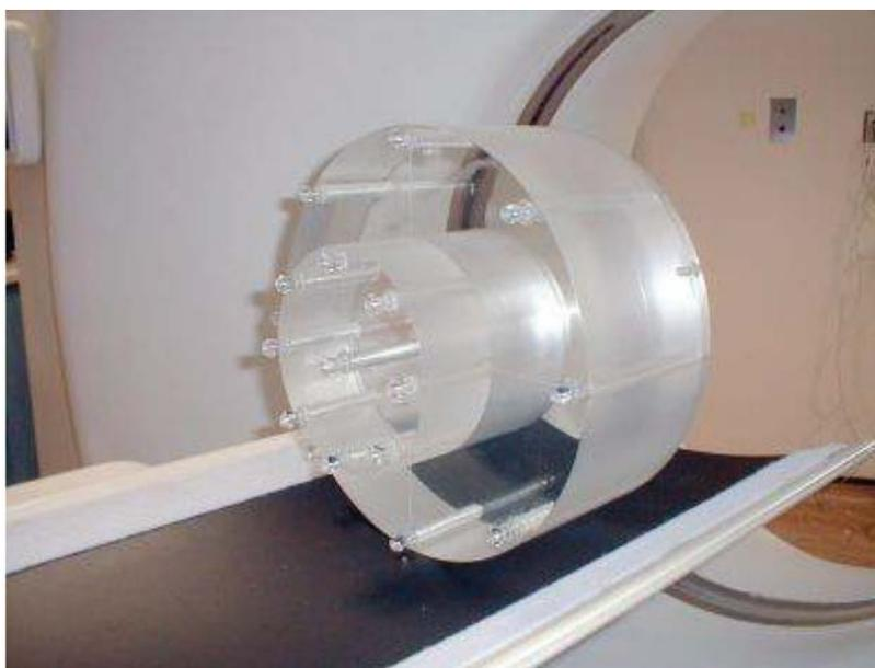
FIG. 37. Photograph of typical standard head and body CT dosimetry phantoms. The head phantom is the innermost cylinder (which has been partially removed for clarity) and when surrounded by a PMMA annulus, the body phantom is formed (from Ref. [26]).
