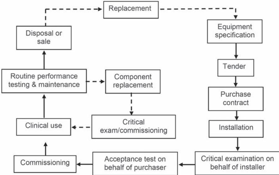
FIG. 17. Life cycle of a piece of equipment.
