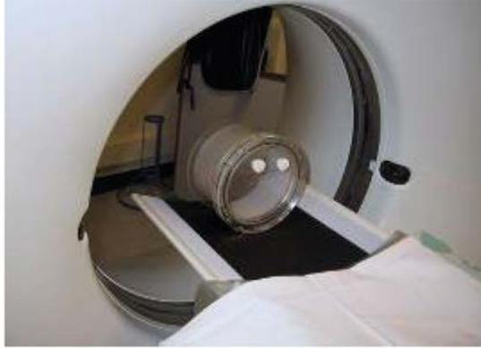
*FIG. 21. A non-commercial head phantom with simulated bone exterior.*
