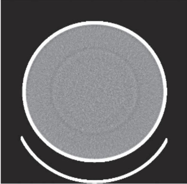
*FIG. 11. Example of ring artefacts in a water filled phantom.*
