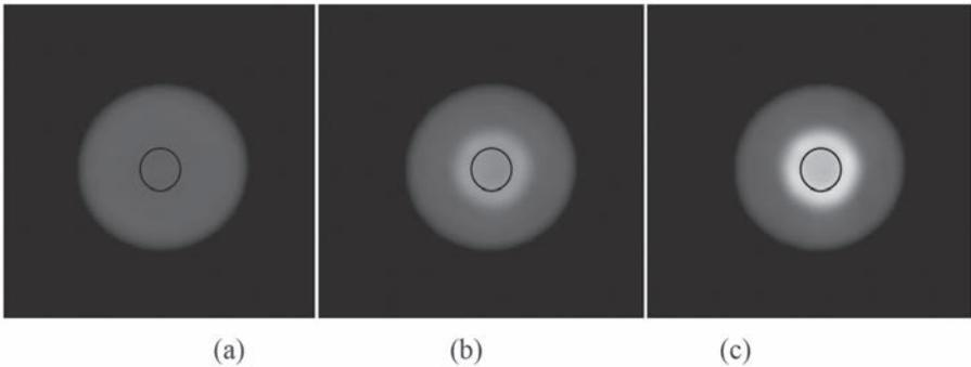
*FIG. 26. Images of test object with ROIs shown drawn over metal ‘delta function’ insert. Insert is (a) not in the tomographic plane, (b) partially in the tomographic plane and (c) centred in the tomographic plane.*
