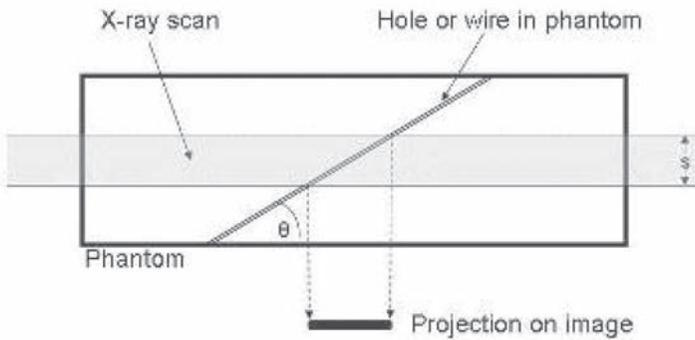
FIG. 34. View of slice width phantom with superimposed CT slice projection and resulting test object projection on image.
