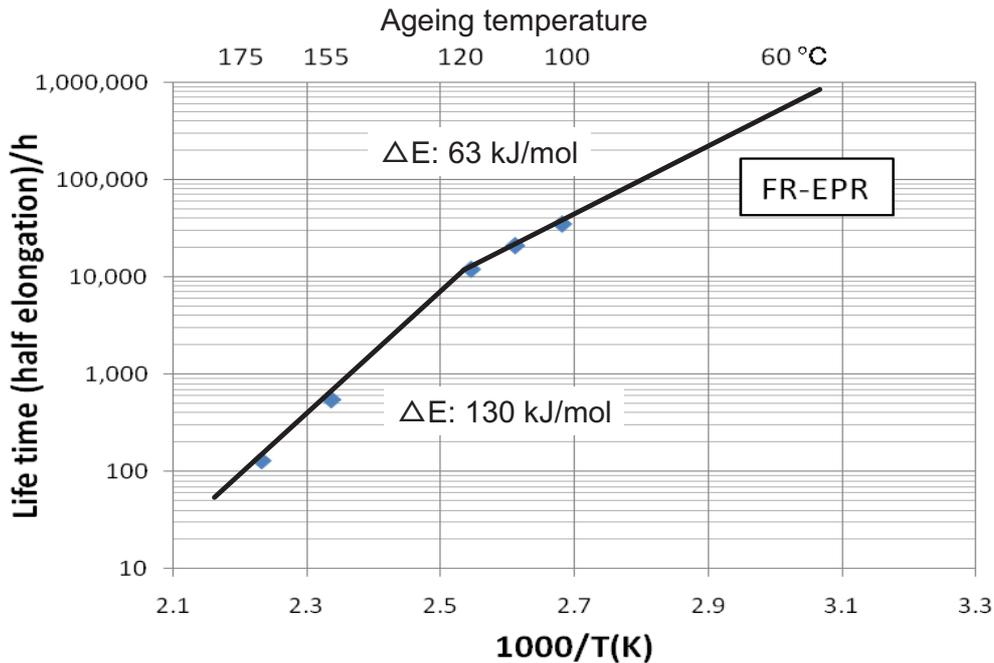
FIG. A-3. Arrhenius plot for an EPR cable material [9].
