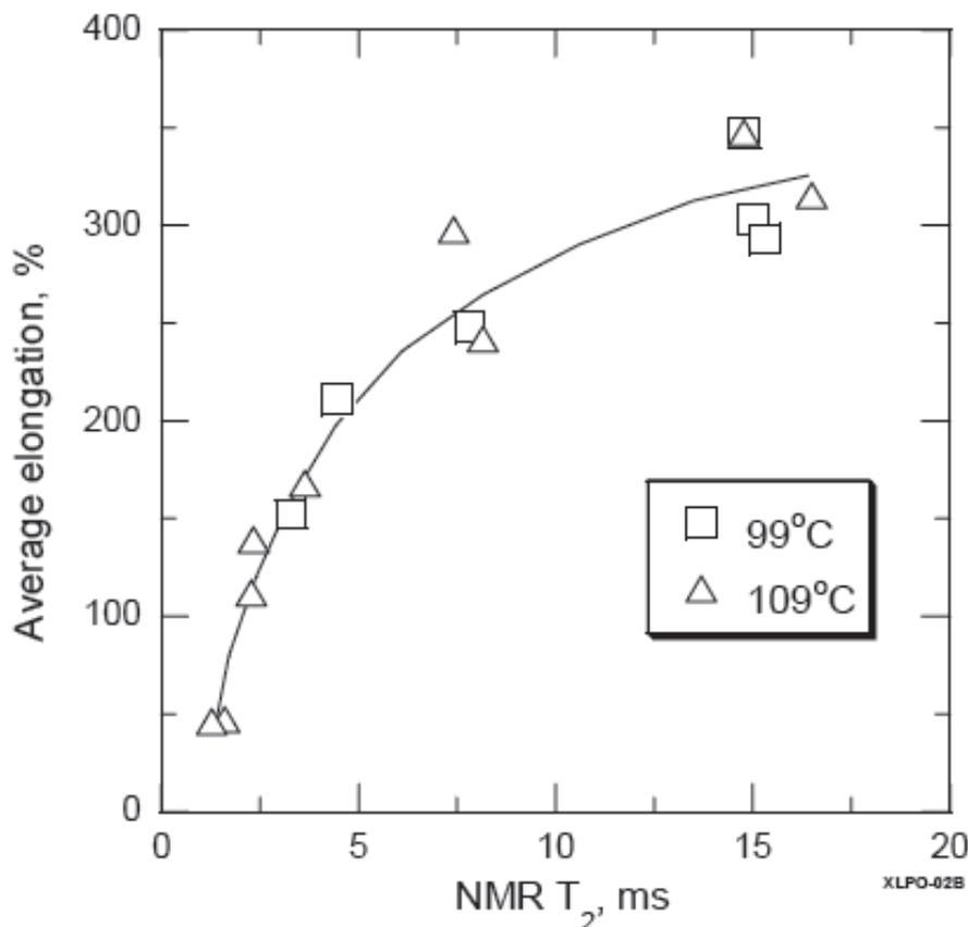
FIG. 4.7. Correlation of NMR relaxation time,  $T_2$  to elongation at break data for a thermally aged, polyethylene based insulation.
