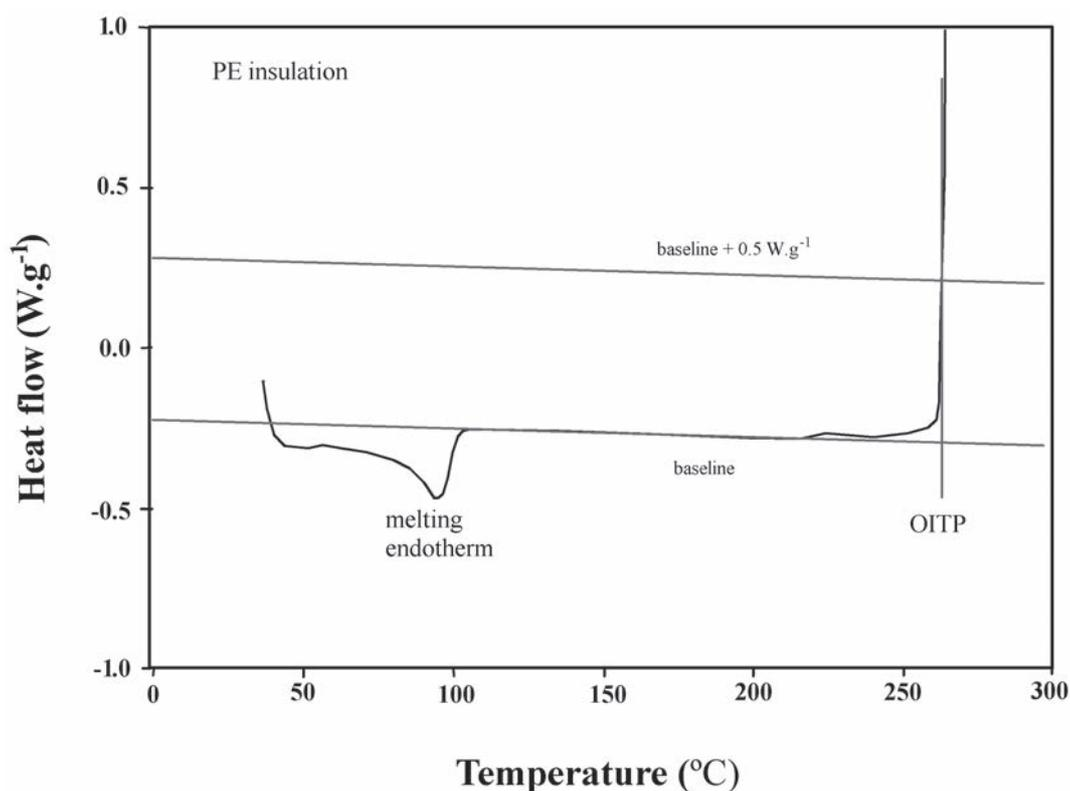
FIG. 4.3. A typical DSC trace for a thermoplastic polymer indicating measuring point for OITP.
