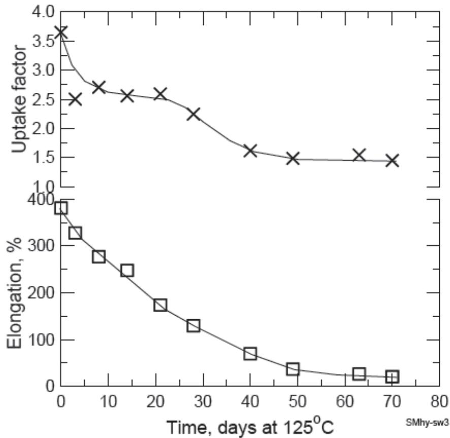
FIG. 4.5. Example plots of the solvent uptake factor and elongation at break against ageing time for a CSPE material.
