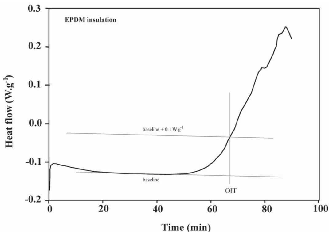
FIG. 4.2. A typical OIT plot showing a threshold measurement at 0.1 W/g.
