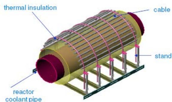
FIG. 6.1. The stand for deposit of reference specimen in the plant containment [38].
