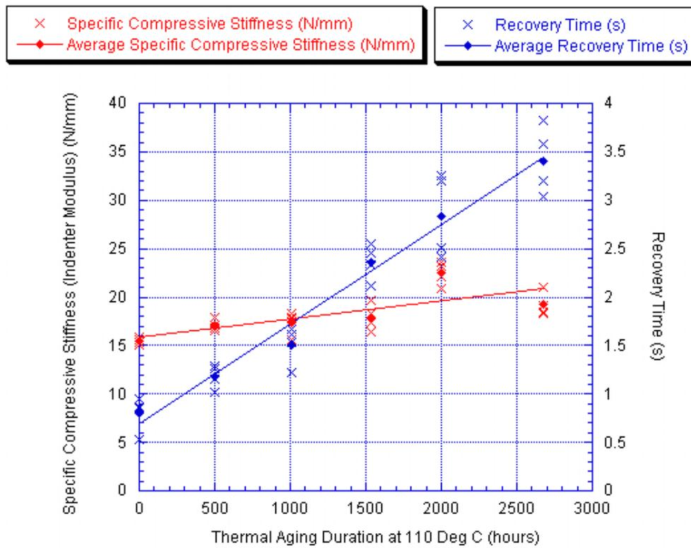
FIG. 4.11. Recovery time and indenter modulus for EPR insulation.
