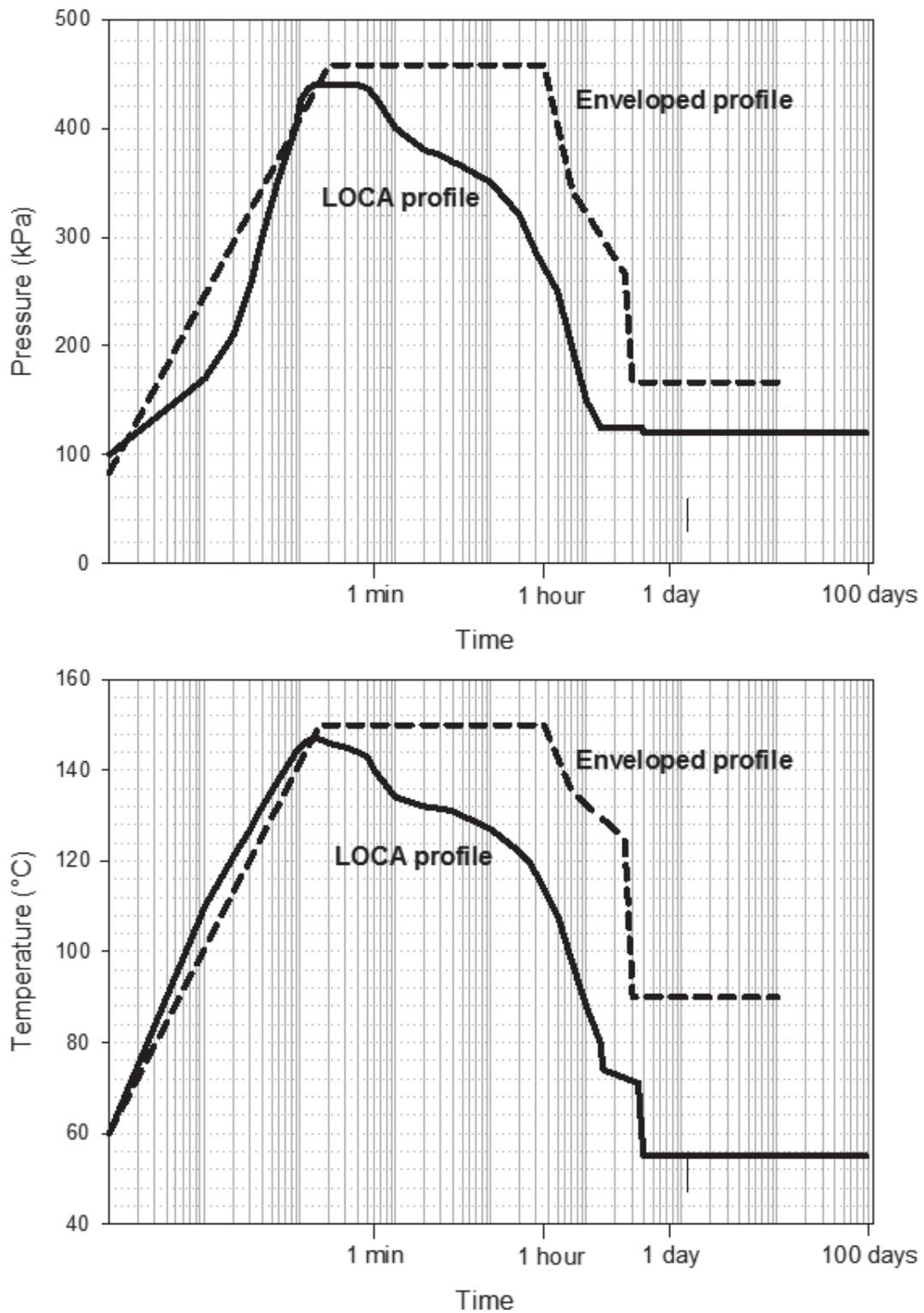
FIG. 3.3. Typical pressure and temperature LOCA profile used for a PWR (WWER-1000) reactor.
