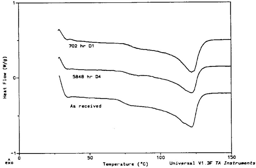
FIG. A-6. DSC traces for a XLPE insulation material showing the crystalline melting endotherm in both unaged and aged material.
