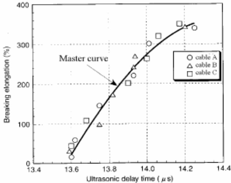
FIG. 4.14. Comparison of the correlation data for various cables from different manufacturers to the master curve for PVC.
