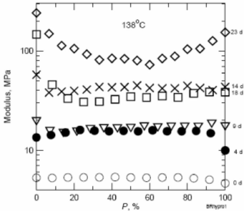
FIG. A-1. Modulus profiling of a CSPE material aged at 138°C where P is the thickness of the sample (1.6 mm) [26].
