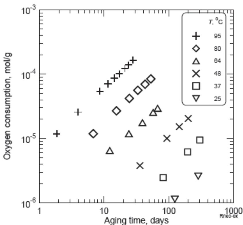
FIG. 4.6. Plots of oxidation consumption against ageing time for a thermally aged PCP sample.
