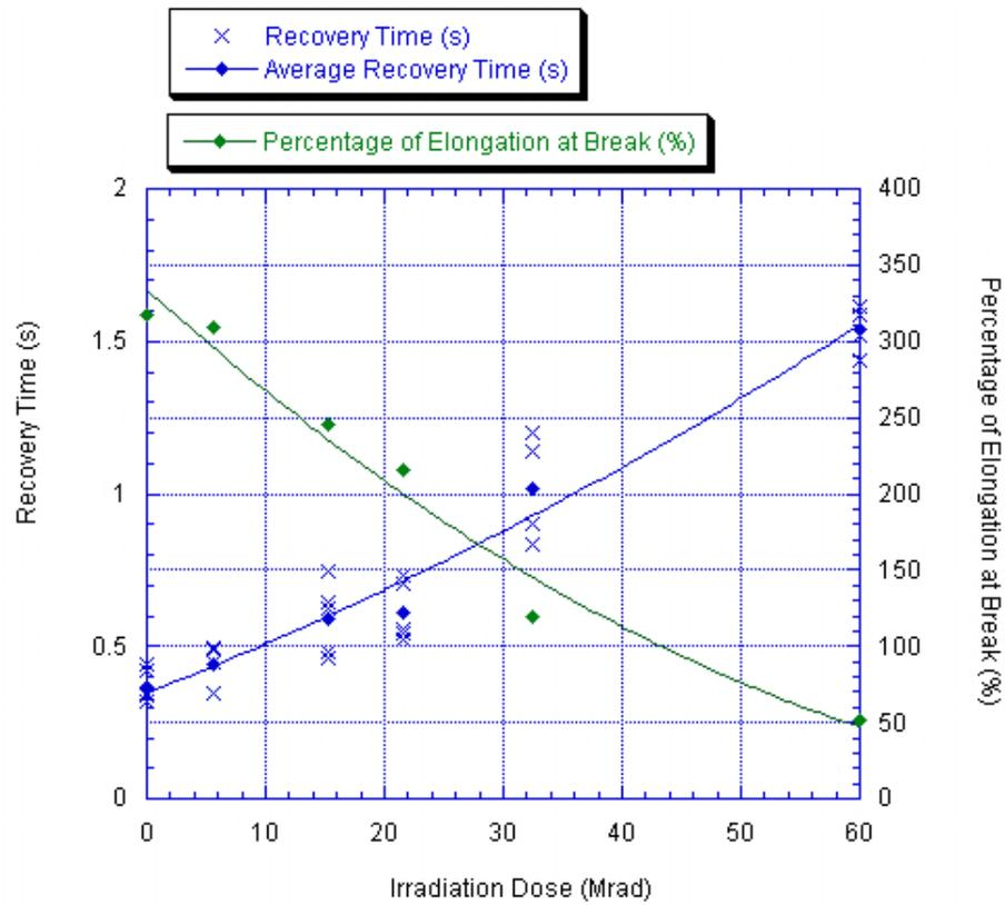
FIG. 4.10. Elongation and recovery time for an irradiated PVC jacket.
