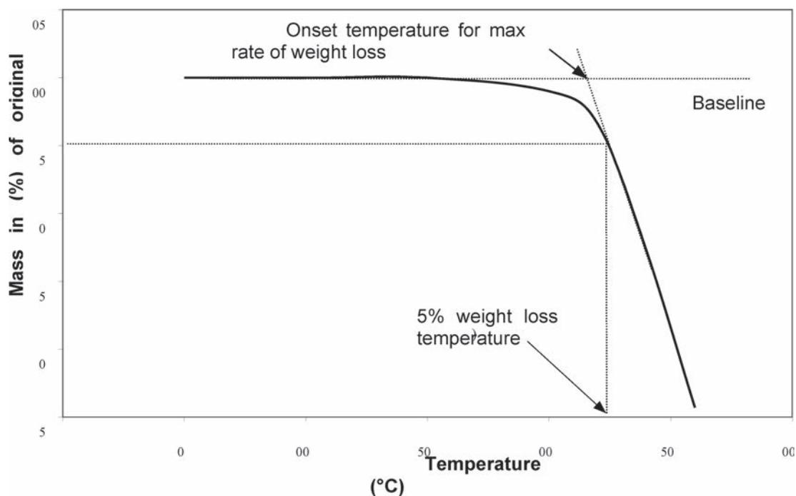
FIG. 4.4. A typical TGA trace showing 5% weight loss temperature and maximum weight loss temperature.
