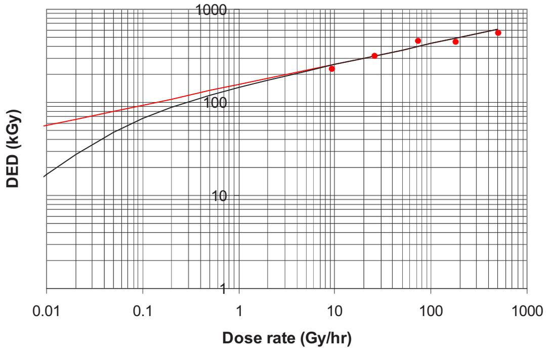
FIG. A-8. An illustration of how the degradation curve for this XLPE might behave at lower dose rates (black line) compared to the power law model (red line).
