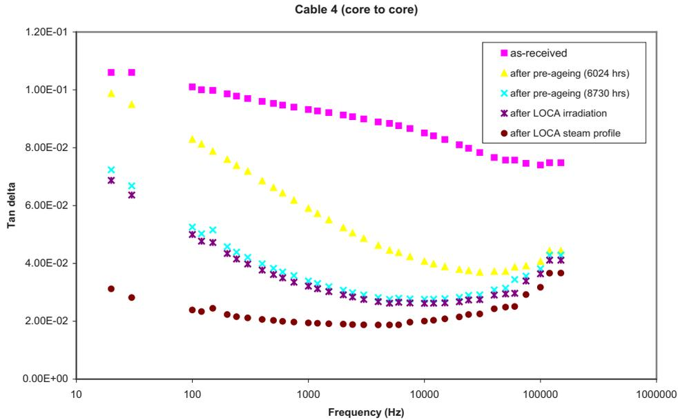
FIG. 4.22. Example plot of  $\tan \delta$  against frequency for an aged EVA insulation.
