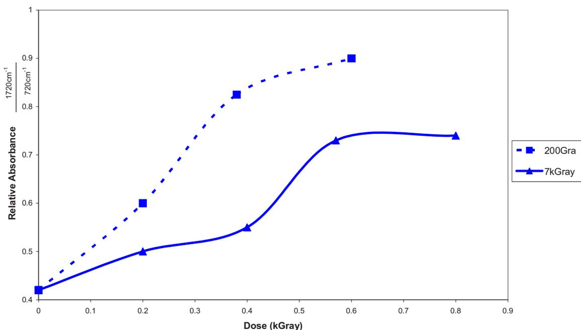
FIG. 4.8. Infrared analysis of a polyethylene material comparing the ratio of absorbance at  $1720$  and  $720\text{ cm}^{-1}$  for unaged and irradiated samples.
