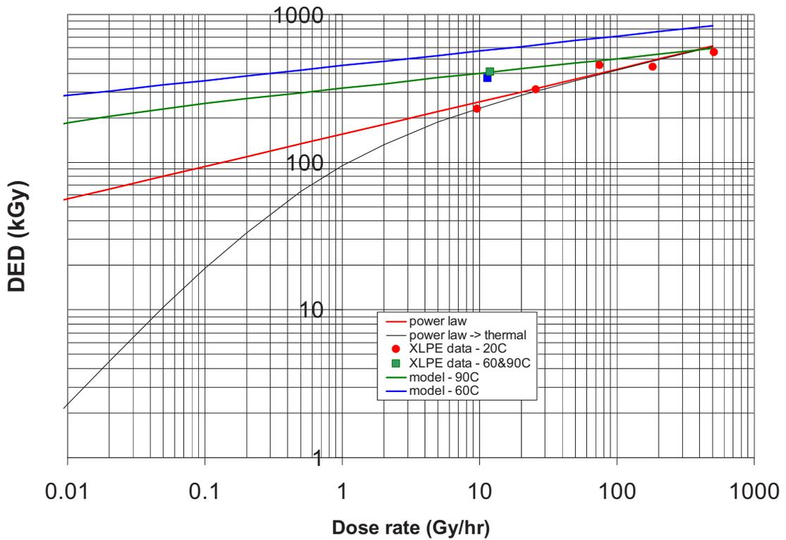
FIG. A-7. Radiation ageing data for an XLPE insulation material as a function of the dose rate.
