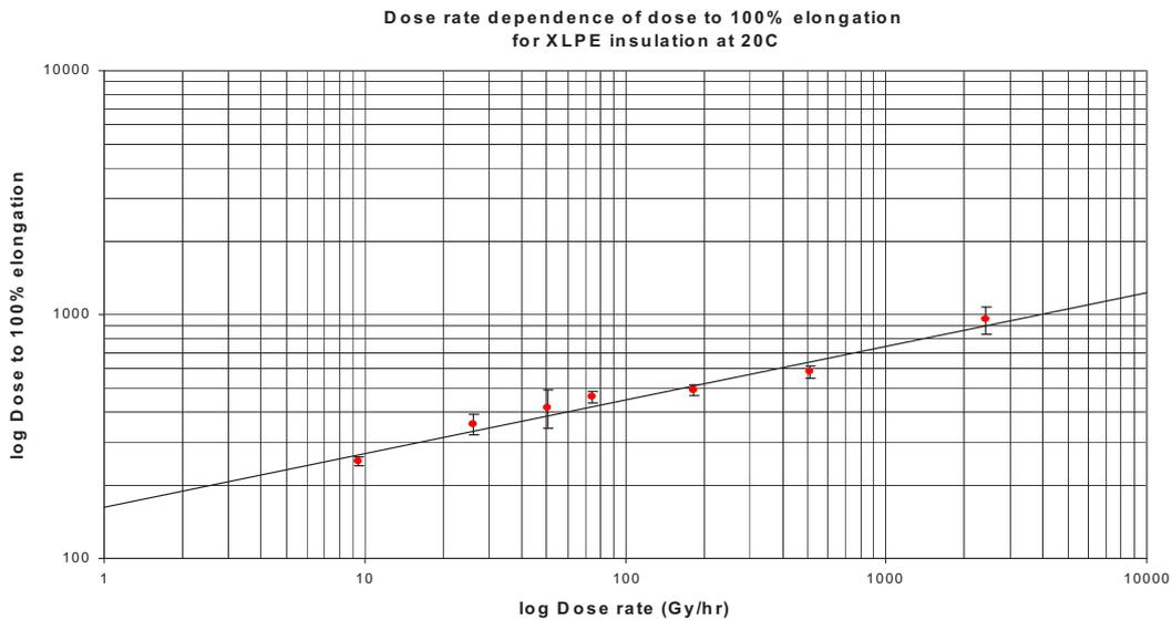
FIG. A-2. Dose required to reach an elongation at break value of 100% absolute as a function of dose rate for an XLPE cable insulation material irradiated at 20°C.
