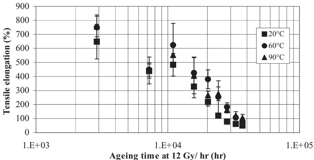
FIG. A-5. Tensile elongation data for XLPE insulation as a function of ageing time at 12 Gy/h.
