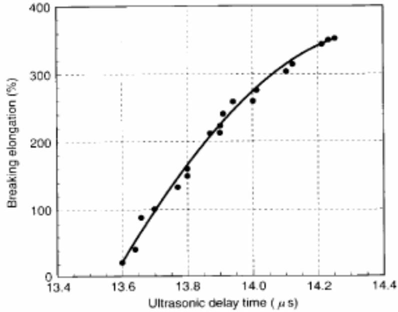
FIG. 4.13. An example of the correlation between the propagation time of ultrasonic waves and elongation at break for a PVC sheath material.
