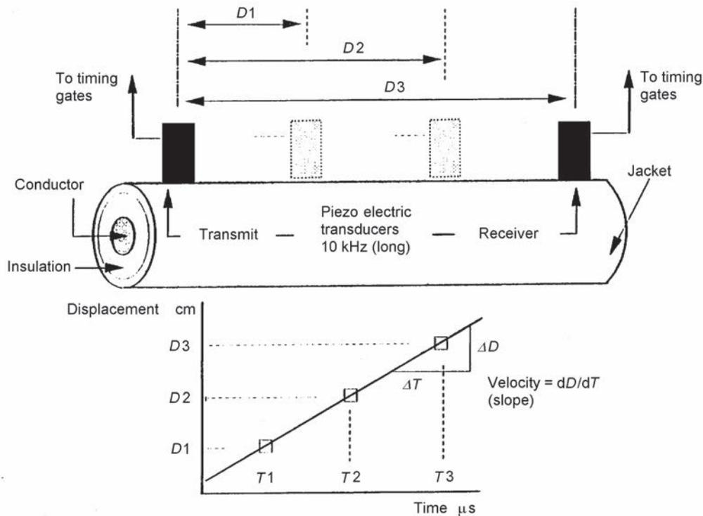
FIG. 4.12. Schematic diagram of sonic velocity test apparatus.
