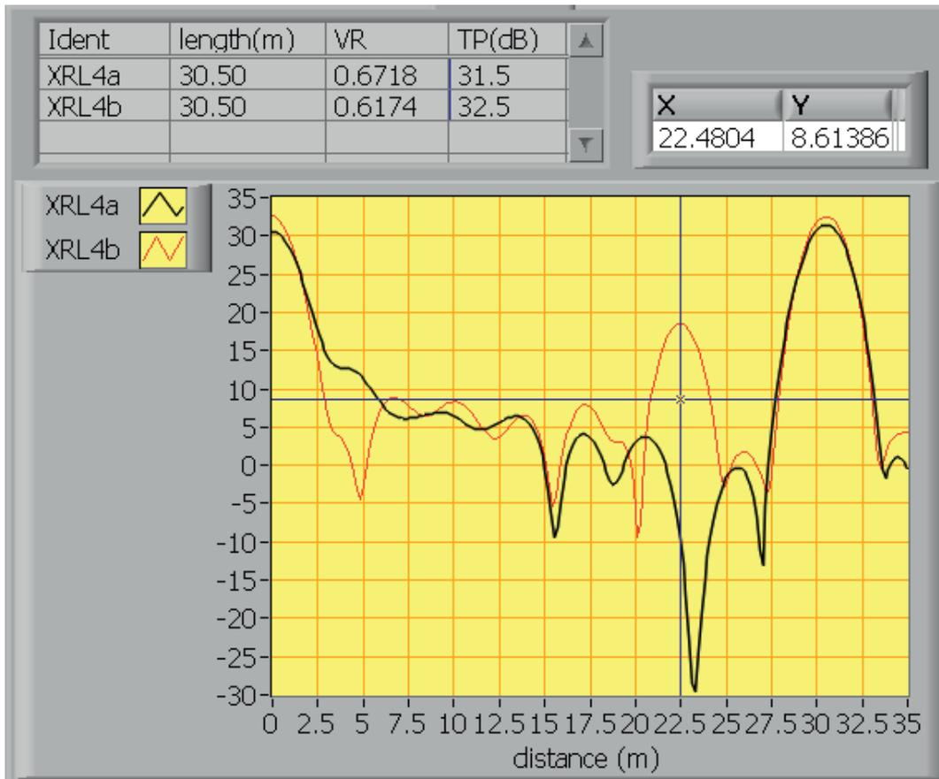
FIG. 4.18. FDR measurement using LIRA on XLPE before (black line) and after (red line) local thermal ageing at 22.5 m.
