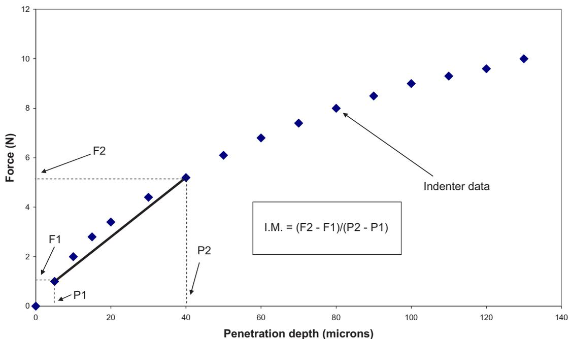
FIG. 4.9. A schematic plot of force against penetration depth, typical of an indenter instrument.
