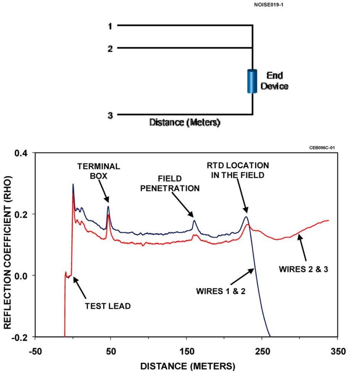
FIG. 4.19. A typical TDR trace involving three wires connected.
