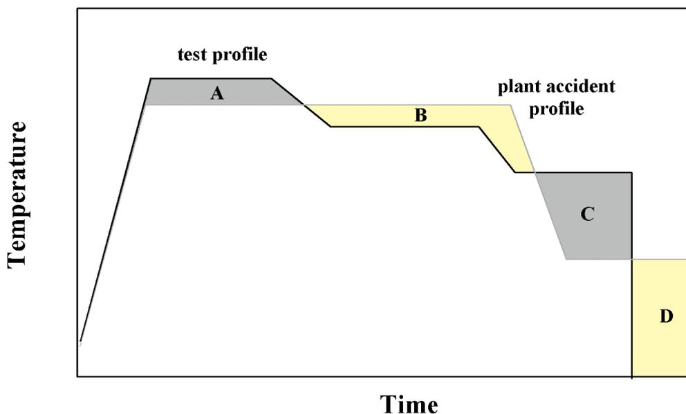
FIG. A-12. Schematic diagram indicating how analysis of DBA test profiles is used.
