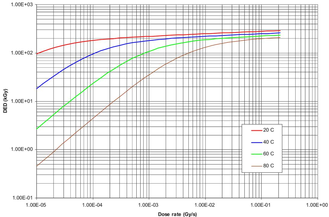
FIG. A-4. Generic plot of the dose required to reach a specific level of degradation (DED) as a function of dose rate at different temperatures for a typical polymeric cable material.
