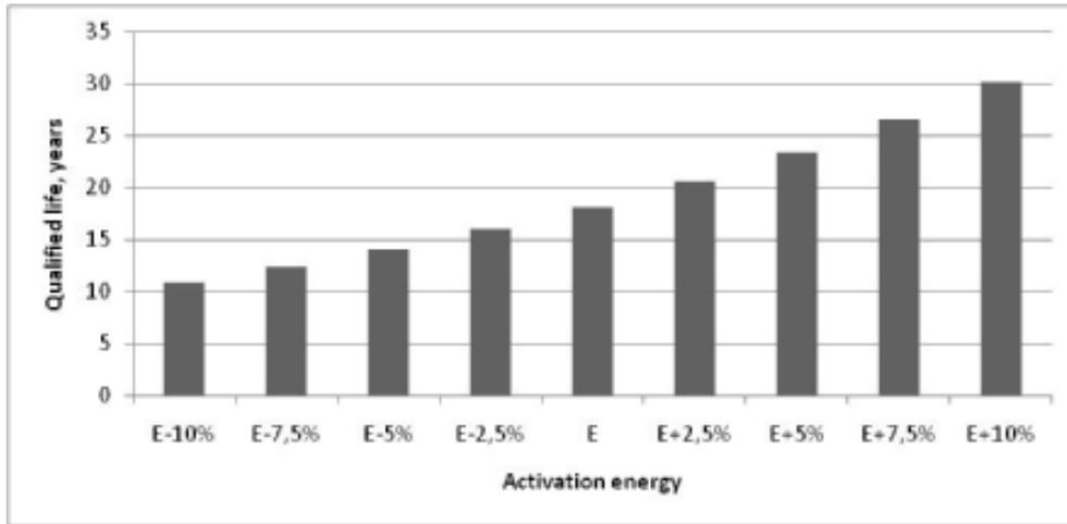
FIG. 5.1. Example of the influence of changes in the assumed value of activation energy  $E$  on qualified life determined from artificial thermal ageing at  $110^{\circ}\text{C}$  extrapolated to a normal service temperature of  $50^{\circ}\text{C}$ .
