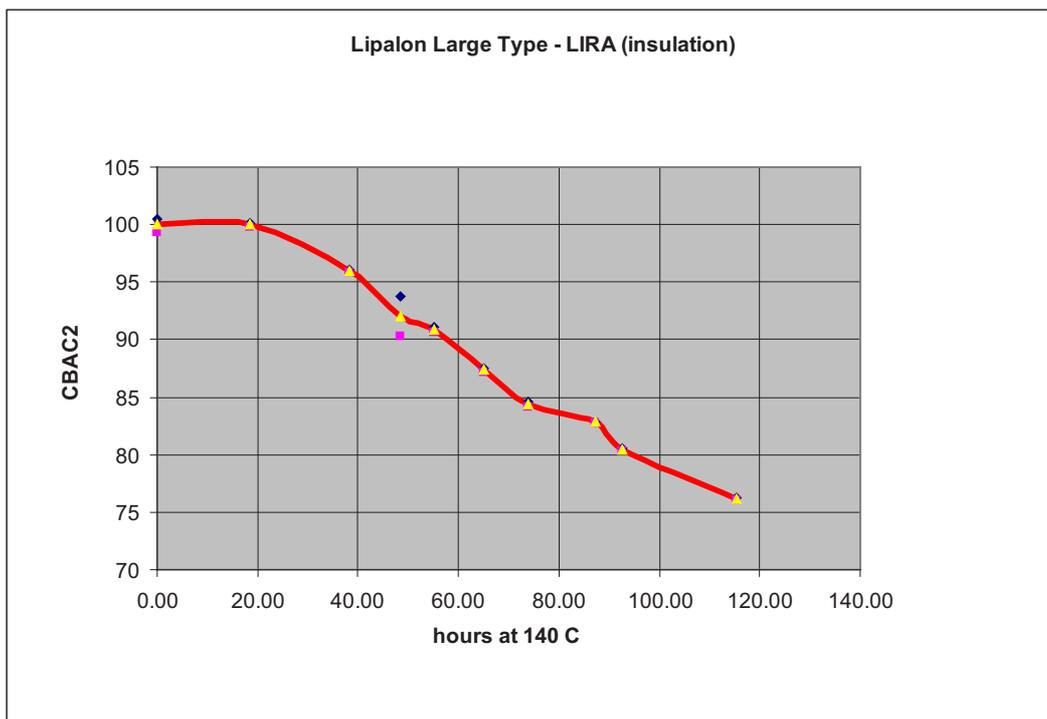
FIG. 4.17. LIRA ageing indicator (CBAC2) versus ageing time, EPDM insulation, low voltage cable.
