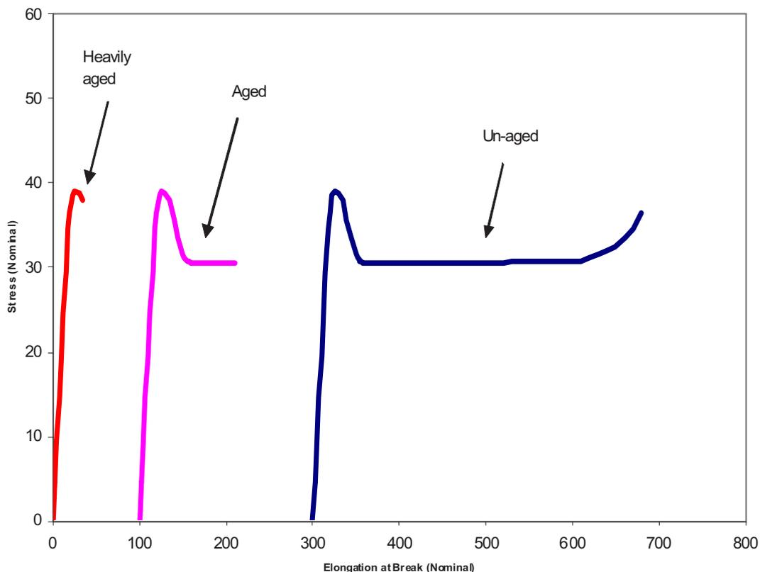
FIG. 4.1. A typical set of degradation curves for a thermoplastic material.
