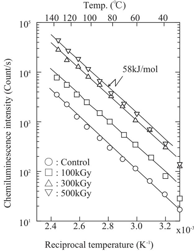
FIG. A-11. Chemiluminescence intensity as a function of measuring temperature for EPR unirradiated and irradiated to 500 kGy.
