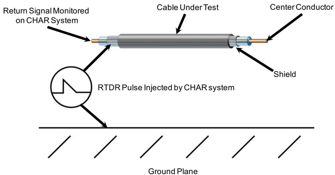
FIG. 4.21. RTDR set-up.
