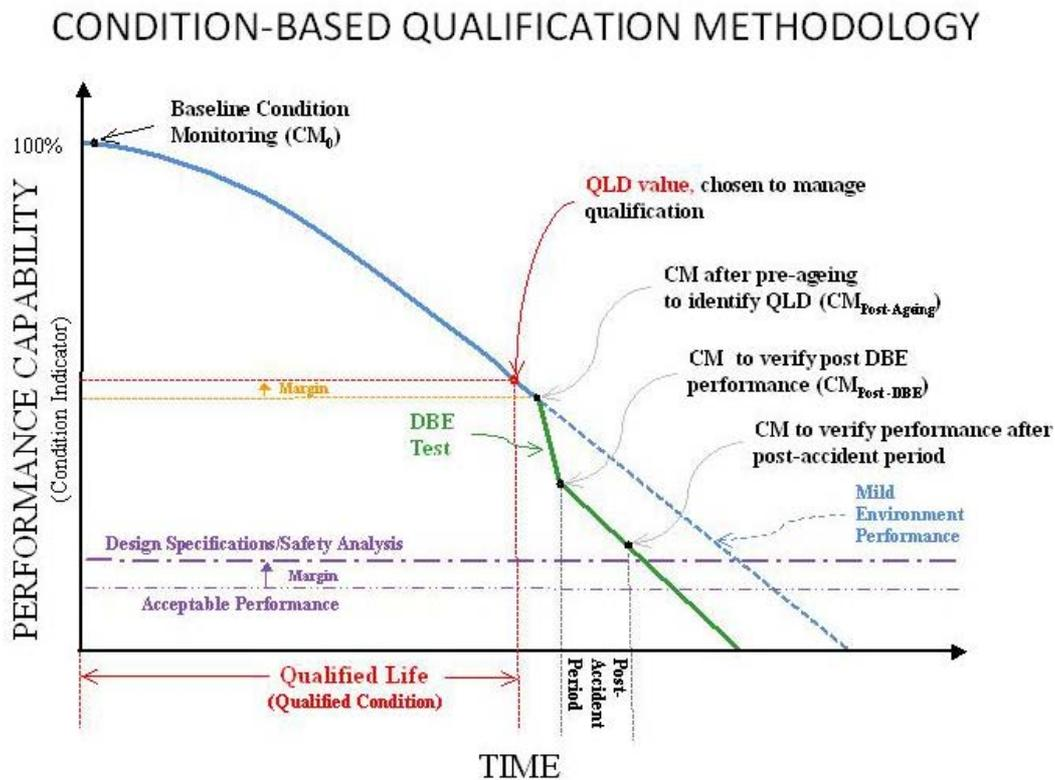
FIG. 3.1. Condition based-qualification methodology.
