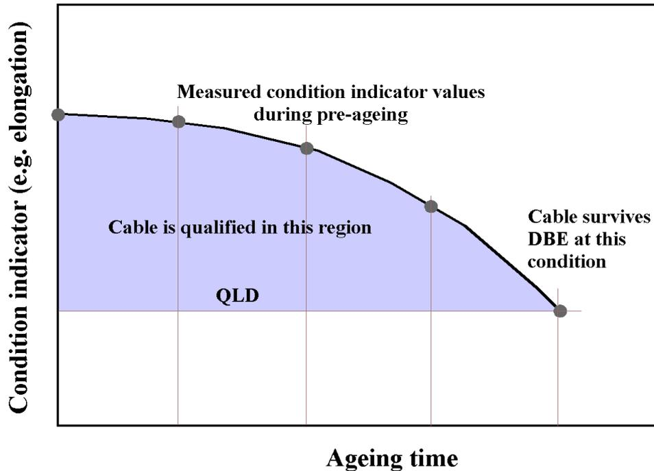
FIG. 5.2. A life curve generated during the pre-ageing stage of EQ for comparison with actual condition of cable.
