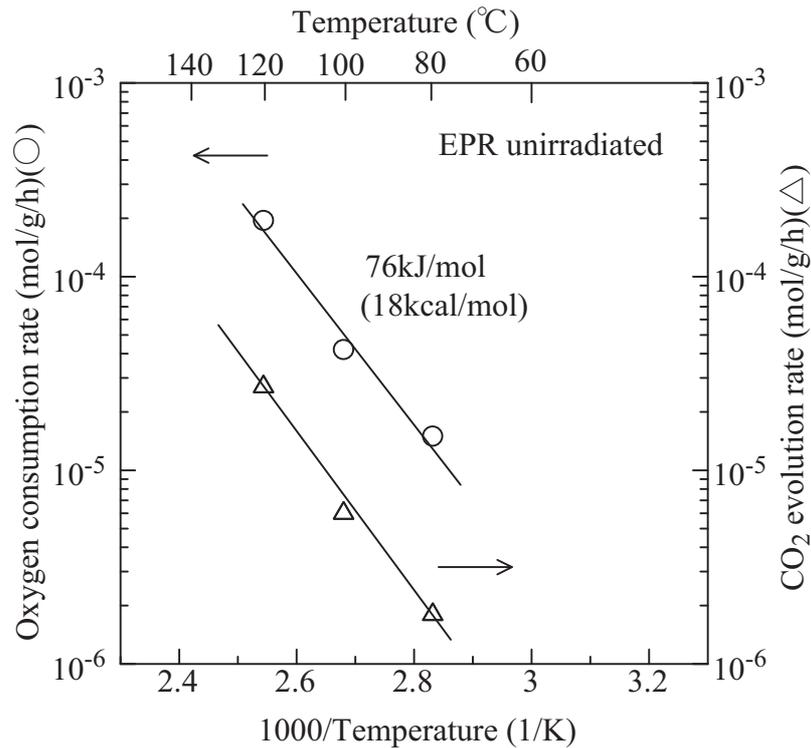
FIG. A-10. Arrhenius plot of oxygen gas consumption and evolved CO<sub>2</sub> for unirradiated EPR.
