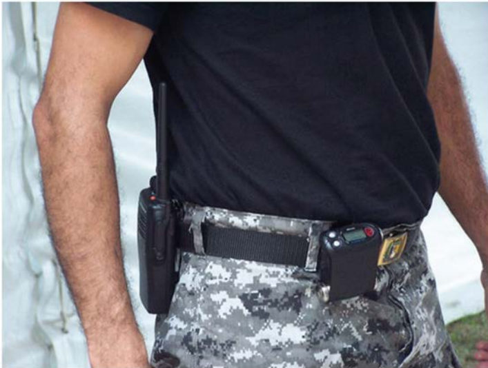
FIG. V-1. Typical example of a PRD.
