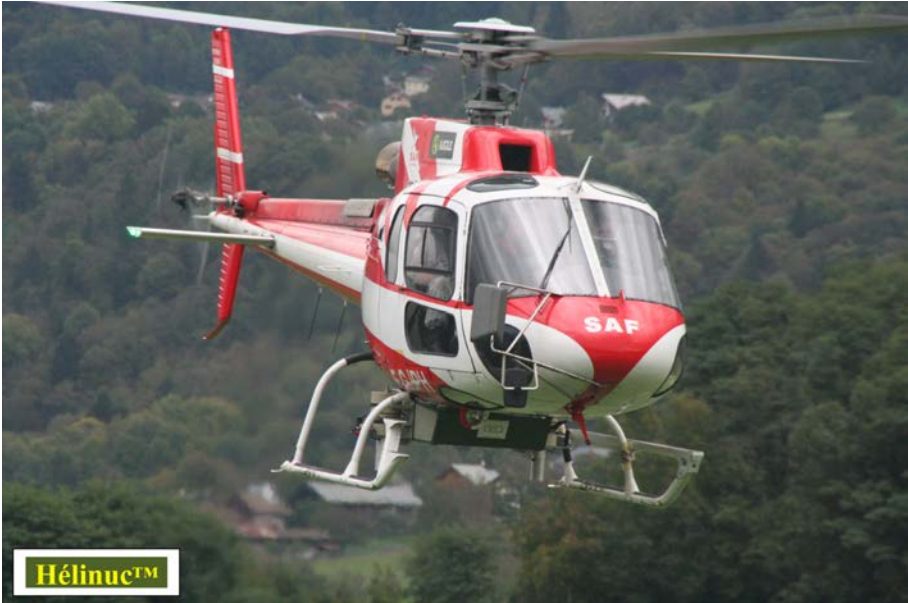
FIG. V-6. Example of an aerial radiation survey system Hélinuc™ (Courtesy CEA/DAM-FRANCE).
