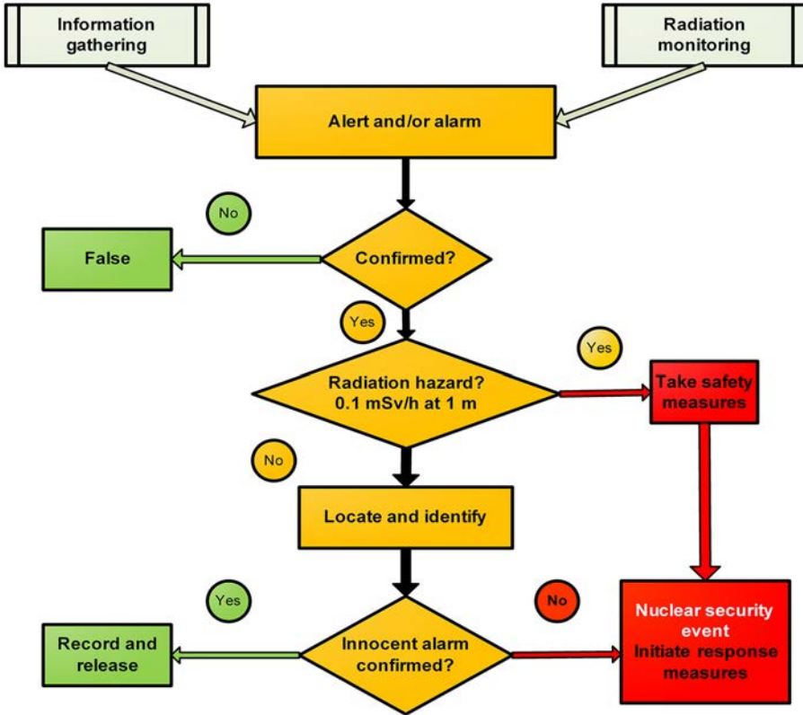
FIG. 1. Generic scheme for assessment of information alert and/or instrument alarm for suspicious objects cleared of explosives.
