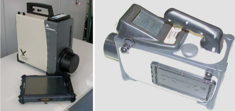
FIG. V-8. Examples of typical high resolution gamma spectrometry systems with the electrically cooled HPGe detector.
