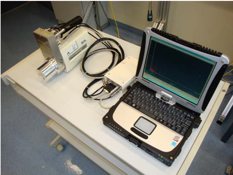
FIG. V-9. Examples of a typical high resolution gamma spectrometry system employing a liquid nitrogen cooled HPGe detector.
