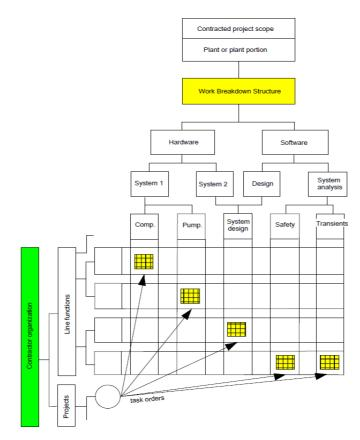
FIG. 10. Responsibility assignment matrix ('line functions' to be changed into 'functions').
