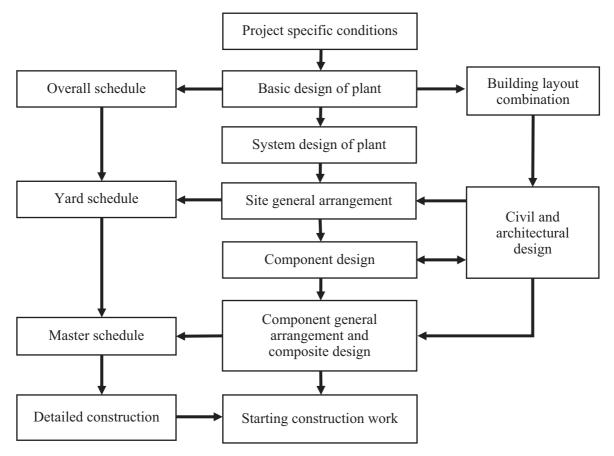
FIG. 7. Example of high level engineering process before the start of construction.
