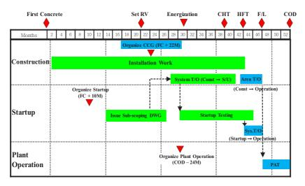
FIG. 23. Typical construction completion process.
