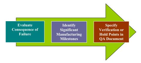
FIG. 15. Graded approach for inspection by the utility.
