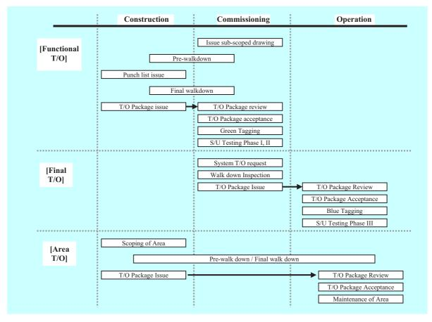
FIG. 24. General turnover process from construction to operation.
