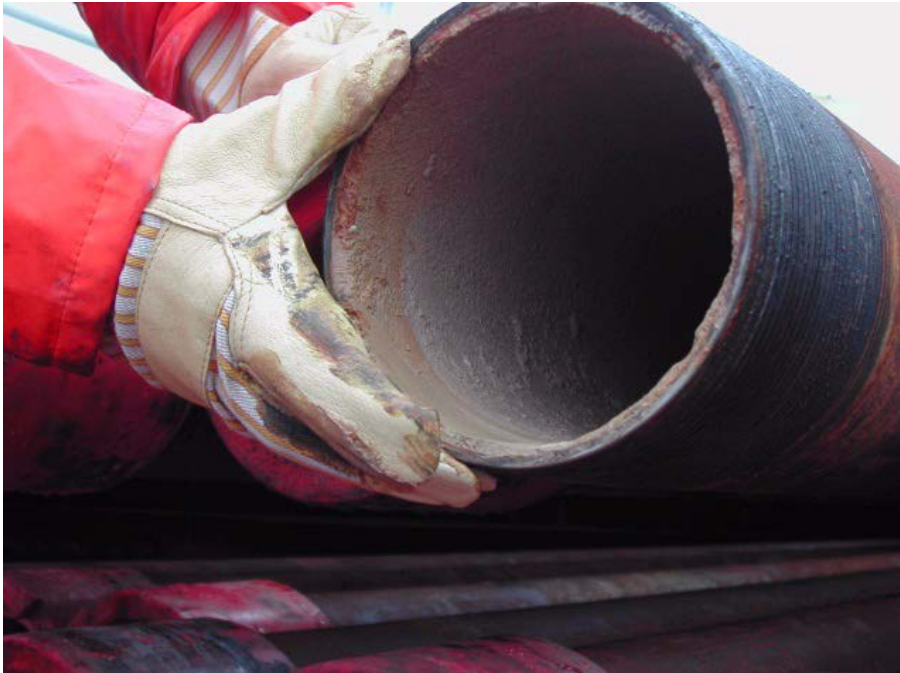
FIG. 13. Oil and gas piping with scale containing ^{226}\text{Ra} and progeny.
