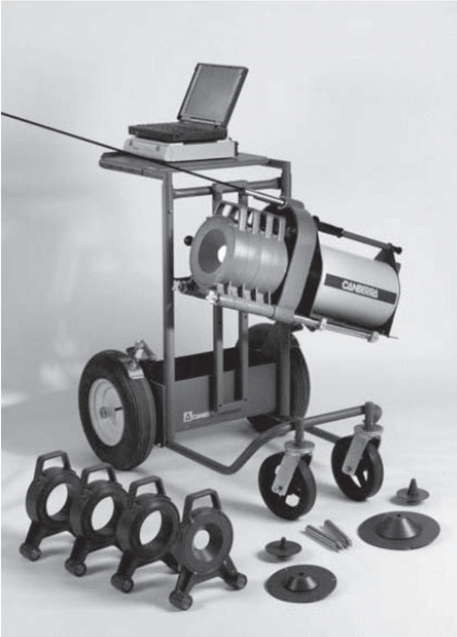
FIG. 5. In situ gamma spectrometer with a collimator manufactured by CANBERRA [22].
