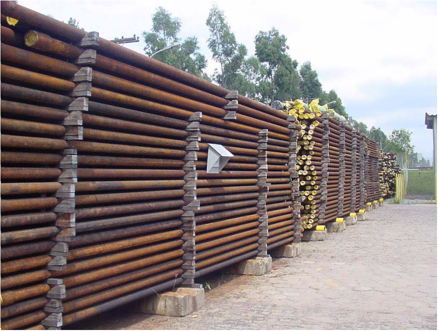
FIG. 14. Piles of pipes contaminated with radioactive scale.
