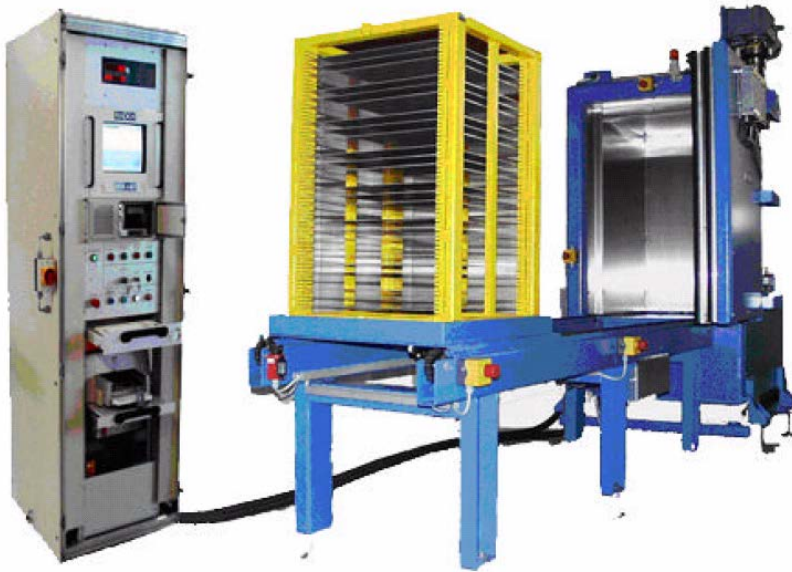
FIG. 4. Bulk monitor manufactured by RADOS (now MIRION Technologies) [21].
