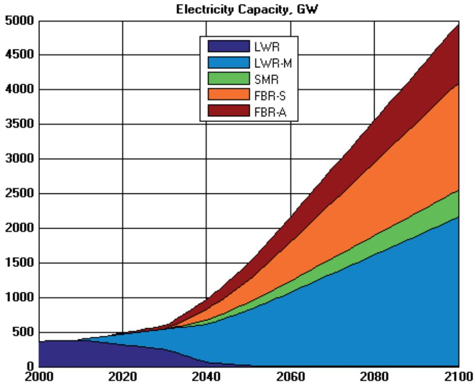
FIG. 14. Global nuclear energy installed capacity by reactor type as a function of time for the MODERATE growth scenario, considering the deployment of two types of fast reactor — case 1.
