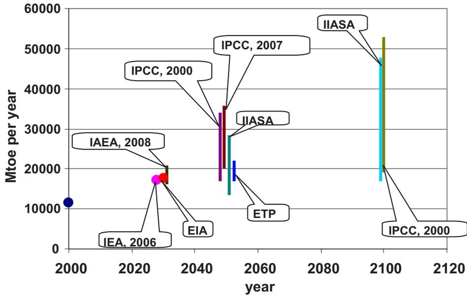
FIG. 1. Scenarios of global primary energy consumption in the twenty-first century (IPCC = International Panel of Climate Change, UN; IIASA = International Institute for Applied Systems Analysis; EIA = Energy Information Agency, DOE; ETP = Energy Technology Perspective, OECD).
