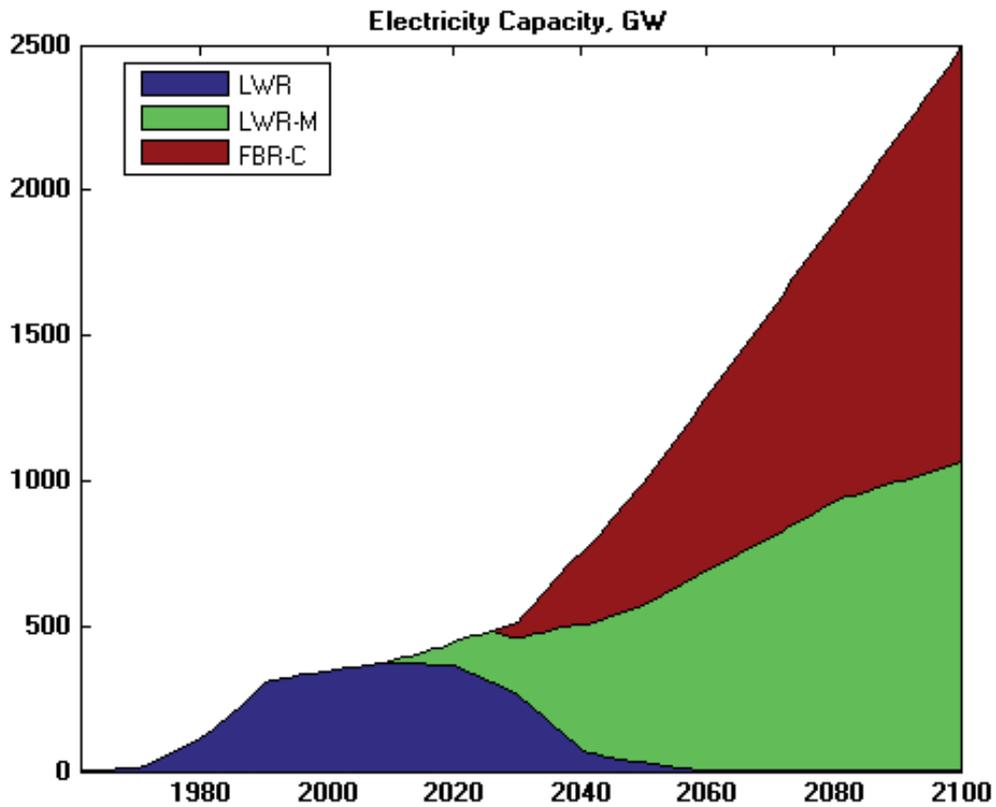
FIG. 10. Global nuclear energy installed capacity by reactor type, as a function of time, for the LOW growth scenario, assuming the deployment of both thermal and fast reactors operating on a closed fuel cycle.
