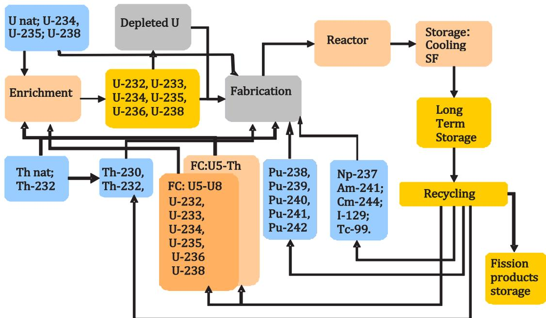
FIG. VI-2. Isotope flow diagram in DESAE.
