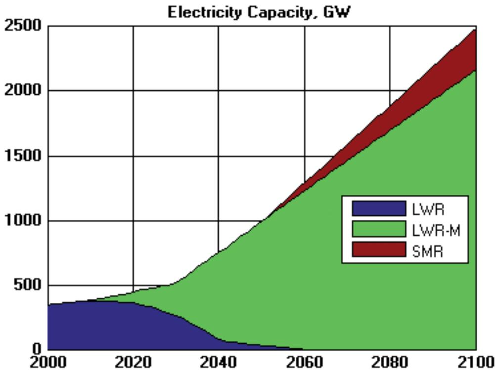
FIG. 8. Assumed global nuclear energy installed capacity by reactor type, as a function of time, for the LOW growth scenario, considering only deployment of thermal reactors.
