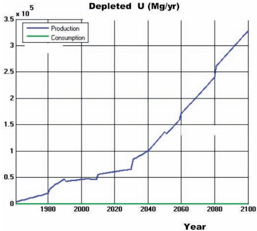
FIG. 12. Amount of depleted uranium produced per year, LOW scenario, corresponding to the nuclear energy system shown in Fig. 10 (thermal plus fast reactors).
