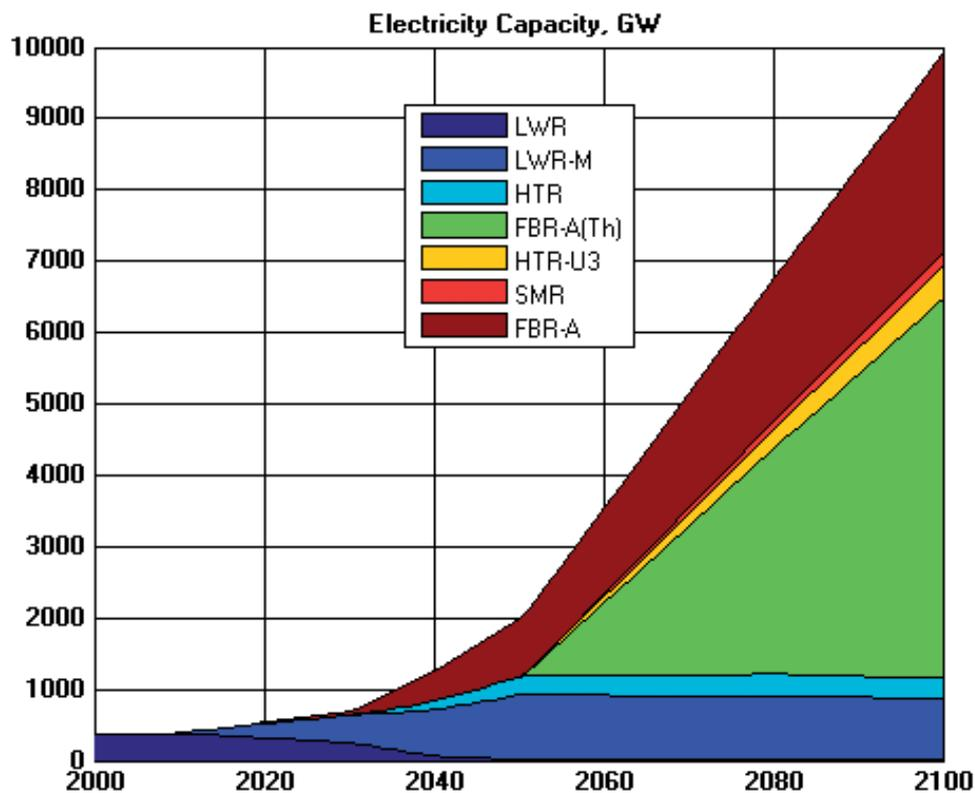
FIG. 19. Assumed global nuclear energy installed capacity by reactor type as a function of time for the HIGH growth scenario.
