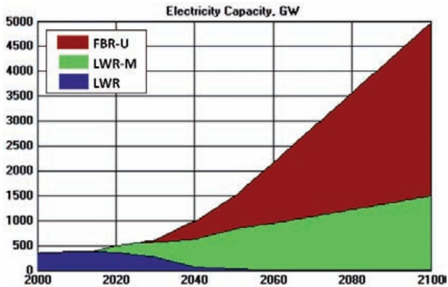
FIG. IV-1. Global nuclear energy installed capacity by reactor type as a function of time for the MODERATE growth scenario, considering the deployment of one type of fast reactor.
