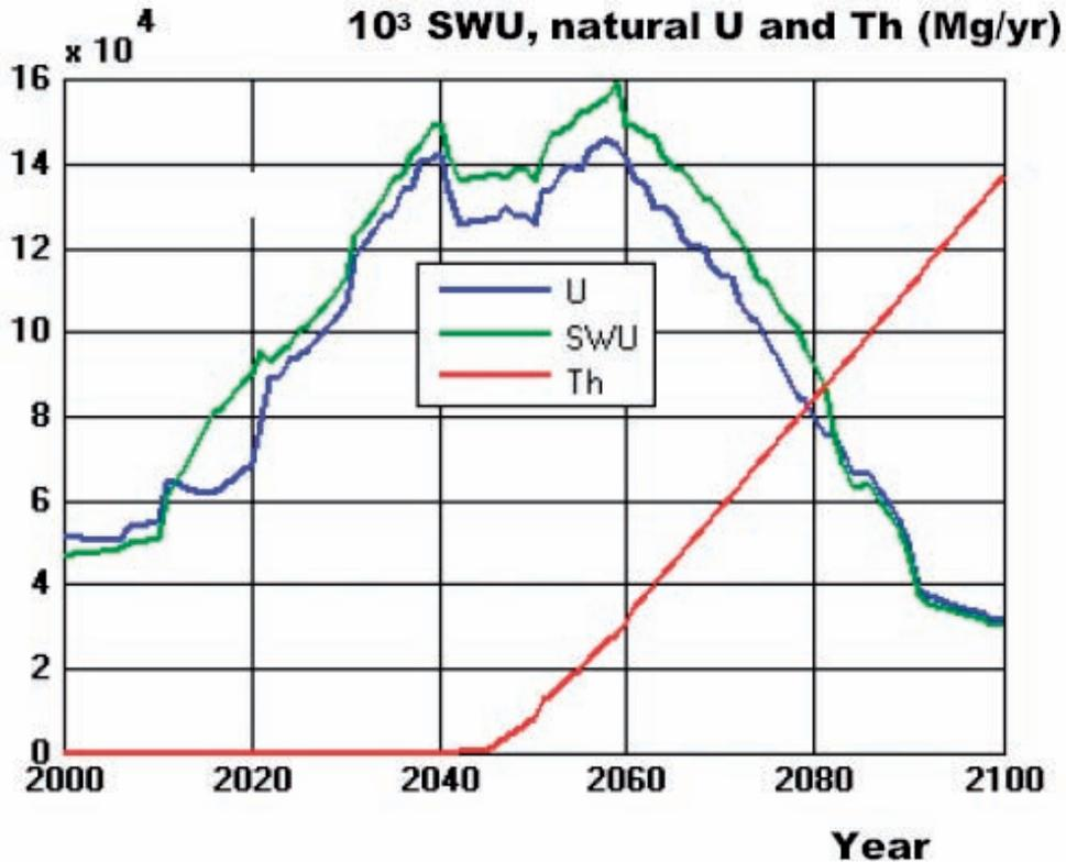
FIG 22. Annual demand of natural U/Th production and separation work for the HIGH scenario in case of use of a fusion neutron source.
