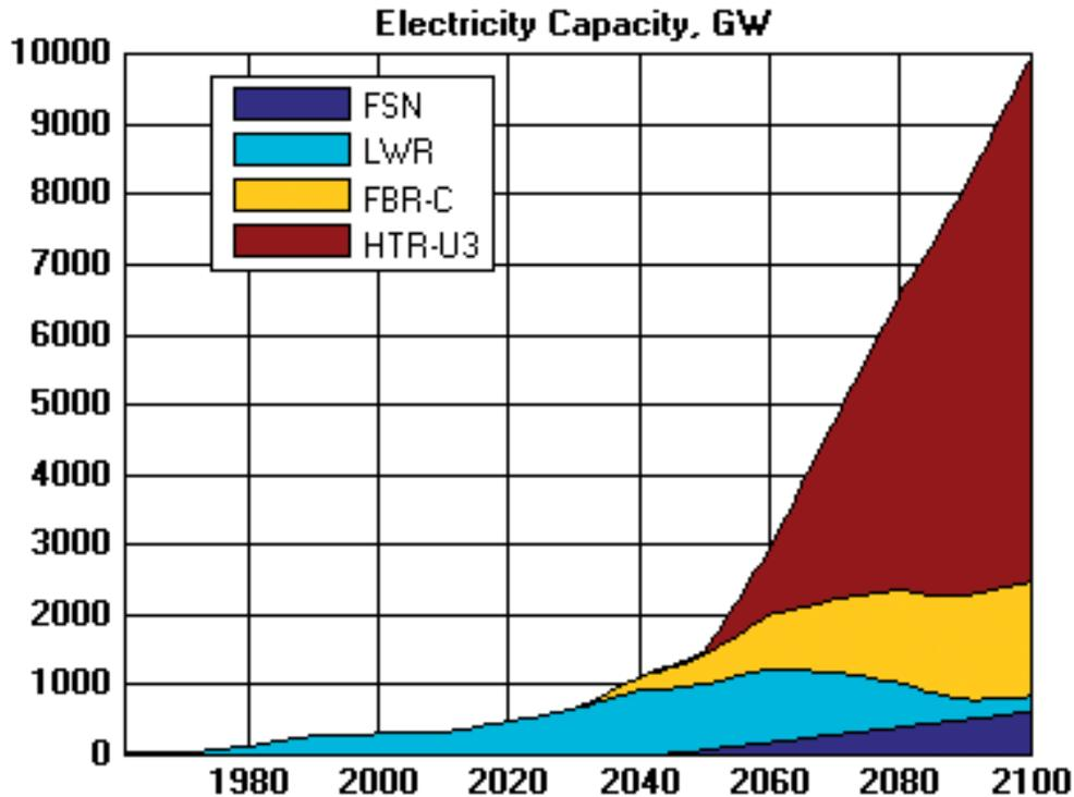
FIG. 21. Global nuclear energy installed capacity by reactor type as a function of time for the HIGH growth scenario, with fusion reactors used to breed fissile material for use in fission reactors.
