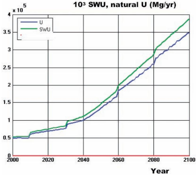
FIG. 16. Annual demand for natural uranium and enrichment for the MODERATE growth scenario — case 1. The accumulated demand for uranium resources totals less than 20 million Mg by 2100.
