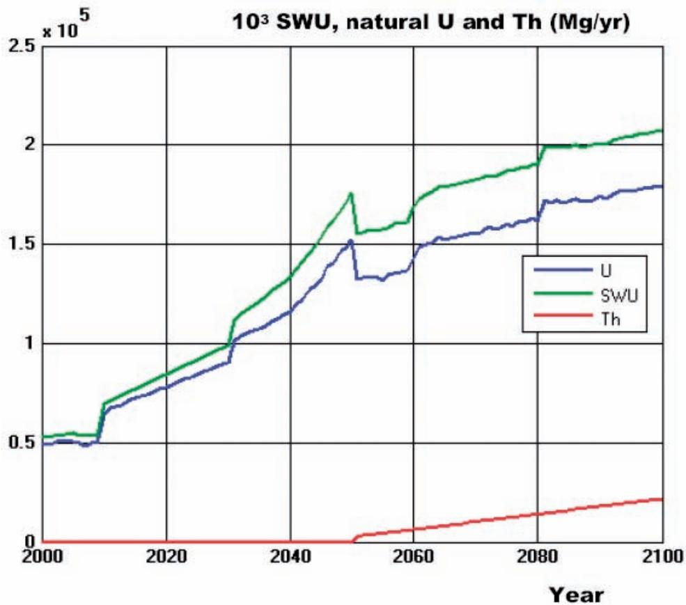
FIG. 20. Annual demand for natural uranium and thorium production and separation work in the HIGH growth scenario.
