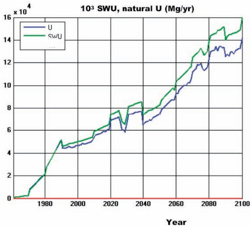
FIG. 11. Annual U production and SWU demand corresponding to the nuclear energy system shown in Fig. 10 (thermal plus fast reactors in LOW growth scenario).
