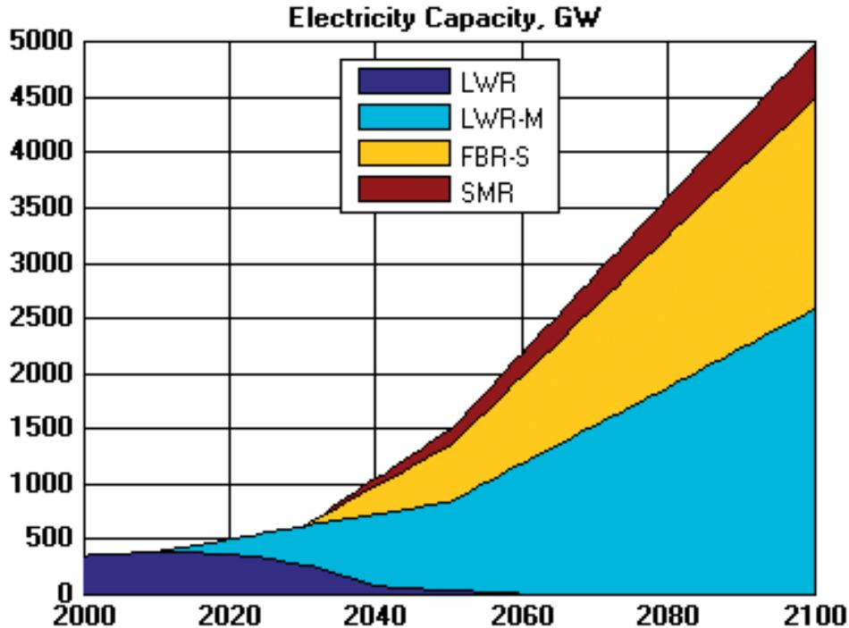
FIG. 15. Global nuclear energy installed capacity (GW(e)) by reactor type, as a function of time, for the MODERATE growth scenario, considering the deployment of only one type of fast reactor — case 2.
