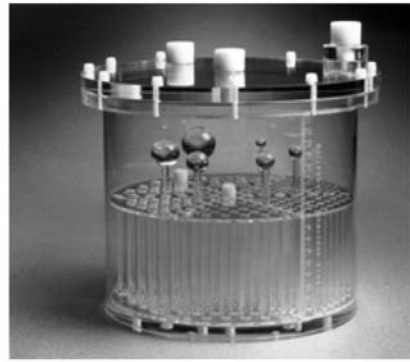
FIG. 45. Data Spectrum ECT phantom (Jaszczak phantom), showing the individual inserts for resolution and contrast assessments (left) and the assembled phantom (right).
