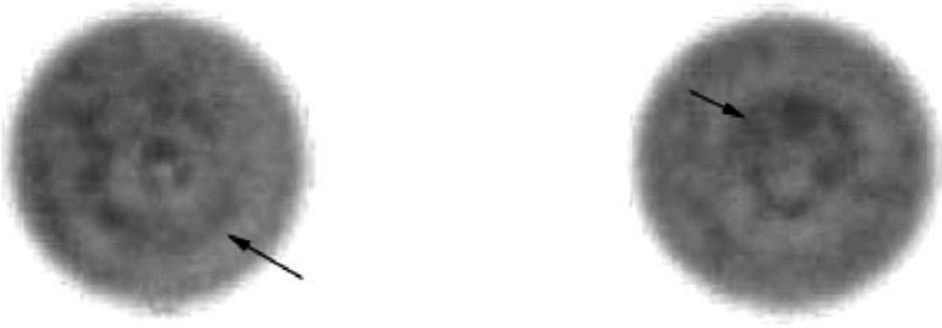
FIG. 48. Partial ring artefact from a dual head SPECT system. Dual detector SPECT system with detector heads at 180^\circ from each other, 360^\circ total angle of rotation (each detector rotates through 180^\circ ), circular orbit. SPECT acquisition of a uniform cylinder, no attenuation correction and no uniformity correction applied. Two images from the set of transverse slices are shown. Different non-uniform artefacts are seen in the transverse slices. In the left image, the centre of the innermost ring corresponds to the centre of rotation. Note that the phantom was positioned off-centre so that this ring artefact does not correspond exactly to the centre of the phantom. Other artefacts are semicircles (arrowed) centred around the axis of rotation and not full rings as would be expected from a 360^\circ rotation of a single detector head SPECT system. In multiple head SPECT systems, each head will contribute to the non-uniformity of the resultant SPECT uniformity. Since the non-uniformity in each head will be different, the resultant pattern observed in the reconstructed images will not be full rings but partial rings (see Ref. [3]).
