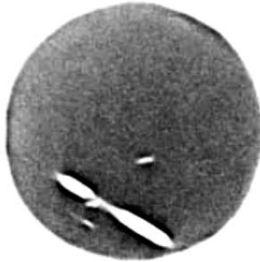
FIG. 21. Cracked crystal. Routine intrinsic uniformity testing revealed various cold areas with hot edges. These cracks are due to thermal changes. The hot edges are due to light reflection at the crack of the crystal (see Ref. [3]).
