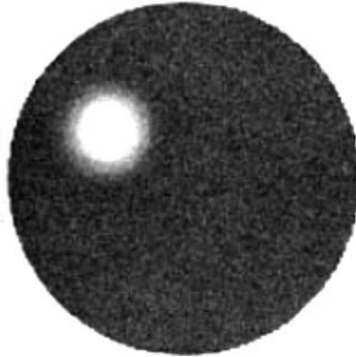
FIG. 14. Defective PMT. Daily quality control image of flood field uniformity, ^{99m}\text{Tc} , 15% energy window, 4 million counts. Results: The image shows a large, circular cold area that was due to a defective PMT. Note the inner halo of lower counts and the outer halo of higher counts at the edge of the defect. Service is required (see Ref. [3]).
