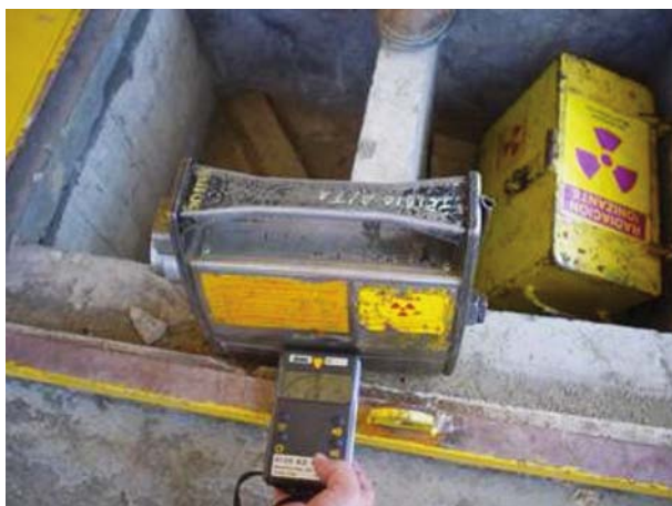
FIG. 2. Amersham Sentinel gamma radiography equipment, model 660, series 5657.
