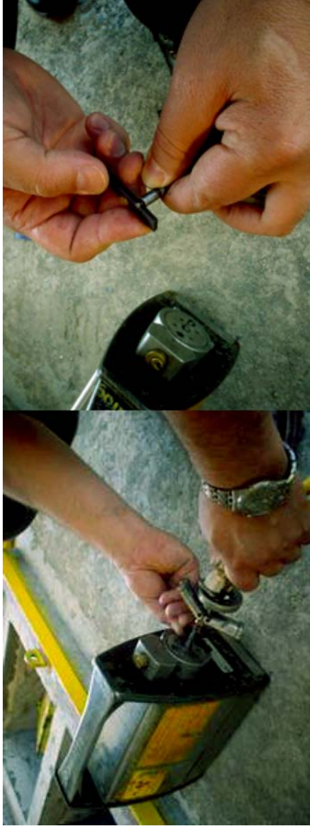
FIG. 11. Verification of the connection between the conductor cable and the source.
