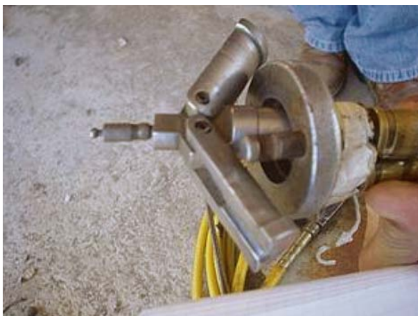
FIG. 4. A connector to the source and the projection exposure container (projector).
