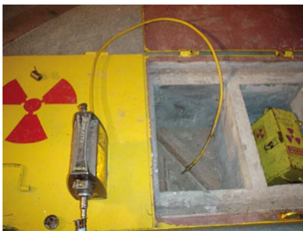
FIG. 5. A gamma radiography unit: the complete connection, including the guide tube.
