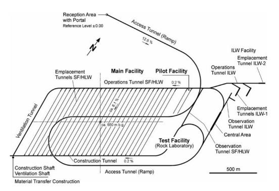
FIG. IV-1. Plan view of the repository for SNF, vitrified HLW and ILW-LL in Opalinus Clay.
