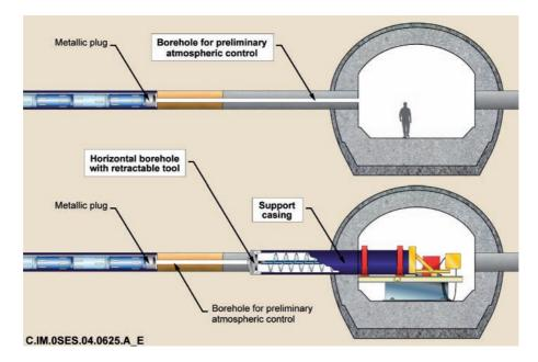
FIG. 5. French concept: Cell seal boring before vitrified HLW retrieval.
