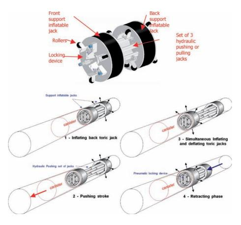
FIG. 3. French concept: Prototype robot for vitrified waste package emplacement and retrieval.
