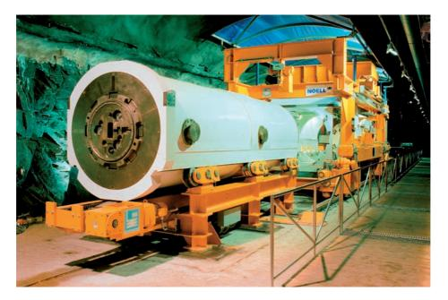
FIG. III-2. Prototype deposition machine for vertical disposal (the machine tilts the canister into the deposition hole).
