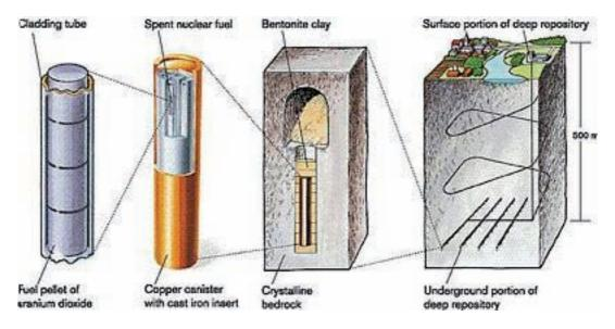
FIG. 1. Representation of the KBS-3 concept.
