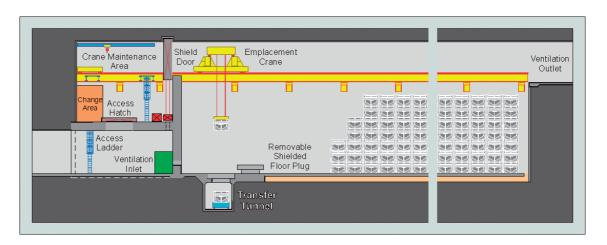
FIG. 6. United Kingdom Nirex concept: Retrievable underground storage facility.
