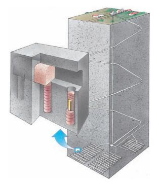
FIG. III–1. Illustration of the KBS-3V concept for the storage of SNF.
