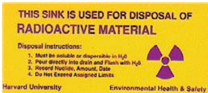
FIG. 2. Typical sign at a dedicated sink.
