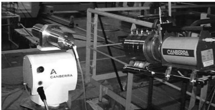
FIG. 3. CARTOGAM and ISOCS for in situ nuclear measurement systems.
