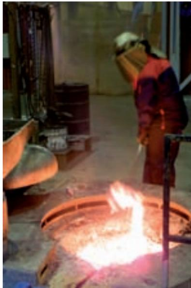
*FIG. 5. Removal of slag.*
