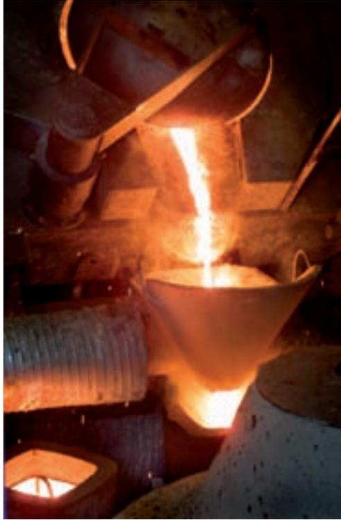
*FIG. 1. Casting of ingots.*
