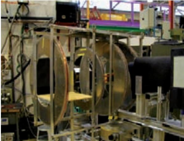
FIG. 2. Coils for polarized neutron reflectometry and off-specular magnetic scattering with wide angle  $^3\text{He}$  spin analysis as it was used in an experiment at EVA (ILL, Grenoble) [4]. The  $^3\text{He}$  bottle itself is not shown in the picture.
