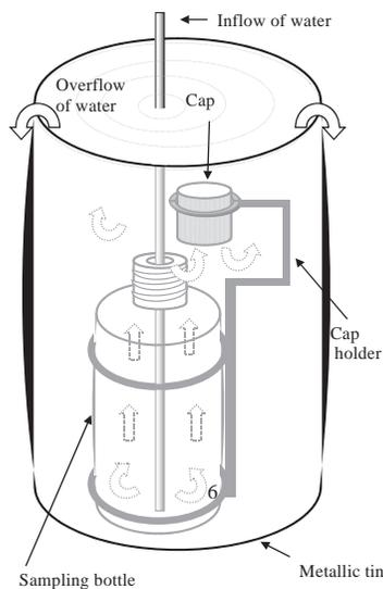
FIG. 12.4. Apparatus for collecting groundwater samples by using small sized 50 mL glass bottles without contact to air.
