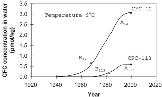
FIG. 5.1. Effect of dilution of CFC containing water by CFC-free water. The curves represent CFC concentrations in water in equilibrium with atmospheric air as a function of time for a water temperature of 9°C. Solid circles mark the CFC containing water sample (year 2000). Open circles represent the measured CFC concentrations of the dilution of 25% of that water by 75% of CFC-free water.
