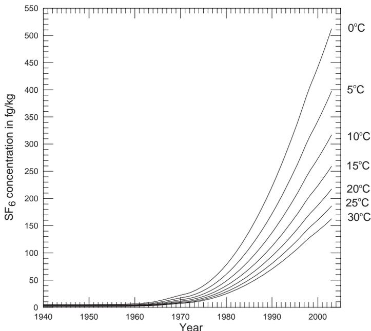
FIG. 10.2. Concentration of  $SF_6$  (femtograms per kilogram (fg/kg)), in water as a function of temperature in equilibrium with North American air at 1013.25 hPa total pressure.
