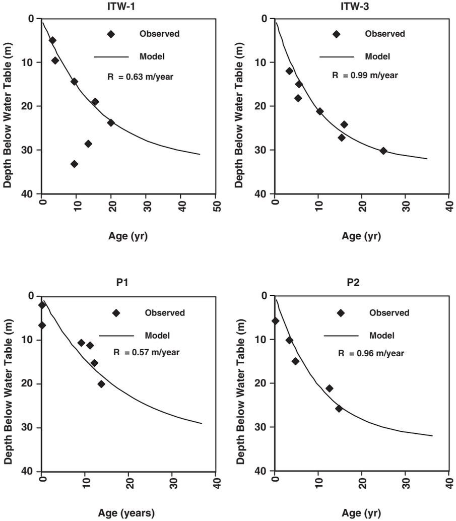
FIG. 7.5. Observed and simulated distribution of groundwater ages are shown. The simulated values were produced using Eq. (6.1), Chapter 6. The recharge rate was adjusted to produce a best fit between observed and simulated values.
