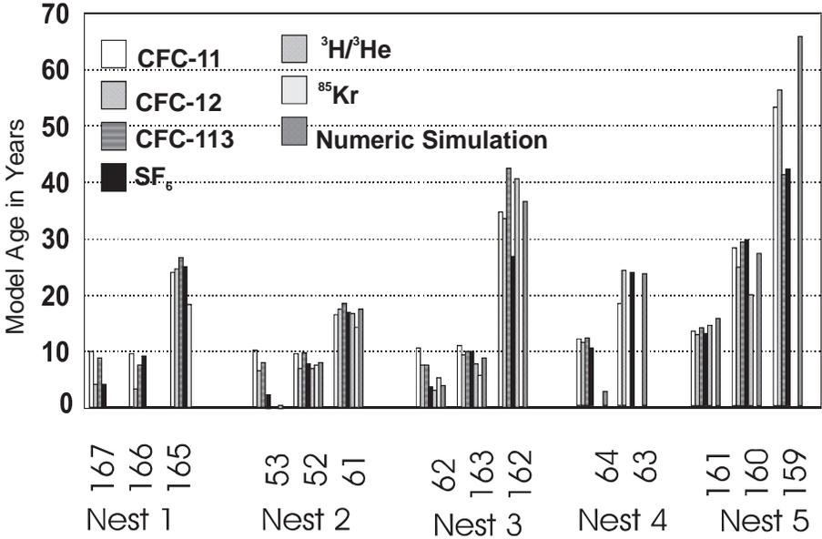
FIG. 9.3. Comparison of model groundwater ages using six different dating methods at Locust Grove, Maryland, USA.
