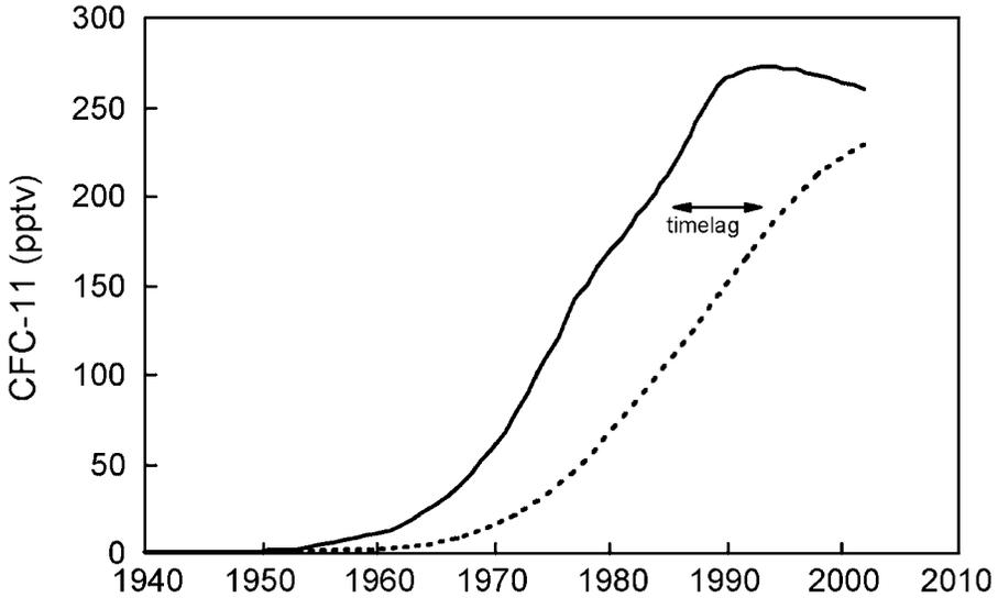
FIG. 4.2. Concentrations of CFC-11 in the atmosphere (solid line), and in the soil atmosphere immediately above a water table at 30 m depth (broken line). The horizontal distance between the two lines indicates the time lag, which was 8–9 years before 1980, and increased to 15 years in 2002.
