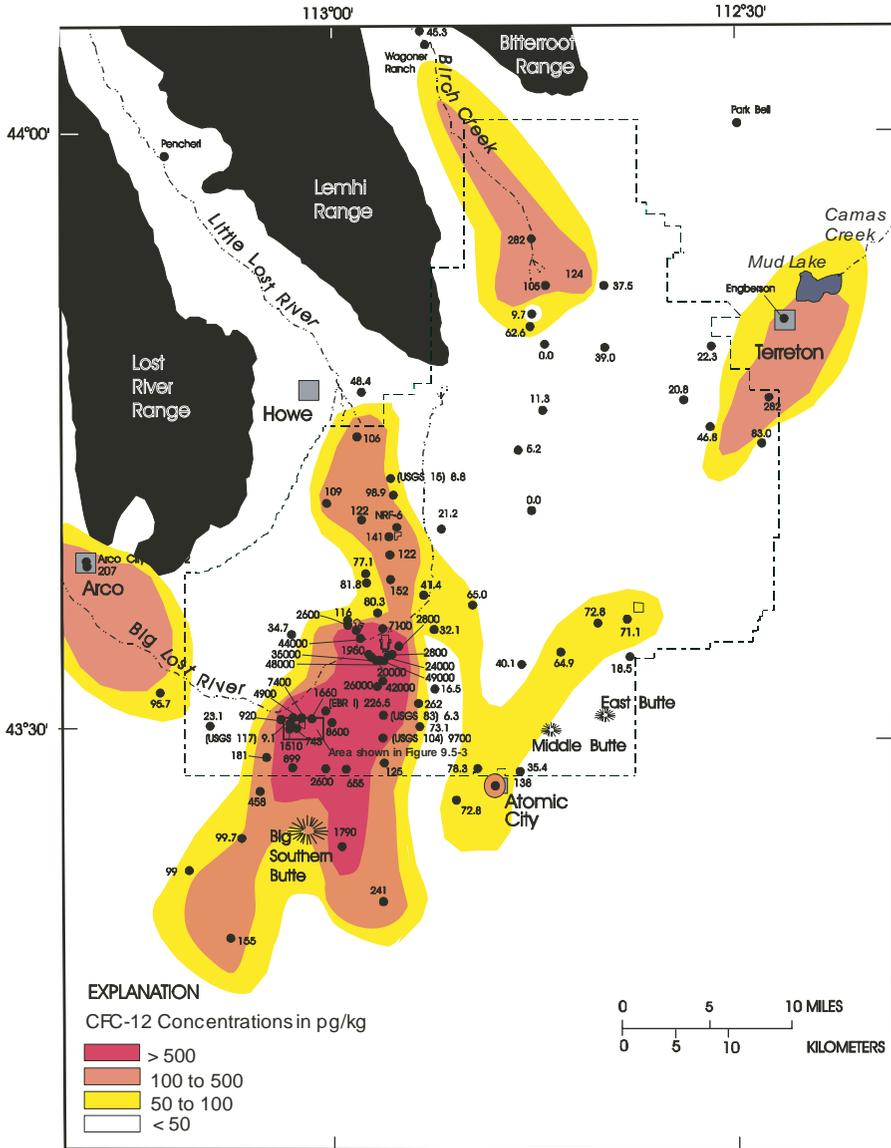
FIG. 9.14. Concentration of CFC-12 in groundwater at the Idaho National Engineering and Environmental Laboratory and vicinity. Samples with greater than 400 pg/kg are waters with higher than air-water saturations of CFC-12.
