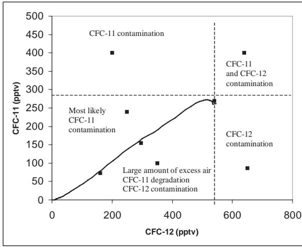
FIG. 8.1. The tracer plot of CFC-11 versus CFC-12 in pptv shows piston flow line, and regions where samples affected by contamination, degradation or excess air would plot.
