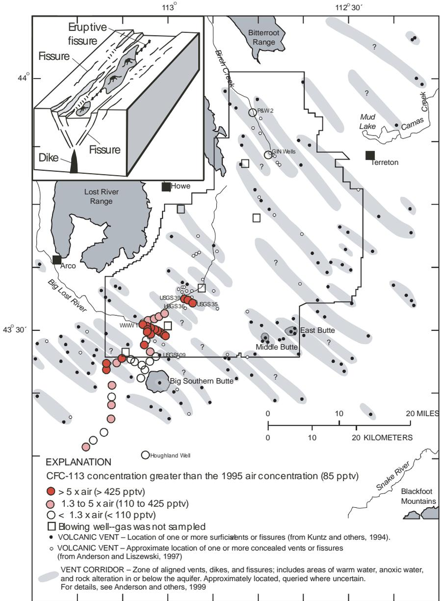
FIG. 9.16. Distribution of CFC-113 in the unsaturated zone at INEEL. The insert is a conceptual model of a vent corridor and the associated fractures (Anderson et al., 1999). Most gas samples were collected from a depth of 1 m, a few samples were collected from gases blowing from around the annulus of wells.
