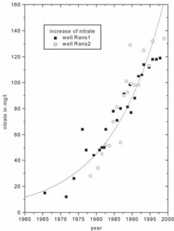
FIG. 9.27. Time series of nitrate concentrations in two wells in Maikammer, Germany.
