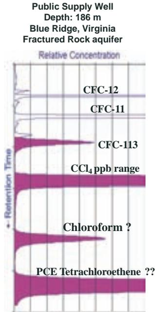
FIG. 9.20. The GC–ECD chromatogram of a water sample is shown from a public supply well in fractured rock in the Blue Ridge province of Virginia. The well has a total depth of 186 m with 175 m of casing and a single water bearing fracture at 186 m.
