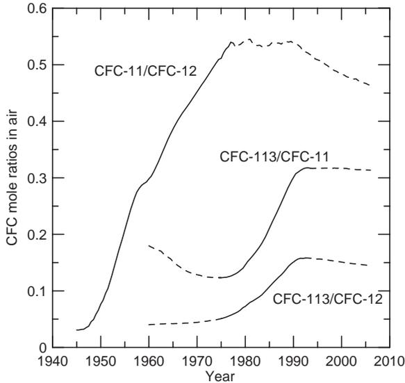
FIG. 3.3. Historical atmospheric ratios of CFC-11/CFC-12, CFC-113/CFC-12 and CFC-113/CFC-11 in North American air. The solid lines show the useful dating range for each ratio.
