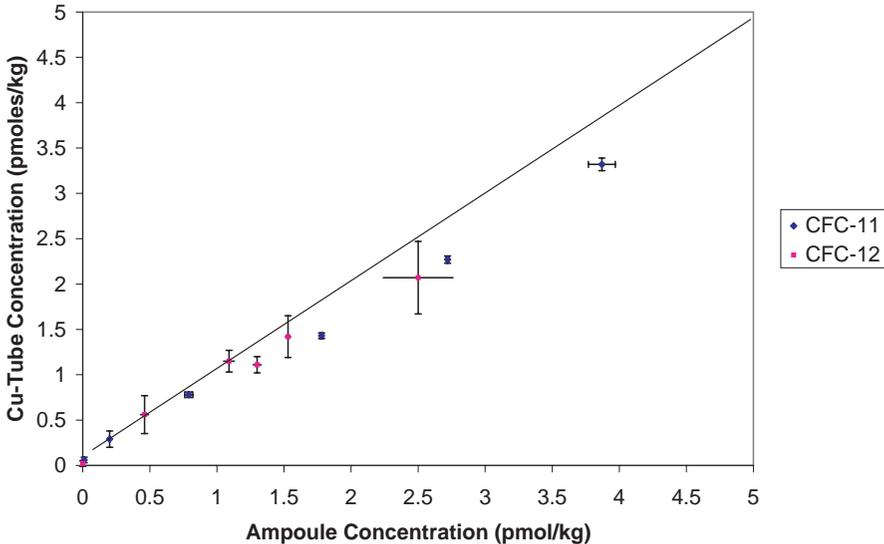
FIG. 12.7. Comparison of the copper tube sampling method with the ampoule method. (After Heilweil et al. (2000).)
