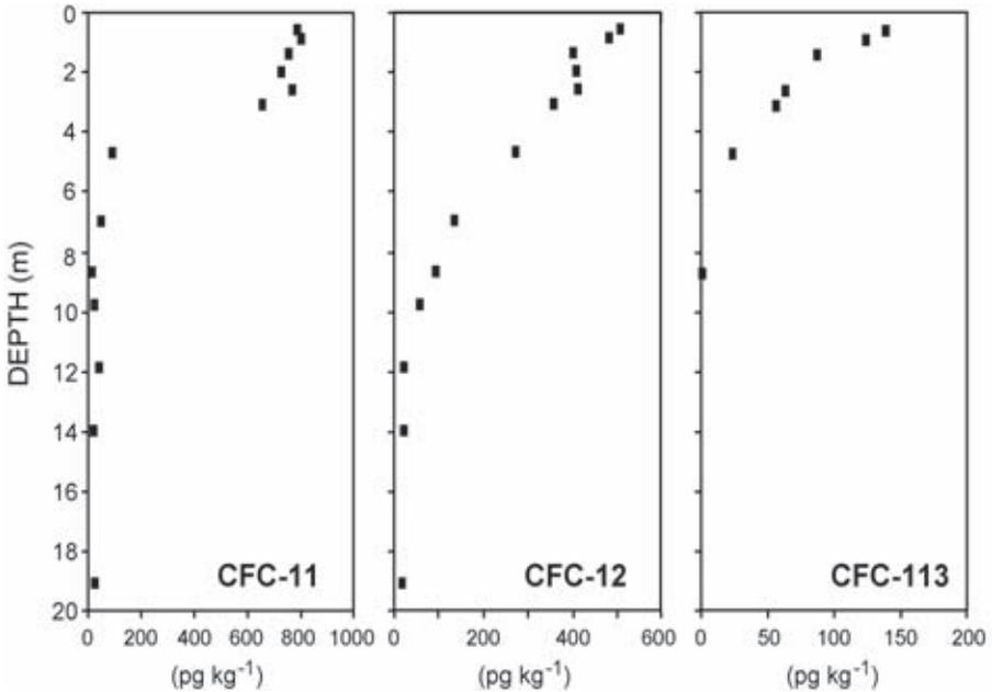
FIG. 9.6. Measured depth profiles of CFCs at Nest 28.
