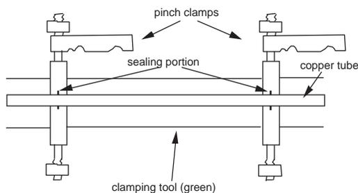
FIG. 12.5. Copper sampling tube with external pinch clamps.
