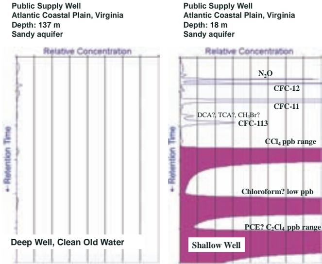
FIG. 9.19. Comparison of two GC-ECD chromatograms of water from public supply wells in a sandy aquifer in the Atlantic coastal plain of Virginia. The sample on the left is from a depth of approximately 126–134 m in coastal plain sands and is virtually free of CFCs and other halocarbons. The sample on the right is from a screened interval of 13.4–18 m depth and contains all three CFCs and significant detections of other halocarbon compounds.
