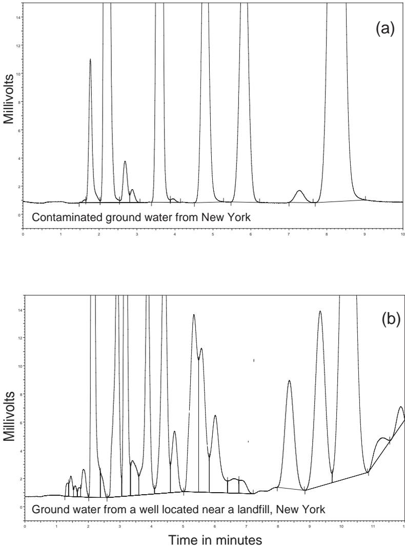
FIG. 12.13. Chromatograms from the U.S. Geological Survey Chlorofluorocarbon Laboratory show: (a) an oxic water sample located downgradient of a capped landfill in the state of New York that is beginning to be affected with VOCs leached from the landfill; and (b) a highly contaminated anaerobic water sample in the contaminant plume beneath a capped landfill in the state of New York. (Plummer and Busenberg, unpublished data (2001).)
