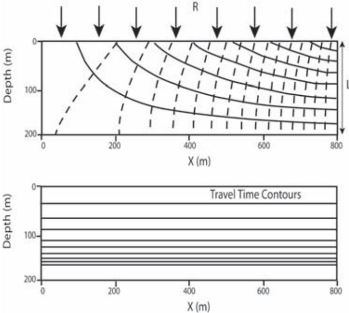
FIG. 6.1. Unconfined aquifer of constant thickness ( $L$ ) and uniform recharge ( $R$ ). The upper diagram is a flow net for this system; the solid lines represent flow paths and the broken lines represent equipotential lines. The lower diagram shows contours of travel time, with age increasing exponentially with depth. The contour interval for travel times is arbitrary, as it depends on the values for recharge and porosity.
