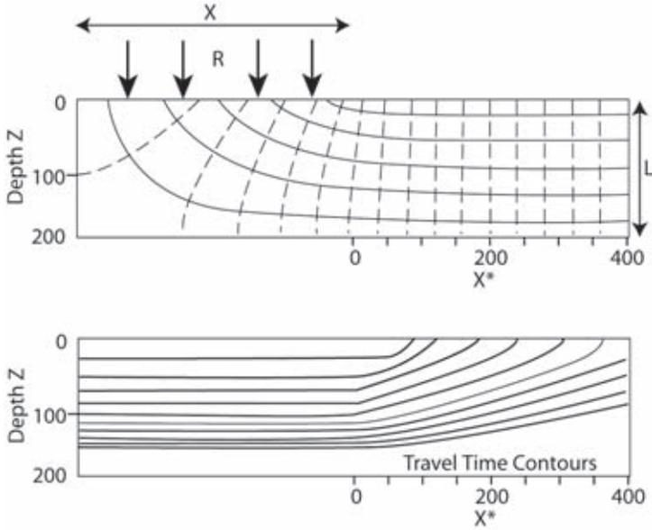
FIG. 6.4. A confined aquifer of constant thickness that receives recharge from an adjacent unconfined aquifer of constant thickness is shown. The upper diagram is a flow net for this system while the lower diagram shows contours travel time. The contour interval for travel times is arbitrary, as it depends on the values of recharge ( $R$ ).
