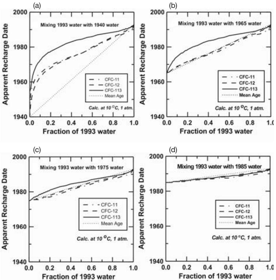
FIG. 5.3. Calculations showing the effect on the apparent age of mixing 1993 water with older water: (a) mixing with old, CFC-free water; (b) mixing with water recharged in 1965; (c) mixing with water recharged in 1975; (d) mixing with water recharged in 1985. The plots were constructed assuming recharge at 10°C and 1013.25 hPa total pressure.
