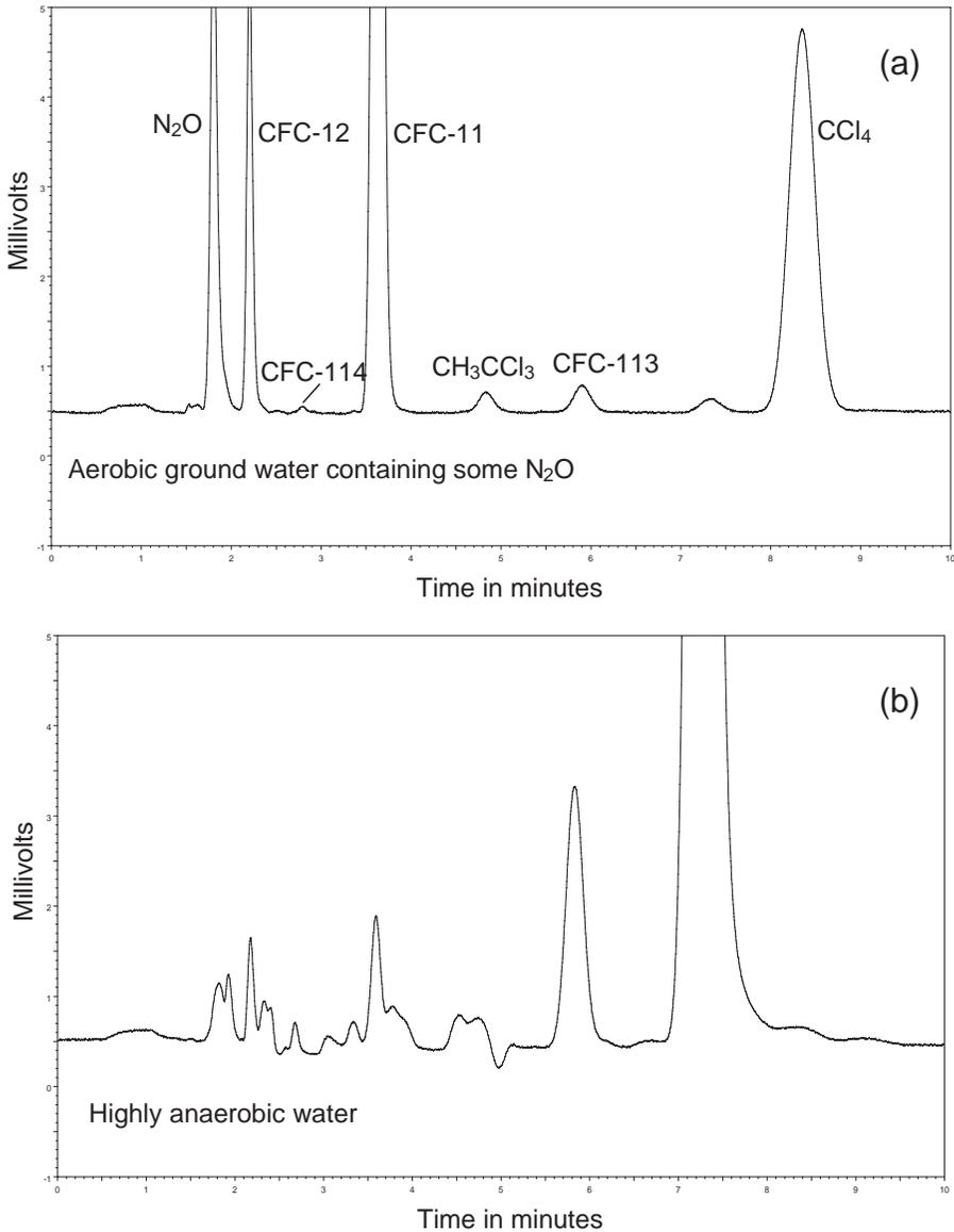
FIG. 12.12. Chromatograms from the U.S. Geological Survey Chlorofluorocarbon Laboratory show: (a) an example of a nearly clean, aerobic water with a stable background that is typical of oxic groundwater samples; and (b) an example of a highly degraded anoxic water sample. Many of the peaks in sample (b) are degradation products of the CFCs and other halocarbons that were originally present in the sample. The unstable background of the chromatogram in (b) is characteristic of anoxic waters.
