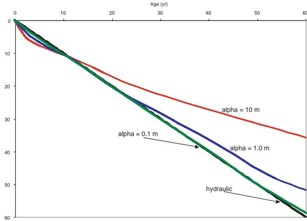
FIG. 4.7. The results of 1-D transport of CFC-12 using various values for longitudinal dispersivity ( $\alpha$ ) are shown. The curves represent solutions to the advection–dispersion equation using the CFC-12 time history in the atmosphere as an input function. In many (if not most) shallow aquifers, the dispersivity acting in the vertical direction will be less than 1.0, resulting in only minimal effects of dispersion on CFC ages.
