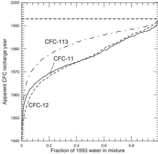
FIG. 5.2. Effects of mixing of recent water (recharged in the year 1993) with CFC-free water on the apparent recharge year of the mixture, as a function of the fraction of recent water in the mixture. The curves are analogue to the CFC air mixing ratios, and show apparent recharge years. The dashed line shows apparent recharge years derived from the CFC ratios which, in the case of mixing with a CFC-free component, is independent of the mixing fraction.
