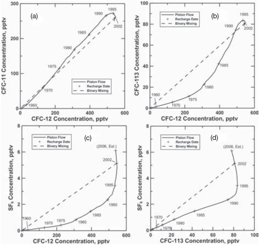
FIG. 5.6. Tracer plots comparing CFC-11, CFC-12, CFC-113 and SF<sub>6</sub> concentrations in pptv for North American air. The solid lines represent unmixed (piston flow) with selected apparent ages ('+'). The dashed line shows one example of binary mixing for the case of water recharged in 2002 diluted with old, CFC-free water.
