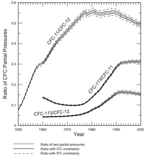
FIG. 4.5. Uncertainty in the ages of groundwater dated by the ratio method introduced by  $\pm 2$  and  $\pm 5^\circ\text{C}$  error in the temperature used to calculate the CFC partial pressures. The water in this example recharged at  $10^\circ\text{C}$ .
