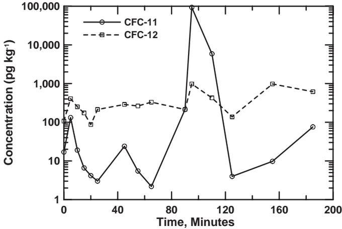
FIG. 12.1. Concentrations (pg·kg<sup>-1</sup>) of CFC-11 and CFC-12 in discharge from a water supply well in fractured sandstone from central Oklahoma, USA. (Modified from Busenberg and Plummer (1992).)
