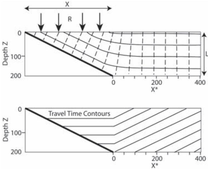
FIG. 6.5. Confined aquifer of constant thickness that receives recharge from an adjacent unconfined aquifer of linearly increasing thickness. The upper diagram is a flow net for this system, while the lower diagram shows contours travel time. The contour interval for travel times is arbitrary, as it depends on the values of recharge ( $R$ ).
