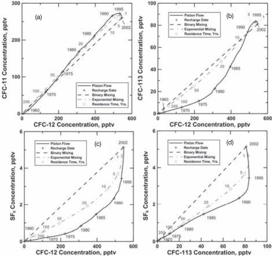
FIG. 6.7. Tracer plots comparing CFC-11, CFC-12, CFC-113 and SF<sub>6</sub> concentrations in pptv for North American air are shown. The solid lines represent unmixed (piston flow) with selected apparent ages ('+'). The dark dashed lines show one example of binary mixing, for the case of water recharged in 2002 diluted with old, CFC-free water. The dash-dot lines represent exponential mixing for residence times of 1 to 200 years. (Modified from Plummer et al. (2003).)
