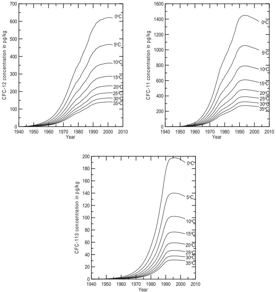
FIG. 4.3. The concentration of CFCs in water as a function of temperature in equilibrium with North American air at sea level are shown.
