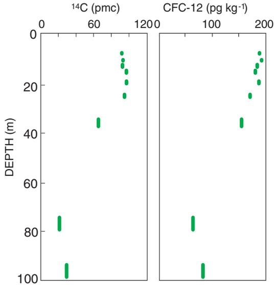
FIG. 9.23. Vertical profiles are shown of  $^{14}\text{C}$  and CFC-12 obtained from a piezometer nest installed in Mintaro Shale.
