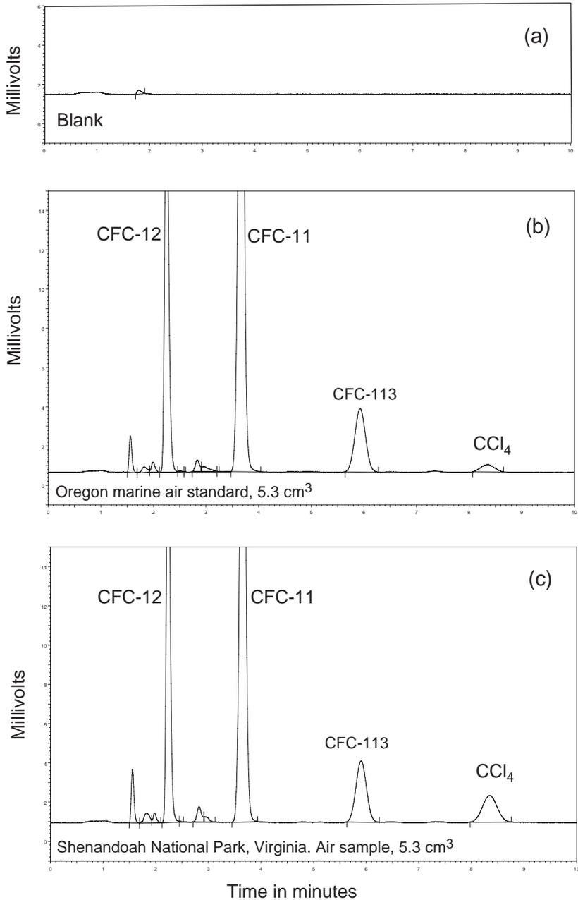
FIG. 12.10. Sample chromatograms from the U.S. Geological Survey Chlorofluorocarbon Laboratory show: (a) an instrument blank of 5.3 cm<sup>3</sup> of ultra-pure N<sub>2</sub> carrier gas; (b) 5.3 cm<sup>3</sup> of Oregon marine air standard; (c) 5.3 cm<sup>3</sup> of 2001 air from the Air Monitoring Station at Shenandoah National Park, Virginia.
