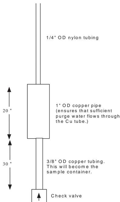
FIG. 12.6. The diagram shows a Cu tube sampler when used as a 'bailer' (1 in. = 25.4 mm).
