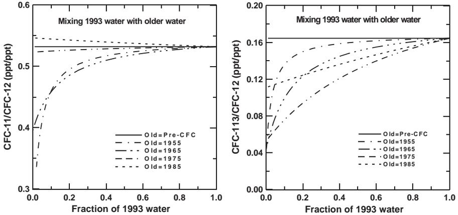
FIG. 5.4. Calculations showing variations in the CFC-11/CFC-12 and CFC-113/CFC-12 ratio in binary mixtures of modern 1993 water with various fractions of water recharged in the years 1955, 1965, 1975 and 1985. The CFC ratios are constant only in binary mixtures of young water with old, CFC-free water. These calculations were made using North American air at 10°C and 1013.25 hPa total pressure.
