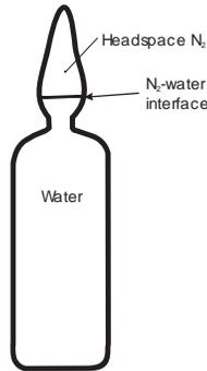
FIG. 12.8. Ampoules used to sample water for CFCs. The location of the water- $N_2$  interface is marked with a pen. The volume of the headspace is determined after the analysis of the sample by filling the top of the ampoule to the mark with water and then determining the weight of the water by difference.
