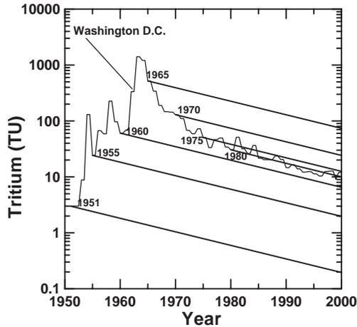
FIG. 11.1. A smoothed record of  $^3\text{H}$  in precipitation at Washington, D.C., is shown. Parallel lines show the path of decay of  $^3\text{H}$  in groundwater if recharged from precipitation in the years 1951, 1955, 1960, 1965, 1970, 1975 and 1980.
