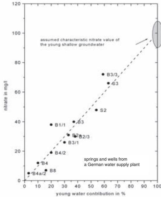
FIG. 9.24. Relationship shown between nitrate concentration and per cent young water as determined using CFC data with a binary mixing model.
