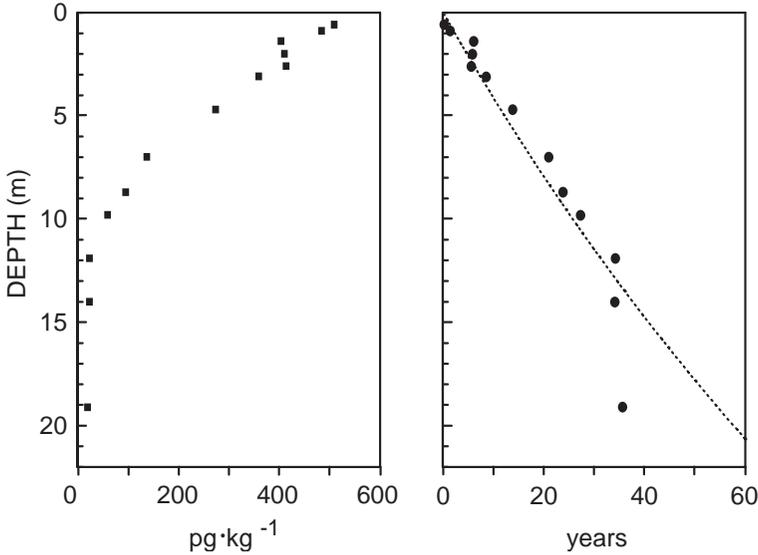
FIG. 7.1. Profiles of CFC-12 concentration and apparent CFC-12 age in the Sturgeon Falls aquifer are shown. The broken line represents results of a two-dimensional flow model calibrated using tritium data, from Cook et al. (1995).
