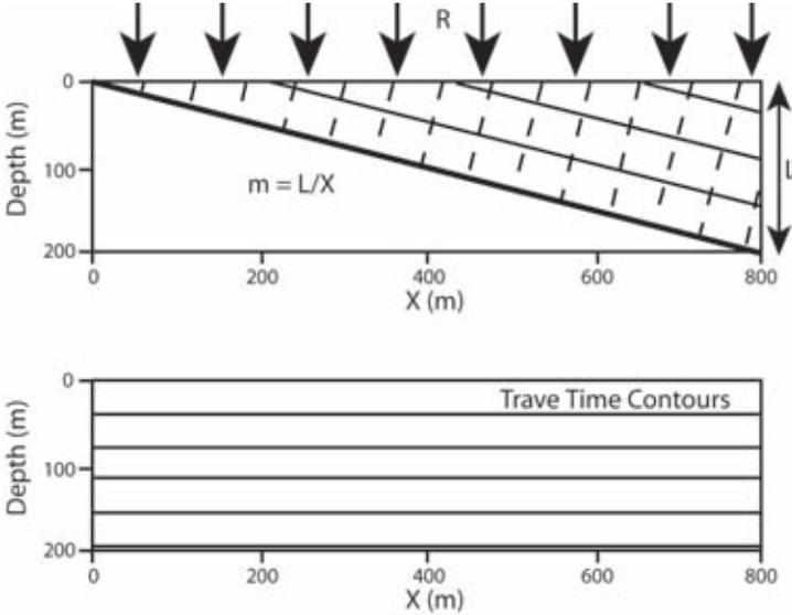
FIG. 6.3. Unconfined aquifer with linear increasing thickness ( $L$ ) and uniform recharge ( $R$ ). The upper diagram is a flow net for this system while the lower diagram shows contours of travel time. The contour interval for travel times is arbitrary, as it depends on the value of recharge.
