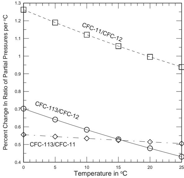
FIG. 4.4. Per cent error in the ratio of two CFC partial pressures for waters recharged between 0 and 25°C for an uncertainty of 1°C in the recharge temperature.
