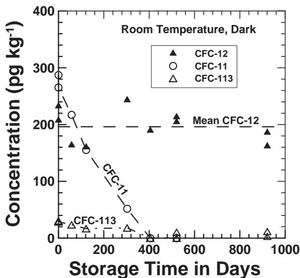
FIG. 12.15. Concentrations of CFC-11, CFC-12 and CFC-113 in sealed ampoules of Withlacoochee River water from south-east Georgia, USA, show degradation of CFC-11 and CFC-113 and apparent stability of CFC-12. Modified from Plummer et al. (1998b).
