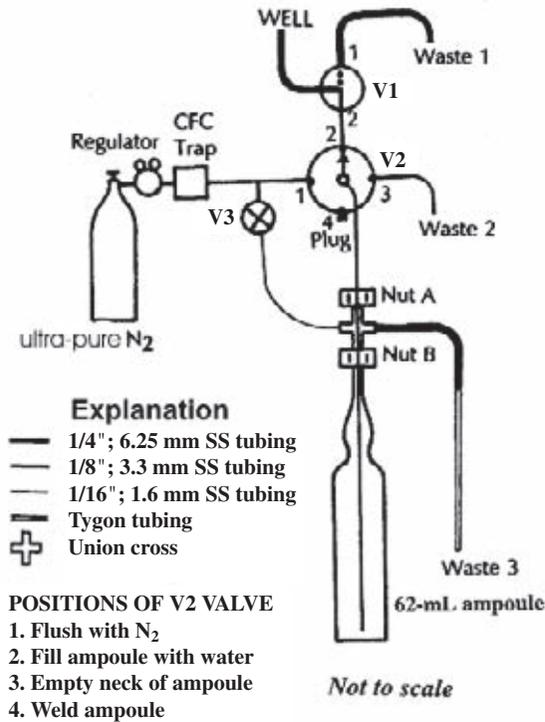
FIG. 12.2. Apparatus to collect groundwater samples without contact with air and flame seal the water in borosilicate ampoules. (See text for details.)
