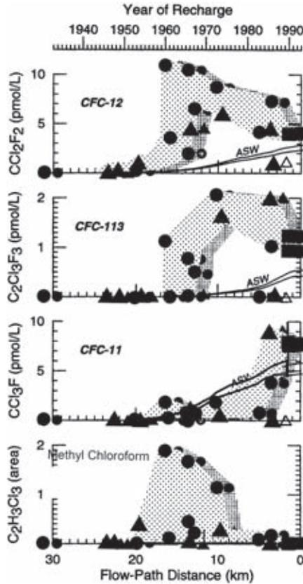
FIG. 9.17. The figure shows concentrations of halocarbons in municipal wells (circles), monitor wells (triangles) and the Danube River (squares). The air saturation with water (ASW) is shown. In reducing waters CFC-11 and CFC-113 was completely or partially degraded. (From Böhlke et al. (1997).)
