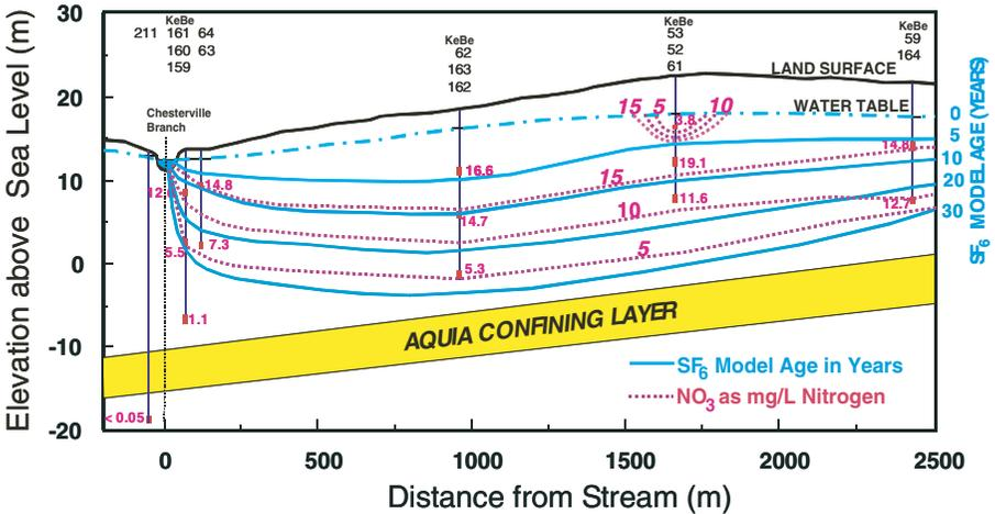
FIG. 9.4. Cross-section of the Locust Grove, Maryland, USA, watershed shows the SF<sub>6</sub> age of the groundwater, as well as the nitrate concentration in the aquifer. Denitrification is occurring in the aquifer in the vicinity of well KeBe 53.
