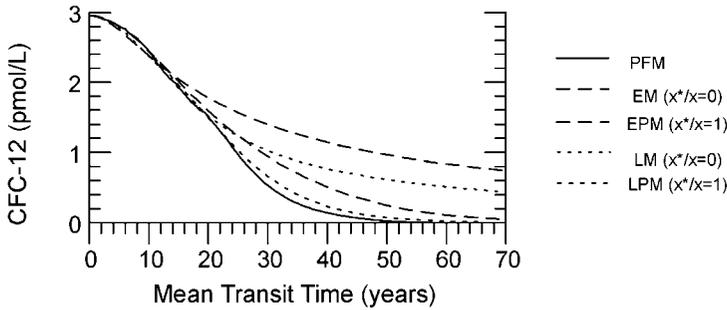
FIG. 6.6. Concentrations of CFC-12 (pmol/L) as a function of the mean transit time (years) for various groundwater discharge models are shown. The vertical axis represents concentrations that would be observed in 1998 in samples of groundwater discharge in which all aquifer flow paths are mixed together, such as might occur at spring. From Cook and Böhlke (2000).
