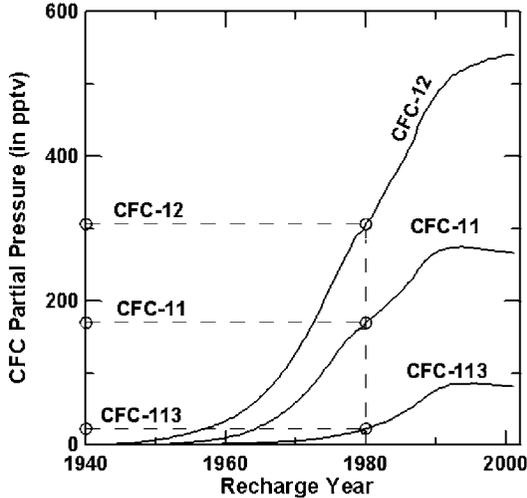
FIG. 3.1. Example showing determination of an apparent recharge date of 1980 from independent analyses of CFC-12, CFC-11 and CFC-113. The curves show historical mixing ratios of CFCs in North American air.
