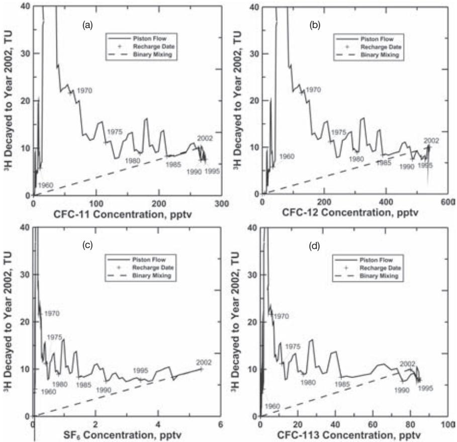
FIG. 5.7. Tracer plots comparing  $^3\text{H}$  in precipitation from Washington, D.C., decayed to the year 2002 with CFC-11, CFC-12, CFC-113 and  $\text{SF}_6$  concentrations in pptv for North American air. The solid lines represent unmixed (piston) flow with selected apparent ages ('+'). The dark dashed lines show one example of binary mixing, for the case of water recharged in 2002 diluted with old, CFC-free water.
