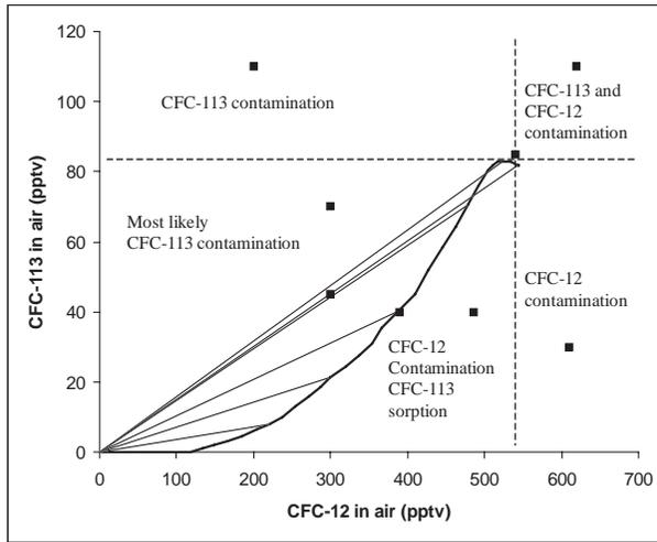
FIG. 8.2. The tracer plot of CFC-113 versus CFC-12 in pptv shows piston flow line, and regions where samples affected by contamination, degradation or excess air would plot. Broken lines denote binary mixing of young and old components (see Chapter 5, Fig. 5.5).
