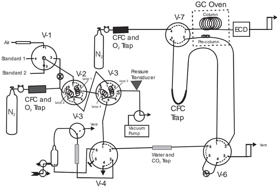
FIG. 12.9. The CFC analytical system used to pre-concentrate and measure CFCs in groundwater and air samples.
