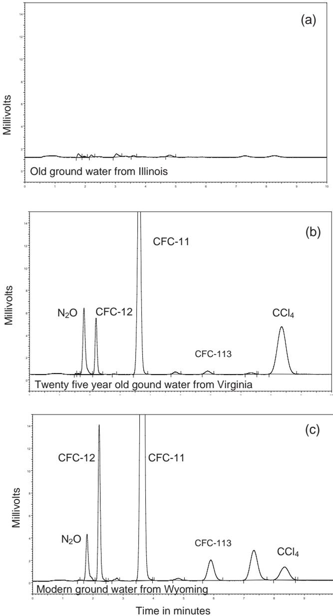
FIG. 12.11. Chromatograms from the U.S. Geological Survey Chlorofluorocarbon Laboratory show: (a) an old, nearly blank sample; (b) a water sample that is approximately 25 year old water from Hudson Spring, Luray, Virginia (sample 3 of Table 8.2); (c) a water sample from Wyoming that is approximately modern (year 2001).
