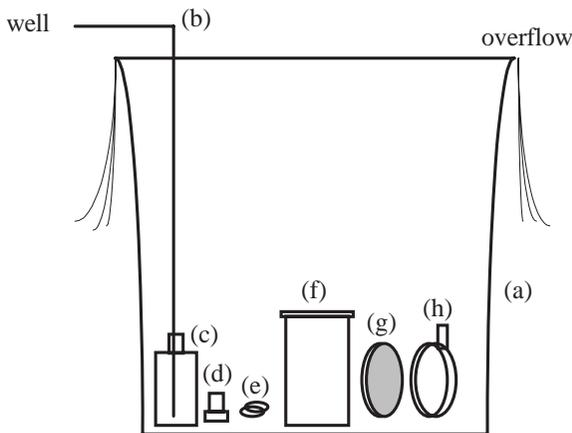
FIG. 12.3. Apparatus for collecting groundwater samples by using large sized 500 mL glass bottles and metal container without contact to air: (a) metal bucket; (b) tubing; (c) narrow neck glass bottle; (d) glass stopper; (e) stainless steel clip (f) metal container; (g) container cover with rubber O-ring sealing; (h) clamp.
