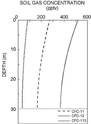
FIG. 4.1. Modelled soil gas concentrations in 1992 above a water table at 30 m depth. Revised from Cook and Solomon (1995) using atmospheric CFC data for the northern hemisphere as reproduced in Appendix II, Table II.1.
