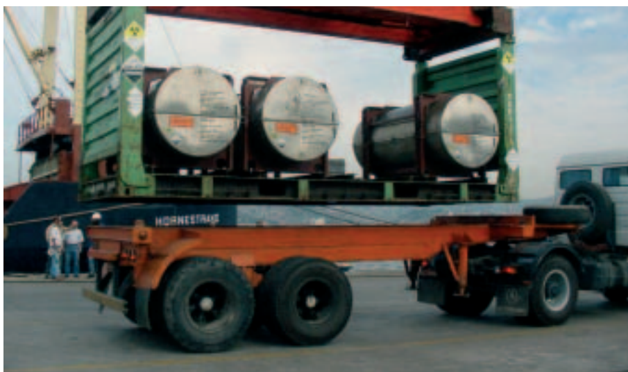
FIG. 5. Closer view of a shipping rack with three cylinders of uranium hexafluoride. The rack is positioned above the flatbed of the first truck in a convoy of several vehicles.
