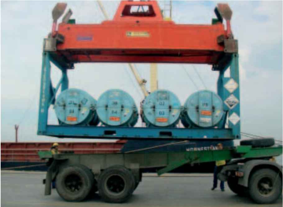
FIG. 6. Closer view of a shipping rack with four cylinders of uranium hexafluoride. The rack is lowered on to the flatbed of the second truck in the convoy.
