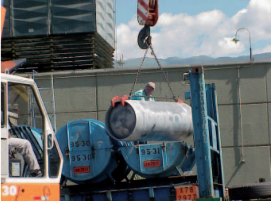
FIG. 10. Reception of uranium hexafluoride at the INB's facilities in Resende, state of Rio de Janeiro: the crane hoisting a cylinder out of its packaging.
