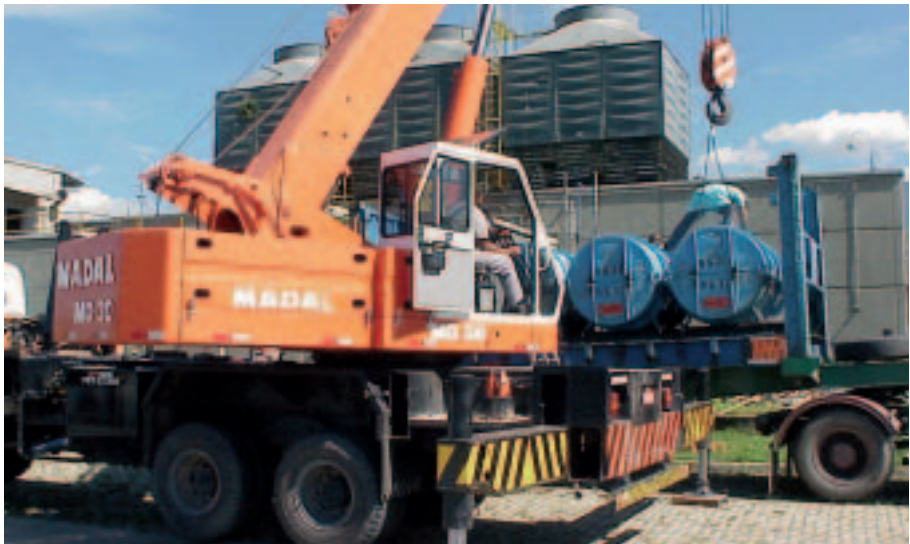
FIG. 9. Reception of uranium hexafluoride at the INB's facilities in Resende, state of Rio de Janeiro: the crane operator and handler position the pulley and hook to lift a uranium hexafluoride cylinder out of its outer packaging.
