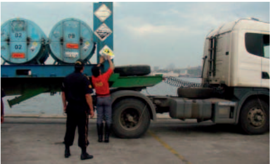
FIG. 7. A technician of the INB applying placards on a truck that carries a load of uranium hexafluoride cylinders.
