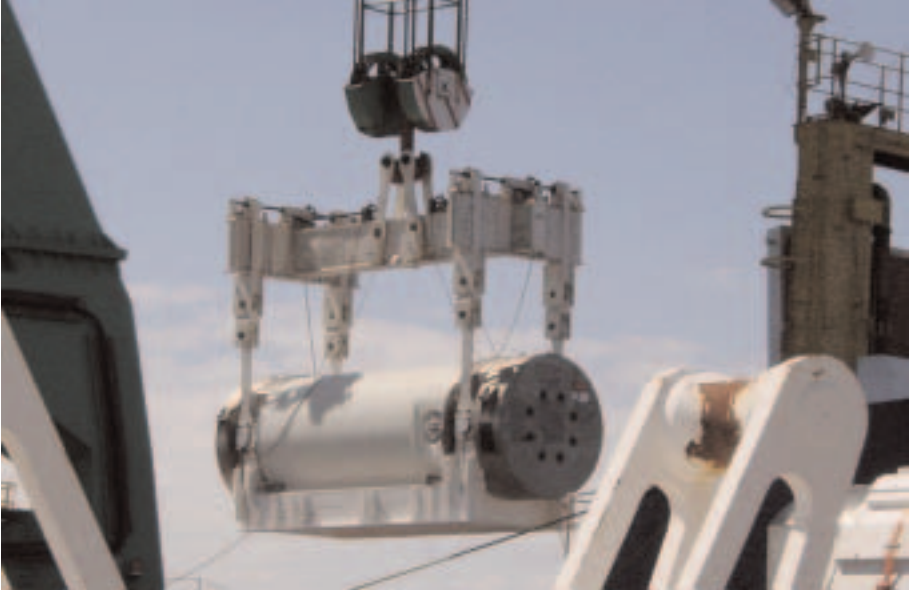
FIG. 12. Flask being transferred by crane from a rail wagon to the ship's hold.
