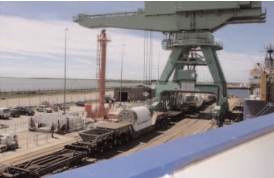
FIG. 9. Flask bearing rail wagons being shunted into location under a crane by DRS locomotives.
