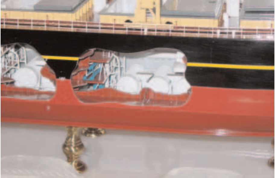
FIG. 6. PNTL ship model showing the location of the holds and double hull.
