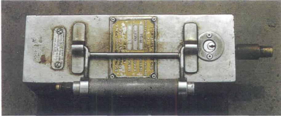
*Photo 3. Radiography camera showing labels and lock.*
