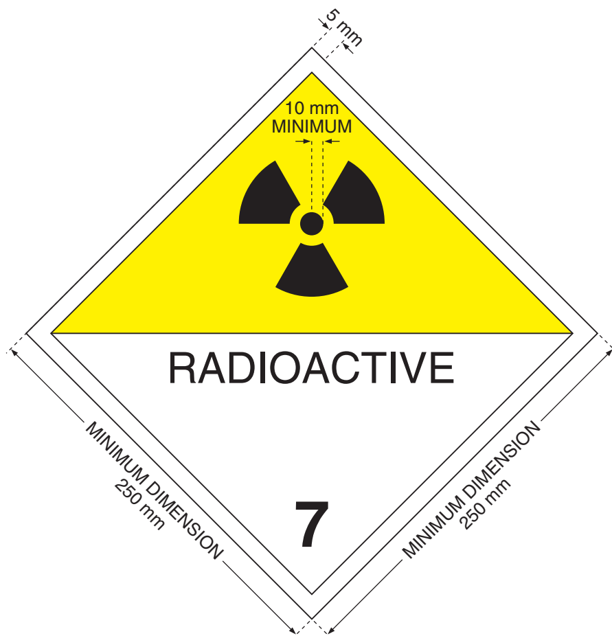
FIG. 6. Placard. Except as permitted by para. 570 minimum dimensions shall be as shown; when different dimensions are used the relative proportions must be maintained. The number '7' shall not be less than 25 mm high. The background colour of the upper half of the placard shall be yellow and of the lower half white, the colour of the trefoil and the printing shall be black. The use of the word "RADIOACTIVE" in the bottom half is optional to allow the alternative use of this placard to display the appropriate United Nations number for the consignment.
