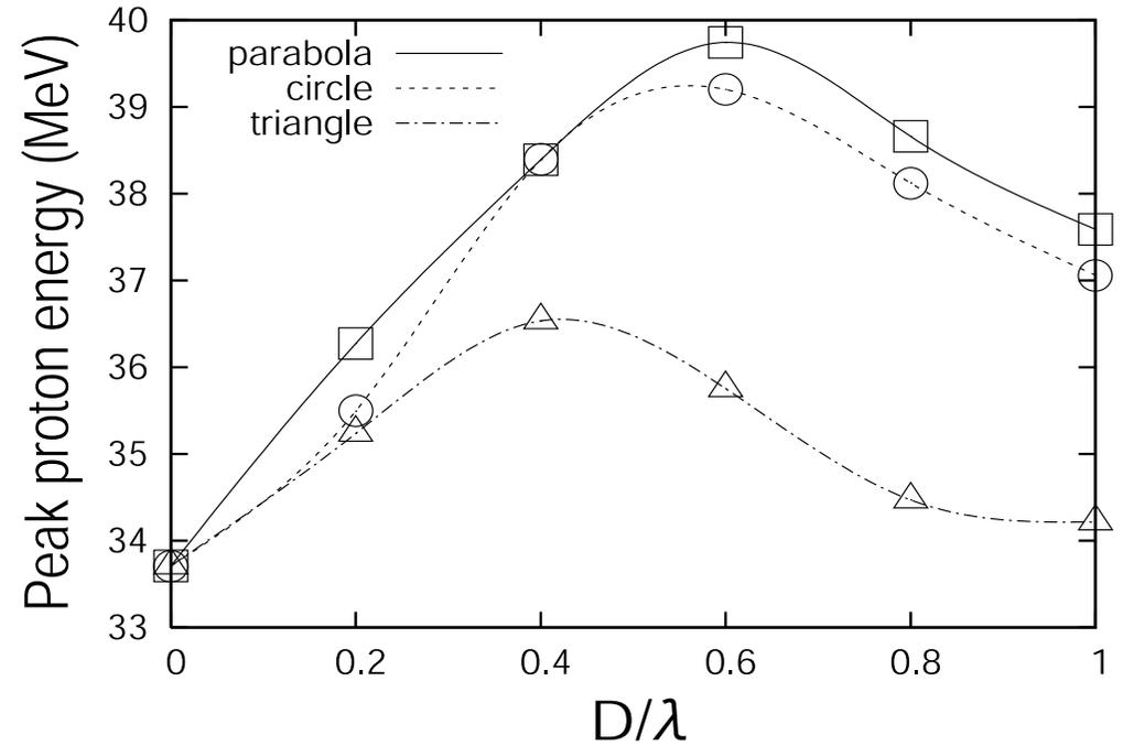
Peak proton energy vs depth of the concave shape ( $D/\lambda$ ) from the triangular, circular and parabolic concave targets at  $\omega t=800$ .
