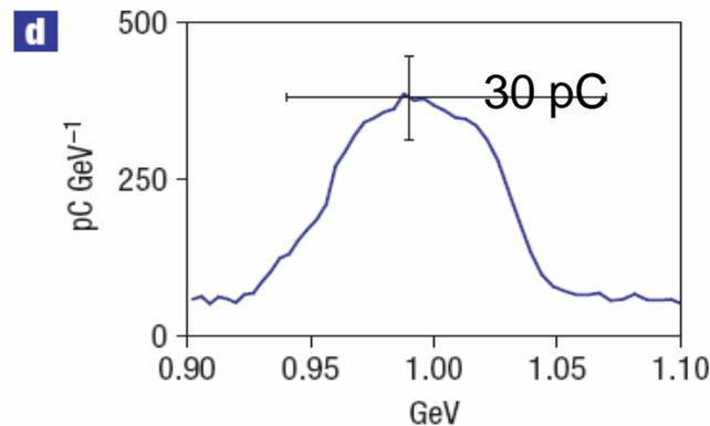
Acceleration to 1 GeV in 33 mm long pre-formed plasma channels
