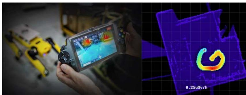
FIG. 24. Example of views of both the source of radiation (left) overlaid onto the spot camera and the dose measurements overlaid onto the building map (right) as real time outputs on the spot controller. (Courtesy of Createc, UK)
