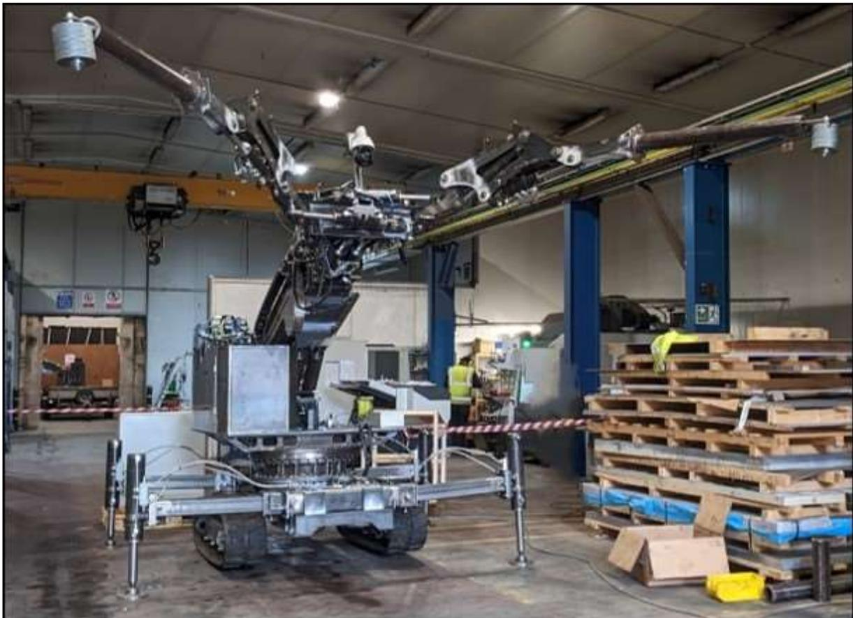
FIG. 19. Current status of Barrnon Integrated Decommissioning System (BIDS) (Courtesy of Sellafield Ltd.)
