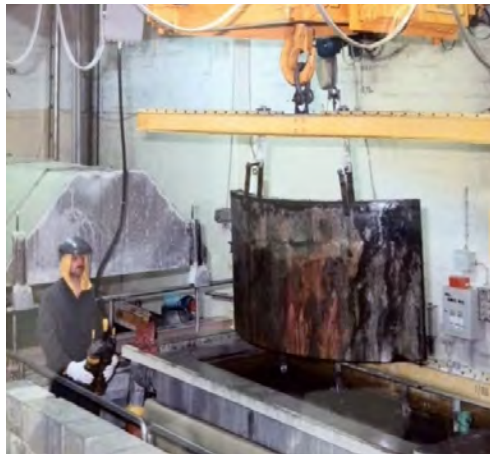
FIG. 6. Electropolishing of a highly contaminated stainless steel piece in the KRB, a boiling water reactor in Grundremmingen, Germany. Courtesy of M. Laraia.
