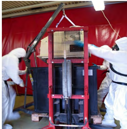
FIG. III-14. Inserting a glovebox used for handling alpha radionuclides (U, Pu, Am, Np) into non-standard disposal units. Courtesy of Nuclear Research Institute Řež, Czech Republic.
