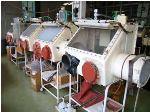
FIG. III-13. Gloveboxes used for handling alpha radionuclides (U, Pu, Am, Np) in ÚJV Řež before decontamination for decommissioning. Courtesy of Nuclear Research Institute Řež, Czech Republic.
