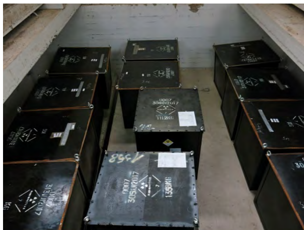
FIG. III–15. Gloveboxes used for handling alpha radionuclides (U, Pu, Am, Np) stored in non-standard disposal units. Courtesy of Nuclear Research Institute Řež, Czech Republic.
