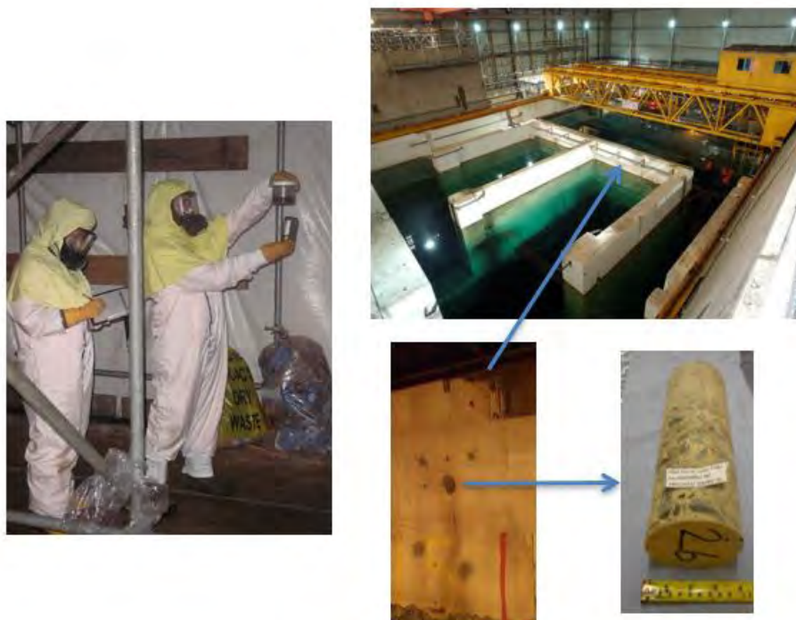
FIG. III-1. Characterization of materials extracted from the cooling pond at Hunterston A power station, United Kingdom, prior to the development of a decontamination strategy. Reproduced with permission from the Hunterston A site, Magnox Ltd, United Kingdom.
