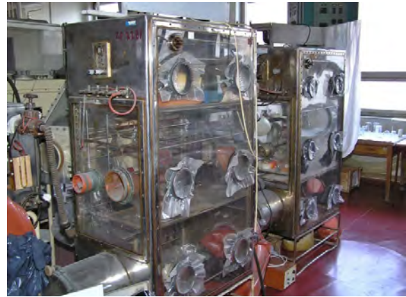
FIG. III-13. Gloveboxes used for handling alpha radionuclides (U, Pu, Am, Np) in ÚJV Řež before decontamination for decommissioning. Courtesy of Nuclear Research Institute Řež, Czech Republic.
