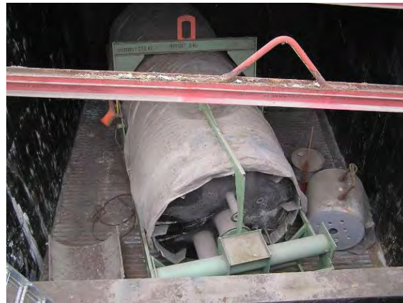
FIG. III-3. Storage of the old VVR-S research reactor vessel. Courtesy of Nuclear Research Institute Řež, Czech Republic.
