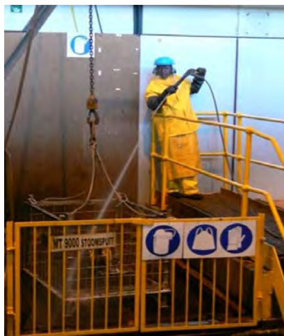
FIG. 5. Example of a chemical decontamination of metals systems. Courtesy of Necsa, South Africa.
