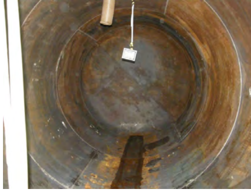
FIG. III-12. Interior of tank B after final decontamination. Courtesy of Nuclear Research Institute Řež, Czech Republic.
