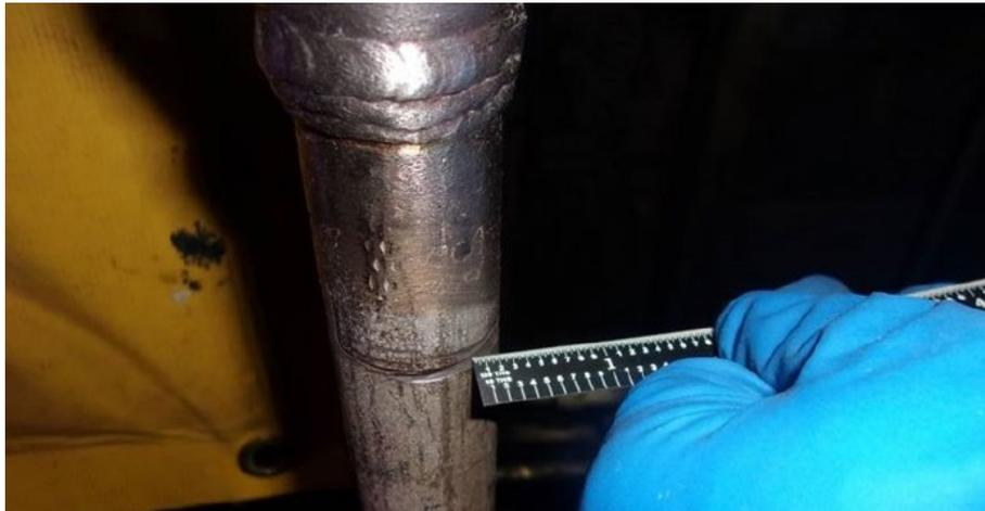
FIG. 12. Pressurizer (PZR) spray line wear caused by flow induced vibration (reproduced from [47]).
