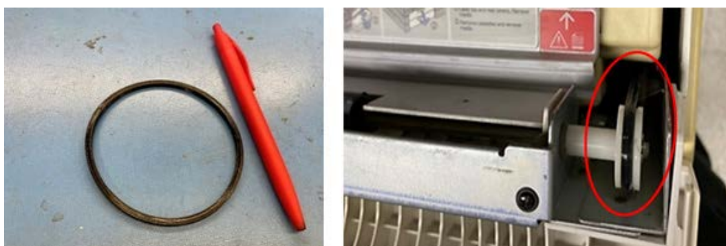
FIG. IV-1. A 3-D printed roller belt by itself and inside the DCC printer.
