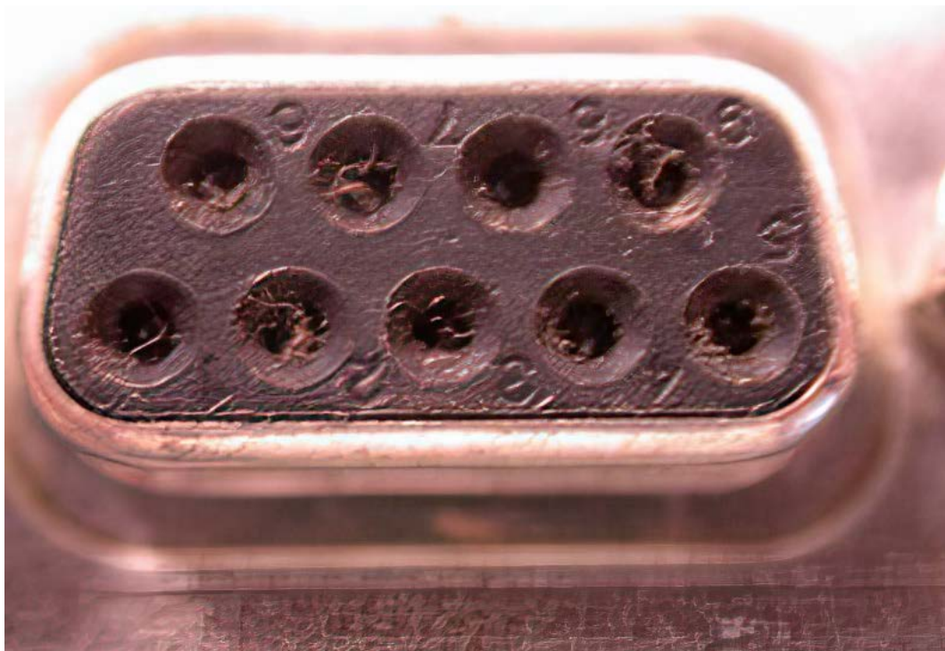
FIG. 8. Connector fluff and dirt contamination.
