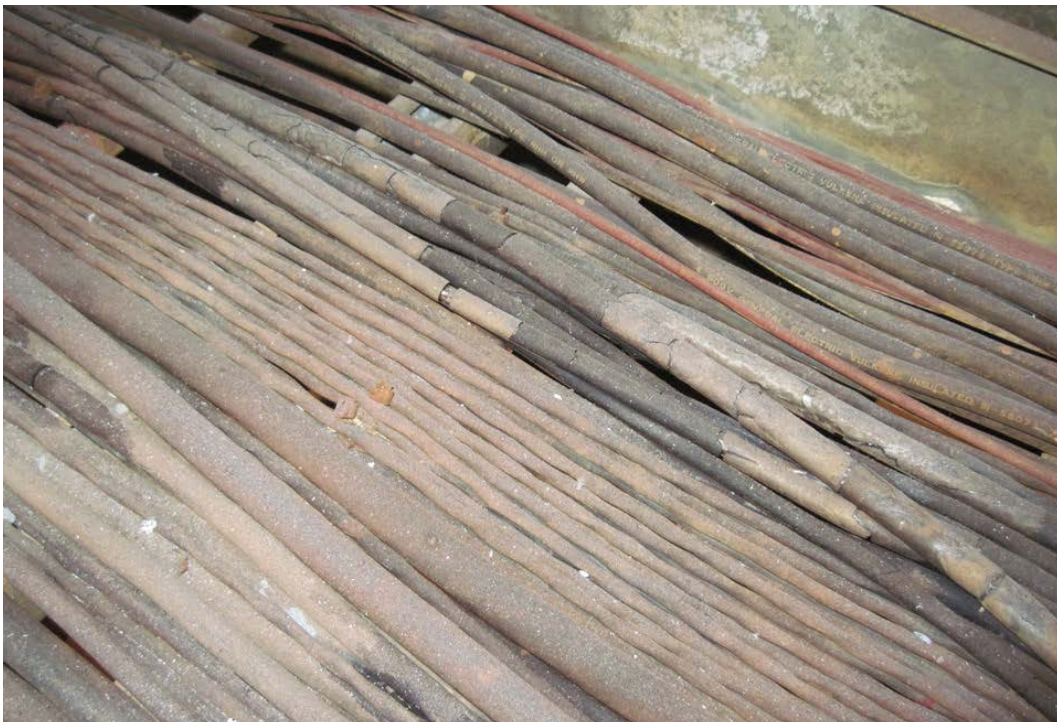
FIG. 17. View of cables degraded from exposure to elevated temperatures.
