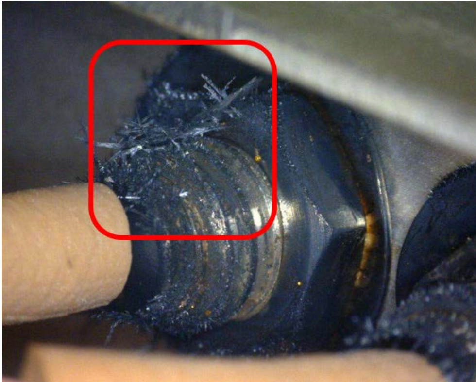
FIG. 3. Silver 'whiskers' growing from a silver plated feedthrough capacitor.
