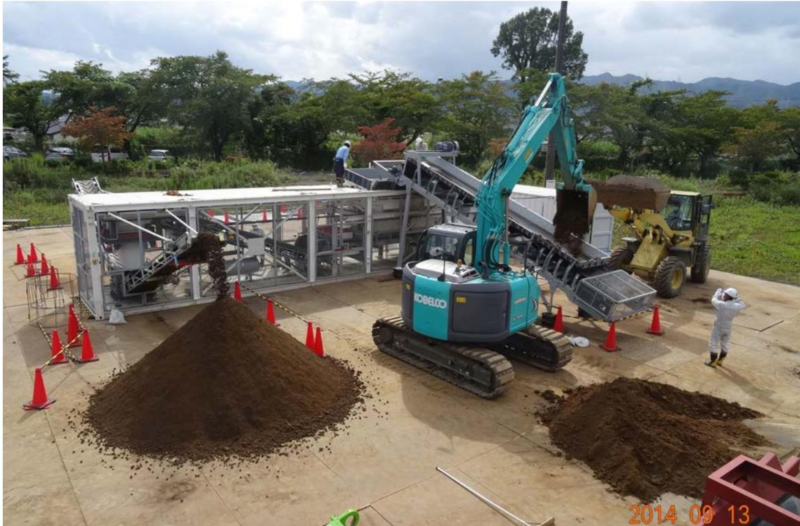
FIG. 27. Contaminated soil sorting unit used at Fukushima Daiichi NPP. Courtesy of GRS VALTECH.
