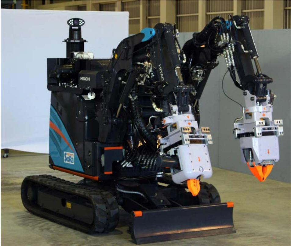
FIG. 21. Remote control robot (ASTACO-SoRa) used to remove rubble and debris in the reactor buildings, significantly reducing the dose to workers. Courtesy of Tokyo Electric Power Company Holdings.
