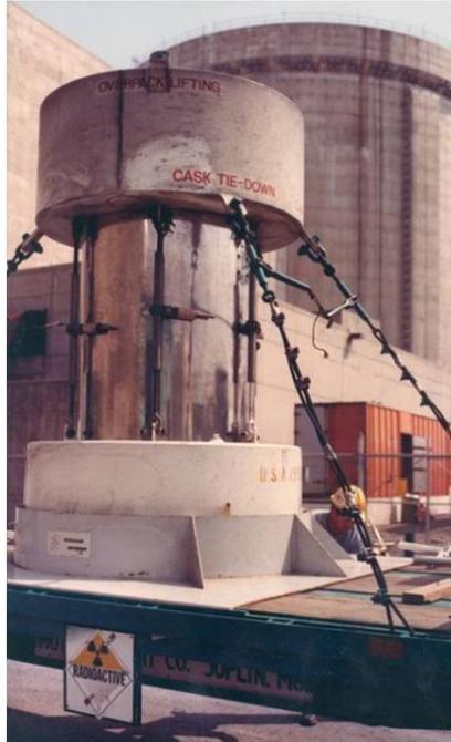
FIG. 43. The CNS 1-13C cask readied for shipment at TMI. Courtesy of Idaho National Laboratory and the US Nuclear Regulatory Commission [152].
