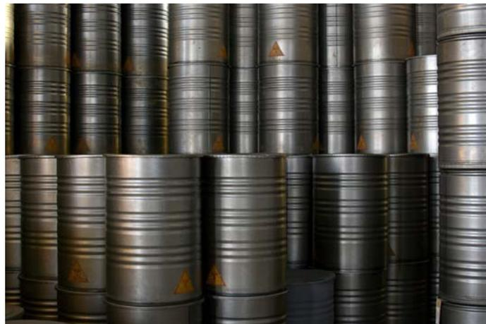
FIG. 41. MB-0.2IV drum used at Chornobyl. Courtesy of State Specialized Enterprise Chornobyl NPP.
