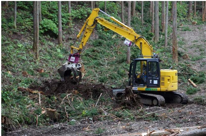
*FIG. 19. Unmanned remote-controlled construction machines used to clear vegetation in off-site areas of the Fukushima region. Courtesy of Kajima Corporation.*
