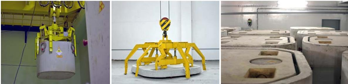
FIG. 40. KZ-3.0 concrete container used at Chornobyl: lifting and translation configuration (top); transportation lid (middle); storage (bottom). Courtesy of State Specialized Enterprise Chornobyl NPP.
