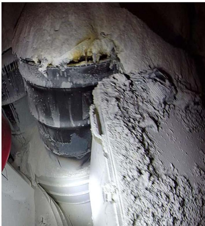
*FIG. 44. Ruptured drum located in Panel 7, Room 7 of the WIPP geological repository. Courtesy of the US Department of Energy [164].*
