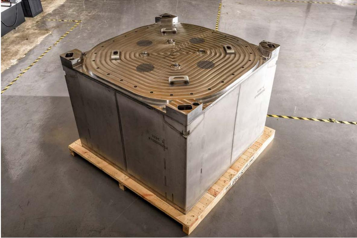
*FIG. 56. The 3 m<sup>3</sup> box for Pile 1 graphite and other reactor wastes that will eventually be disposed of in the national GDF. Courtesy of the Nuclear Decommissioning Authority.*
