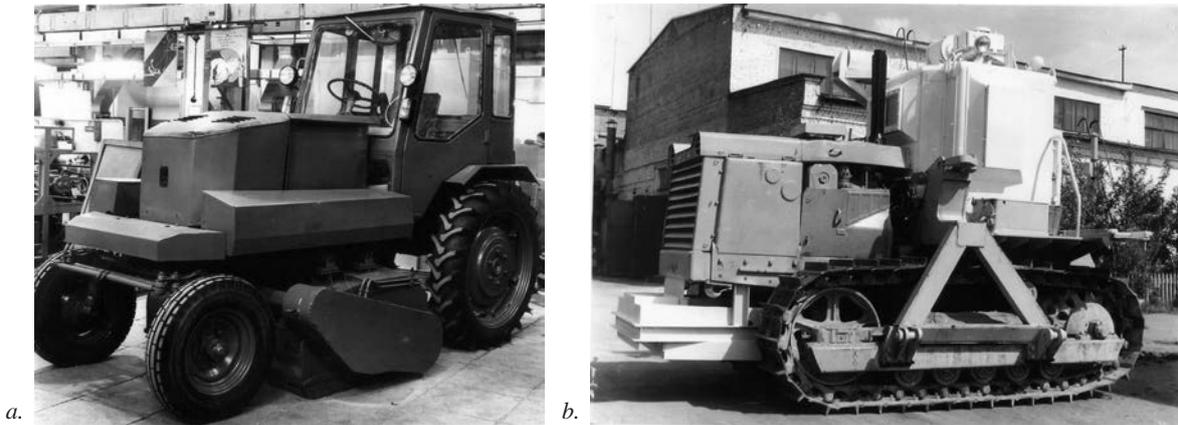
FIG. 16. Modified tractors used in the Chernobyl response. (a) MTZ-80 tractor used for street cleaning to collect radioactive dust and refuse. (b) Heavily shielded modified Cheyabinsk tractor used in cleaning areas adjacent to the damaged Unit 4 reactor and for transportation of supplies. Courtesy of the Ukrainian National Chernobyl Museum.
