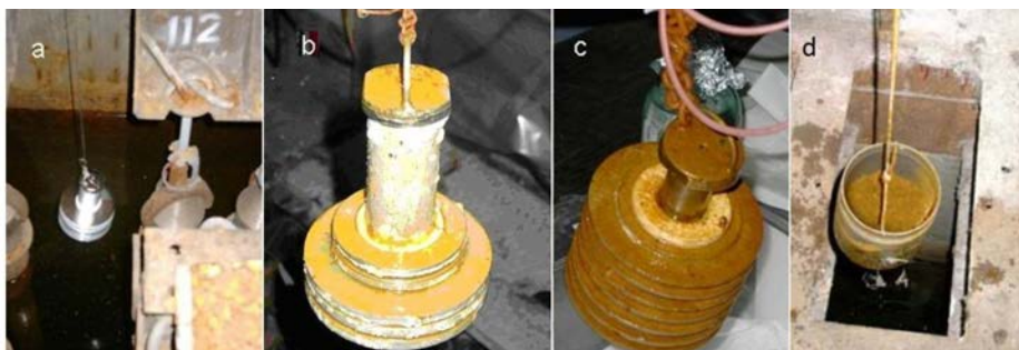
FIG. 33. (a) CRP test rack being immersed in the storage pool water then (b) removed after 24 months, and (c) removed after 72 months, as well as a (d) sediment collector [7].
