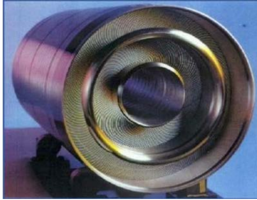
FIG. 15. The HFIR fuel element (courtesy of the Savannah River National Laboratory, USDOE).
