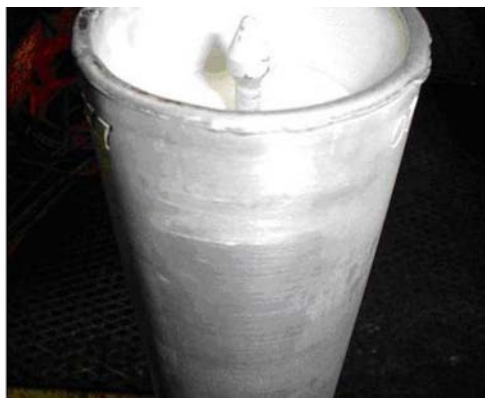
FIG. 30. Canning tube secured by welding (courtesy of BRR [123]).
