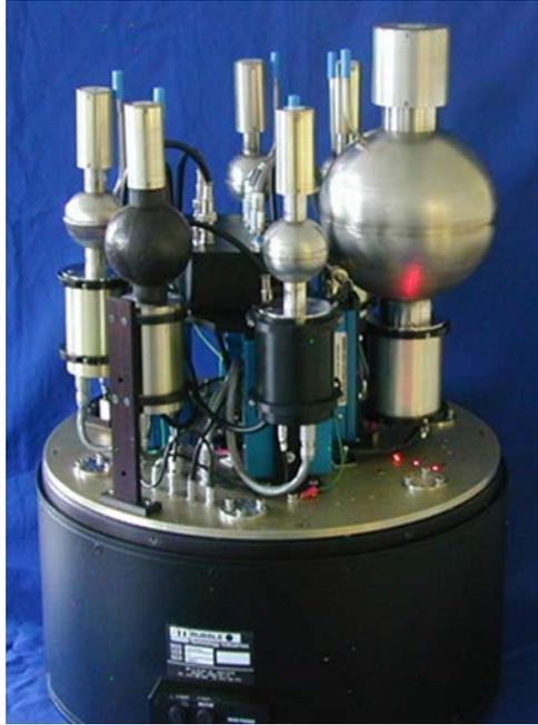
FIG. 9.9. The ROSPEC neutron spectrometer. (Picture supplied by Bubble Technology Industries.)
