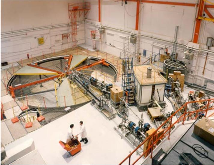
*FIG. 14.2. Low scatter environment for neutron calibrations. Monoenergetic neutrons are produced at the centre of the circle seen at left in the picture at about 6 m from the nearest solid surface (the floor). (Courtesy of National Physical Laboratory.)*
