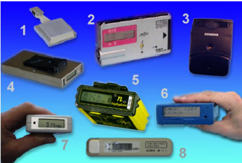
FIG. 11.8. Examples of electronic neutron dosimeters. 1: RADOS DIS-N; 2: FUJI Electric NRNO; 3: Siemens EPD-N and EPD-N2; 4: GSF; 5: SAPHYDOSE-N; 6: University of Munich AMIRA; 7: PTB DOS-2002; 8: ALOKA PDM-313. (Reproduced from Ref. [11.23] with permission from Oxford University Press.)
