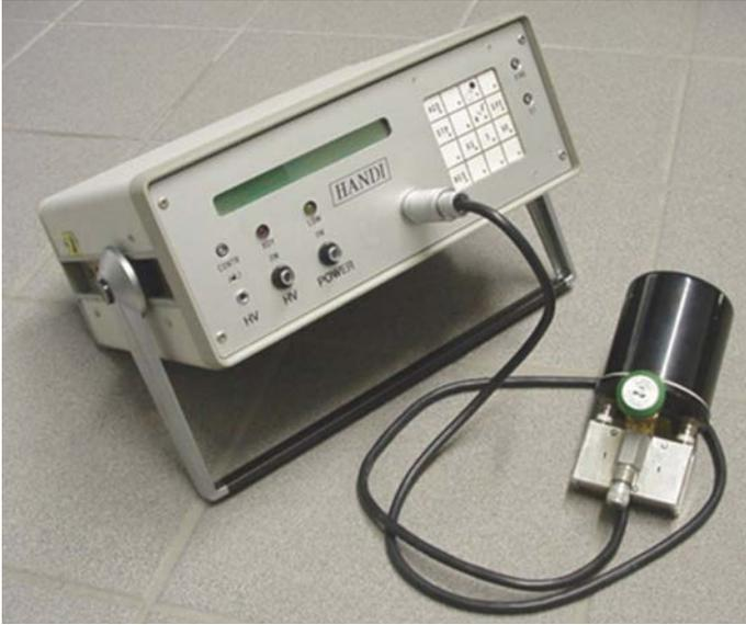
FIG. 10.5. The HANDI TEPC, produced by the University of Saarland. (Photo kindly provided by H. Schuhmacher; PTB.)
