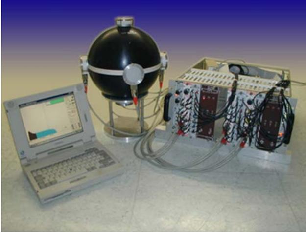
FIG. 13.3. Directional spectrometer as used within the EVIDOS project. (Reproduced from Ref. [13.17] with permission from Oxford University Press.)
