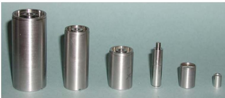
FIG. 7.1. Typical radionuclide source capsules: from left to right, X14 (60 mm long by 30 mm diameter), X4, X3, X224, X2 and X1 (10 mm long by 7.8 mm diameter). The small capsules are used for  $^{252}\text{Cf}$  sources and the larger ones for  $^{241}\text{Am}(\alpha, n)$  sources. (Courtesy of National Physical Laboratory.)
