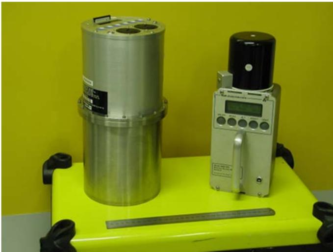
FIG. 10.6. Two commercially available instruments based on TEPCs: the Hawk on the left and the REM500 on the right. (Courtesy of National Physical Laboratory.)
