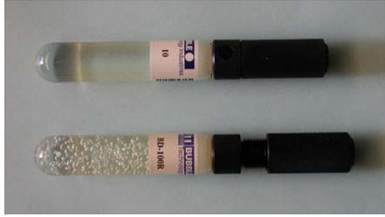
FIG. 8.3. Two bubble detectors: the bottom one shows a large number of bubbles following irradiation, and the top one is unirradiated. (Courtesy of National Physical Laboratory (NPL).)
