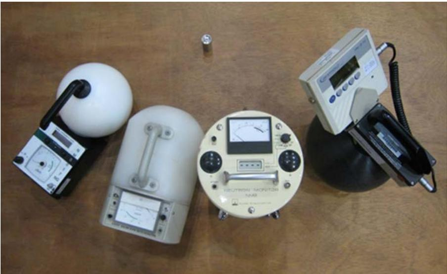
FIG. 10.1. Several commonly used area survey instruments: from the left, a Leake type monitor, a Studsvik/Alnor 2202 D, an NM2 monitor and a Berthold LB6411. (Courtesy of National Physical Laboratory.)
