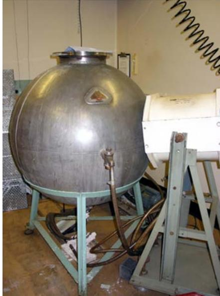
*FIG. 7.5. A manganese sulphate bath. For this model, sources are positioned on the end of a rod and are inserted into the bath from the top. A long counter, to the right in the picture, measures neutron leakage from the surface of the bath. (Courtesy of National Physical Laboratory.)*
