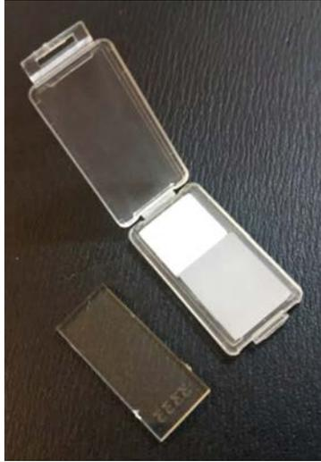
FIG. 11.1. A commercially available etched track dosimeter containing both a hydrogenous and a boron loaded converter layer. These can be seen inside the dosimeter case on the right. The etched track plastic material is on the left. (Courtesy of Chiyoda Technol.)
