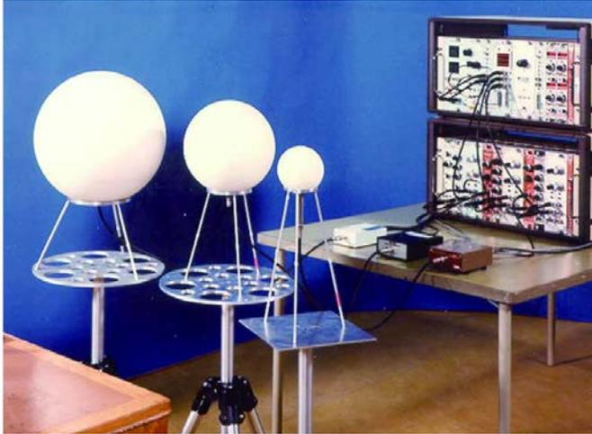
FIG. 9.1. Three Bonner spheres from a set that utilizes a spherical  $SP9$   $^3\text{He}$  proportional counter as the central sensor, shown with their associated electronics. (Courtesy of National Physical Laboratory.)
