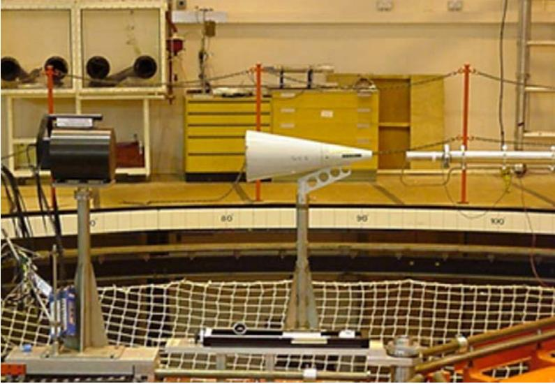
FIG. 14.3. A shadow cone being used with neutrons from an accelerator target. (Courtesy of National Physical Laboratory.)
