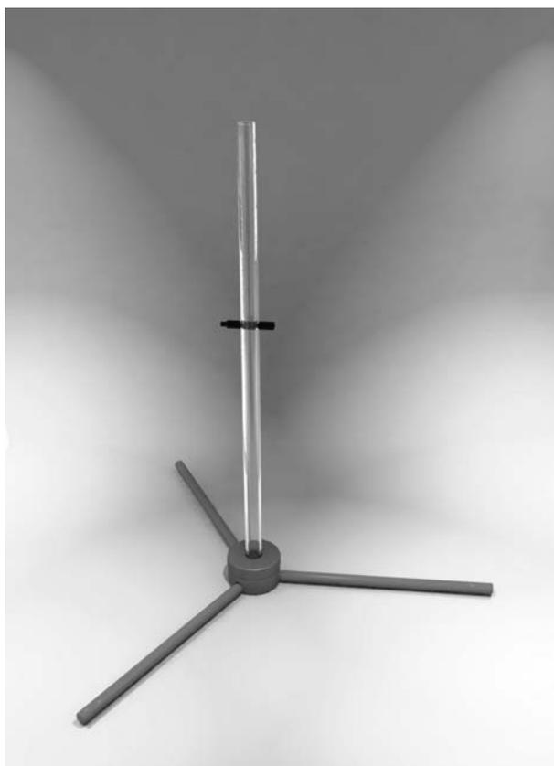
FIG. 2. Standard TLD holder for dosimetry audits of photon beams (reproduced from Ref. [106]).
