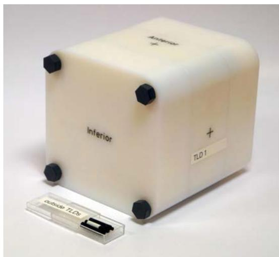
FIG. 63. Phantom containing IMRT QA insert loaded with film and TLDs, and a pillbox with TLDs to be affixed to the outside of the phantom.
