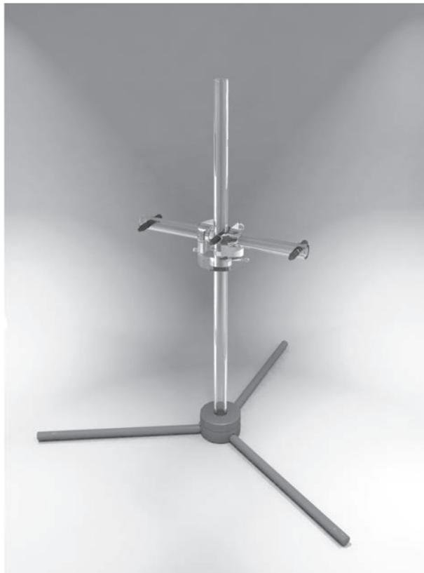
FIG. 9. Modified standard TLD holder for off-axis measurements with photon beams (reproduced from Ref. [106]).
