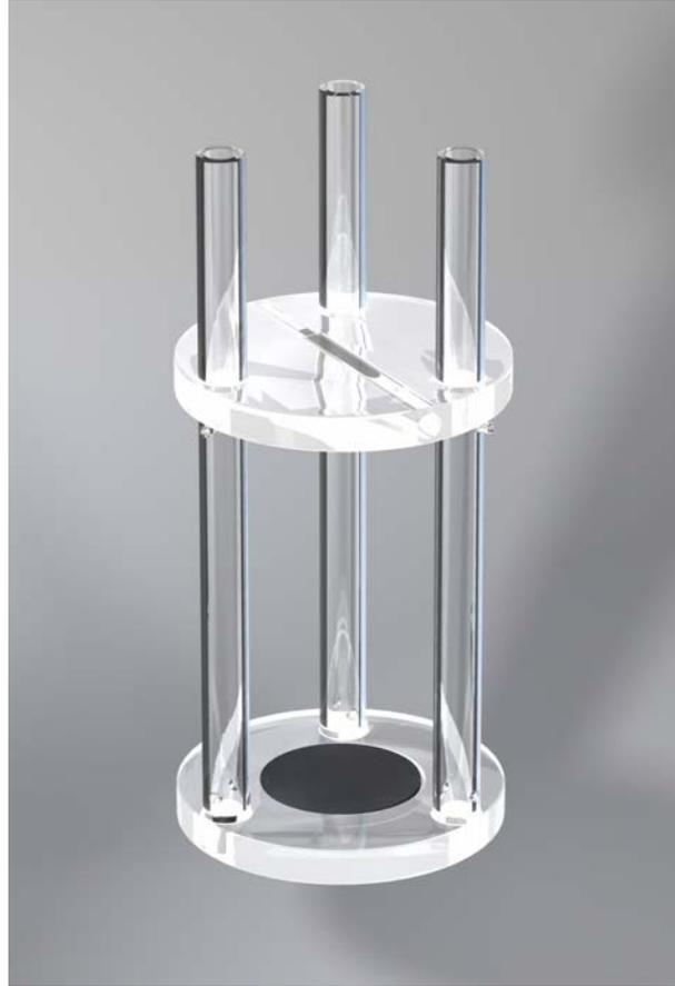
*FIG. 7. Standard TLD holder for electron beams.*
